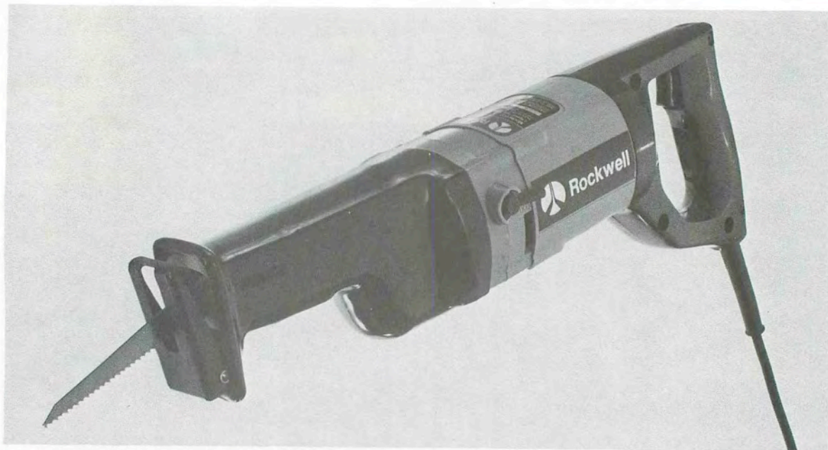
Fig. 15-19. Reciprocating saw with short blade (courtesy Rockwell International).
