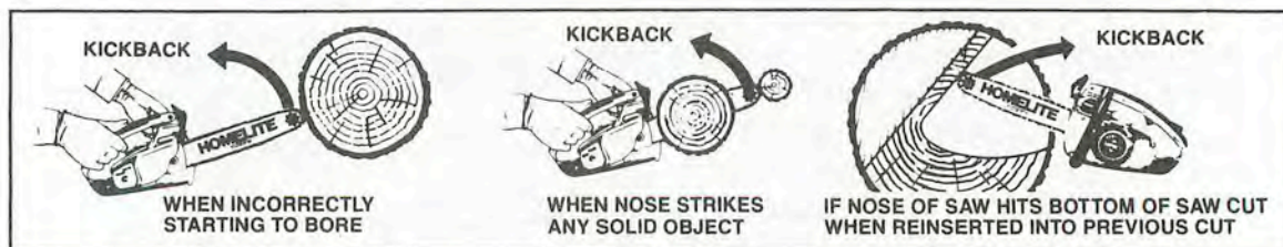
Fig. 24-9. Situations known to cause kickback toward the operator (courtesy Homelite).
