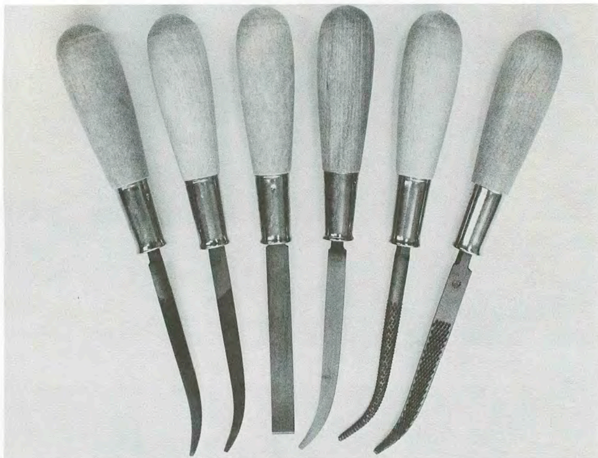
Fig. 12-14. Nicholson's riffler wood rasps and files (courtesy Cooper Tool Group).
