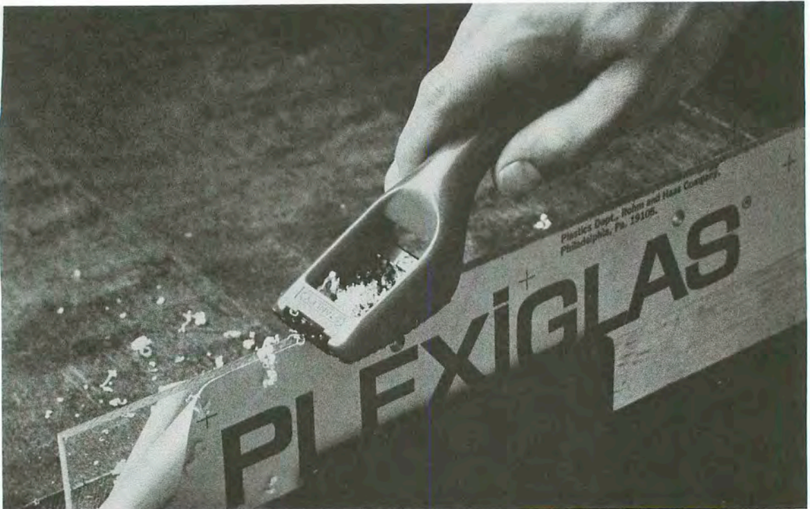
Fig. 12-4. Surform in use on plastic (courtesy Stanley Tools).
