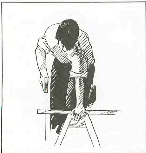
Fig. 3-12. Sawing a board to size.
