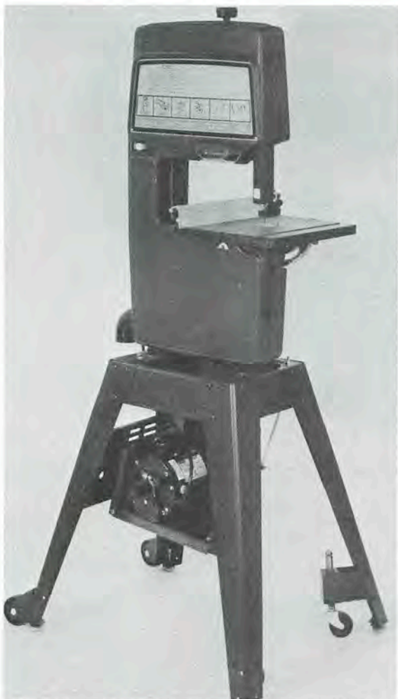
Fig. 23-2. A Craftsman 12-inch band saw (courtesy Sears, Roebuck and Co.).
