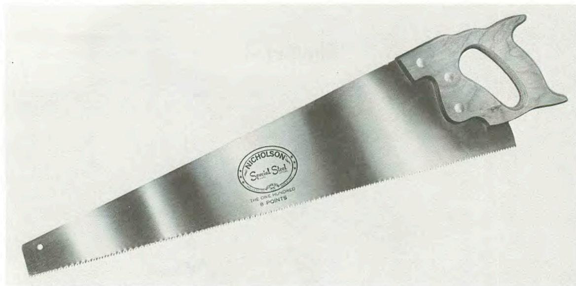
Fig. 3-1. An 8-point handsaw (courtesy Nicholson).
