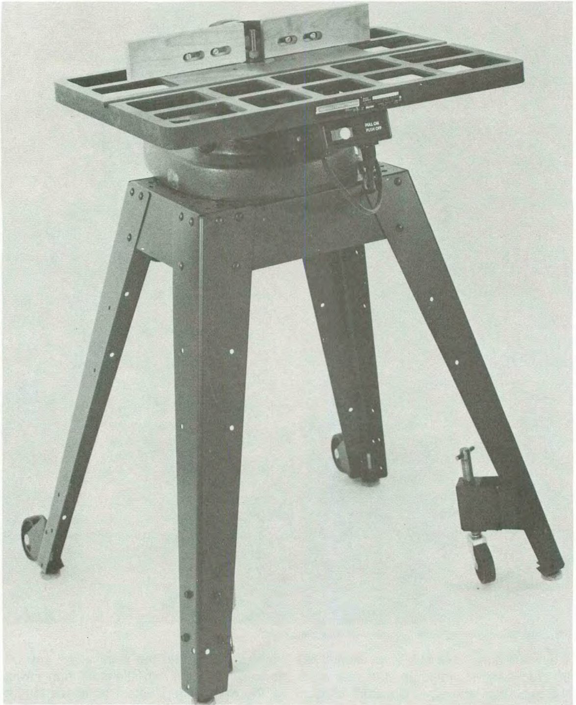
Fig. 23-27. A table shaper with an open-grid table allows chips to fall with less worry about waste buildup (courtesy Sears, Roebuck and Co.).
