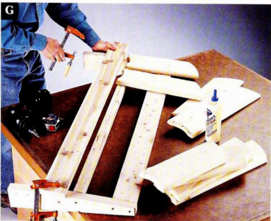
G Clamp a straight board to the back frame to help keep the back slats aligned along their bottom edges as you install them.
