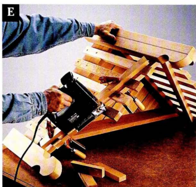
E Use a cutting guide to trim the tops of the slats so they extend beyond the tops of the stringers.
