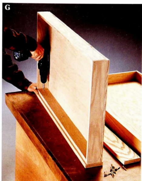
Attach drawer faces with glue, and drive wood screws through the inside of the drawer box into the drawer face.
