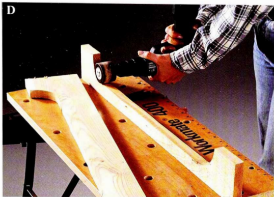
Smooth the jig saw cuts on the radius cutouts using a drum sander attachment and drill.
