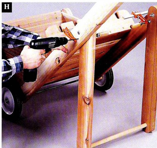
Drill \frac{1}{8} "-dia. holes through the back supports and into the arms for inserting the hitch pins that lock the arms in position.
