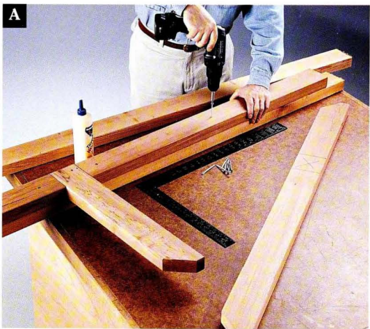
Butt an end of the upper section against the top edge of the mailbox arm, and fasten it to the side.
