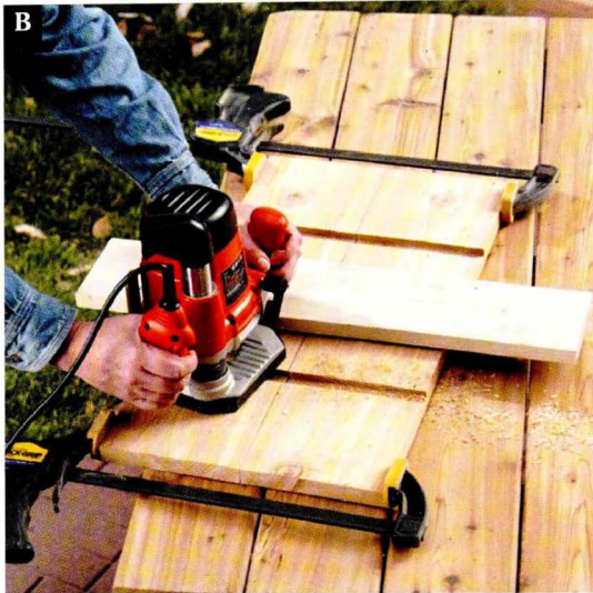
Cut dado grooves in the side panels for the removable divider walls.
