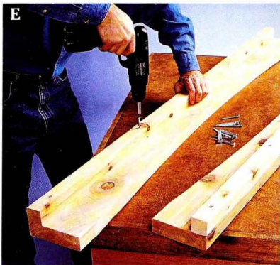
Attach a 2 \times 2 slat to the top, inside edge of each apron, using 2\frac{1}{2} " deck screws and glue.
