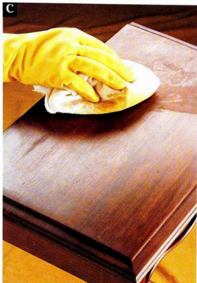
Begin buffing the wax with a soft cloth, using a light, circular motion. Buff the entire surface until the filminess disappears and the wax is clear.
