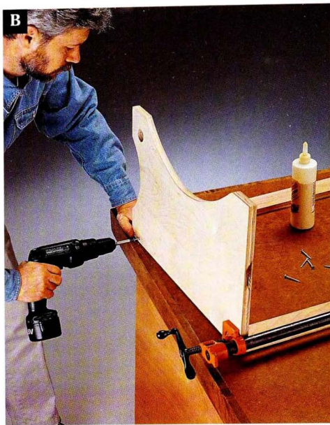
B Apply glue and drive screws through the ends and into the stretchers. Use pipe clamps to ensure square joints.
