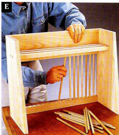
E Insert dowels into the holes under the back first, then drop them down into the holes in the rail.
