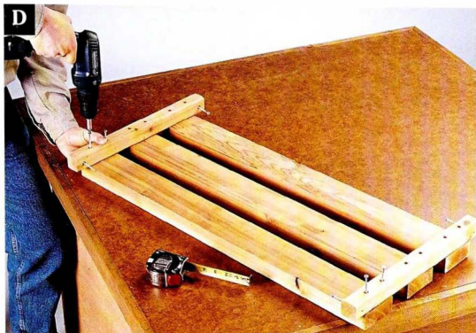
Fasten the bottom cleats to the shelf slats, keeping the ends of the slats flush with the outside edges of the cleats.
