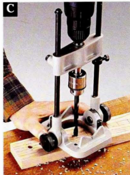
A portable drill stand helps you drill straight or angled holes.
