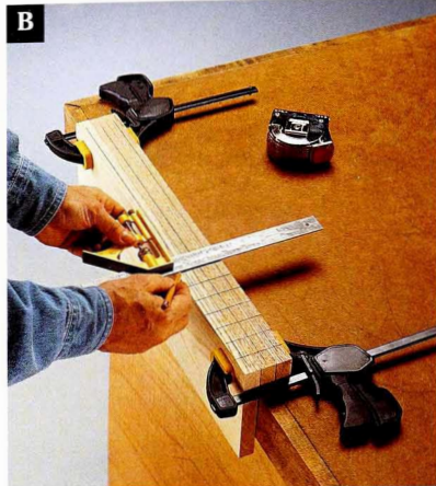
Clamp the rails and back together and mark the dowel holes.
