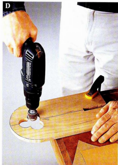
Use a drum sander or sandpaper wrapped around a dowel to smooth the inside of the cutout.
