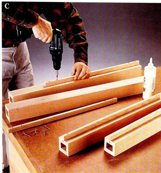
Attach the end half slats to the legs with glue and wood screws.
