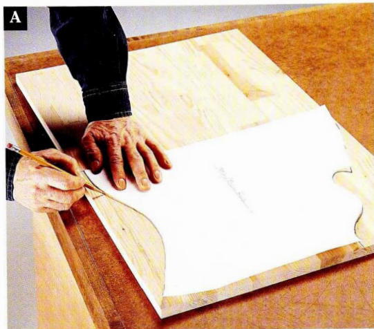
Lay out the pattern on the back piece by tracing half the pattern on one side of the centerline, then flipping the pattern and tracing the other side.
