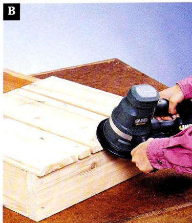
Round the slat edges with a router or a power sander.
