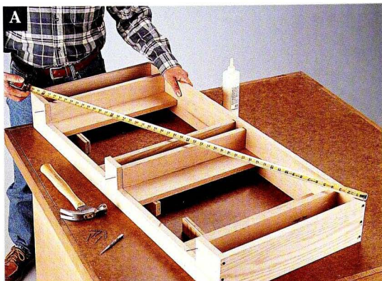
A Measure the diagonals and adjust the apron frame as needed until it is square.
