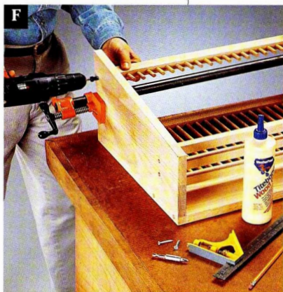
F Clamp the front rail, predrill the sides, counterbore, glue and screw in place.
