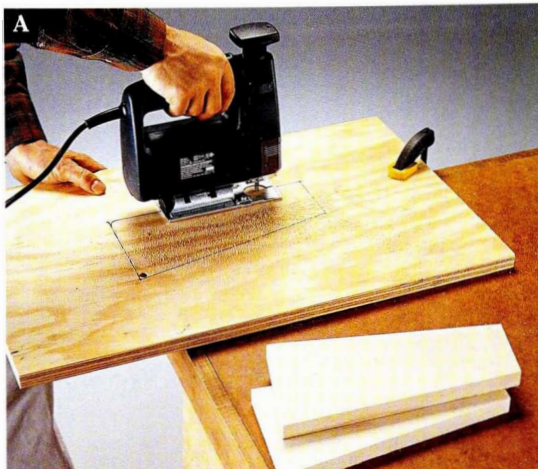
To make the jig, trace an outline of a side on a piece of plywood and cut with a jig saw.
