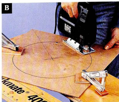
Cut out the router template using a jig saw.
