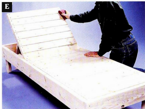
Sand all surfaces carefully to eliminate splinters, and check to make sure all screw heads are set below the wood surface.
