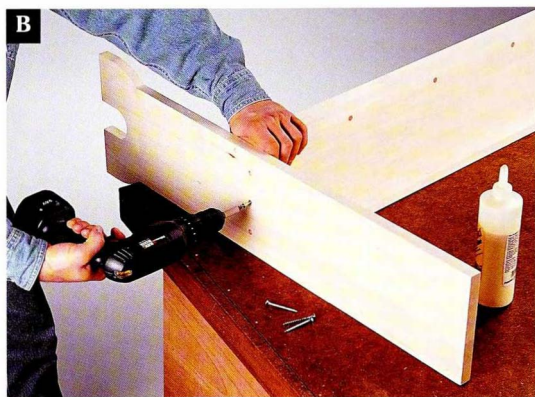
Attach the shelf by driving wood screws through counterbored pilot holes in the legs.
