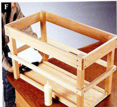
F Fasten the bottom shelf by driving wood screws through the bottom rails and into the legs.
