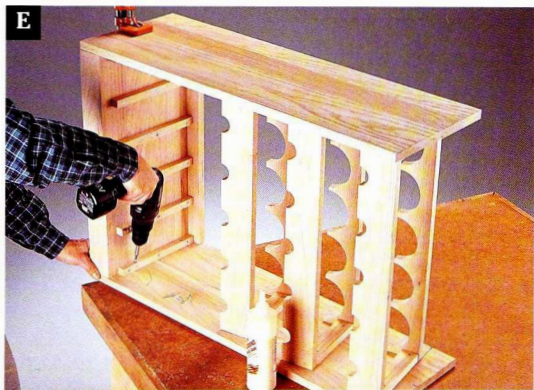
E Drive screws through the slats to secure the top to the sides.
