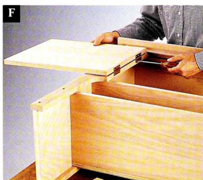
Attach each door to a leg, using 1 1/2 x 3" butt hinges.
