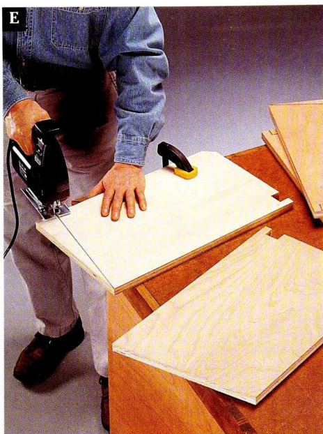
E Clamp the bin sides to your work surface, and use a jig saw to cut the notches and bevels.
