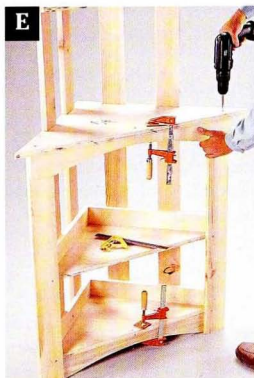
Drive screws through the center shelf and into the face frame.
