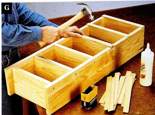
G Using glue and 4d finish nails, attach the swing-out shelf sides.
