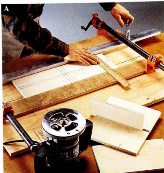
To cut the shelf dados, rout both sides in one pass, using a clamped straightedge as a guide for the router base.
