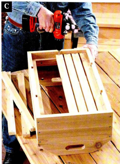
Attach the floor slats to the support cleats with galvanized screws.
