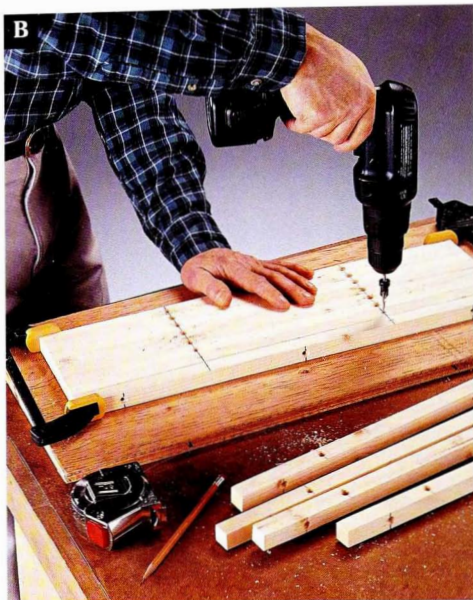
B Gang the cleats together while drilling countersunk pilot holes.
