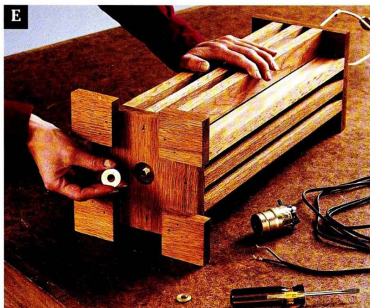
Install the threaded lamp rod, and secure it to the bottom plate with a washer and nut.
