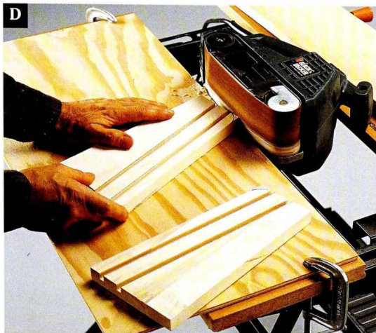
Round the edges on the sides and base with a belt sander.
