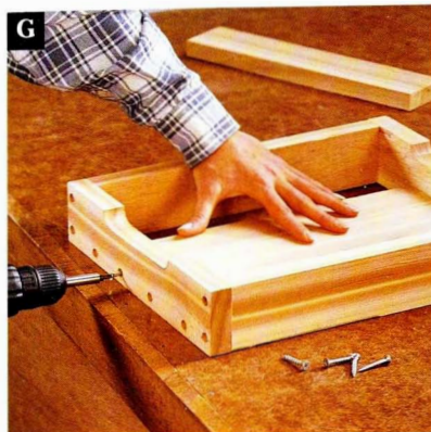
Attach the tray bottoms to the tray ends and sides with glue and screws.
