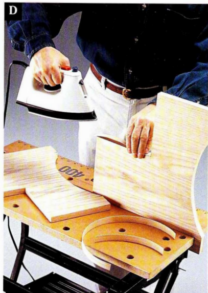
Apply veneer tape to the front and back edges of the sidepieces to give them a solid wood appearance.
