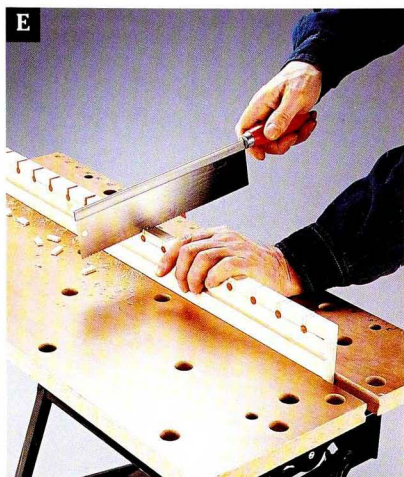
Cut a \frac{1}{8} "-wide notch along the front edge for each of the spoon rack holes, using a backsaw.
