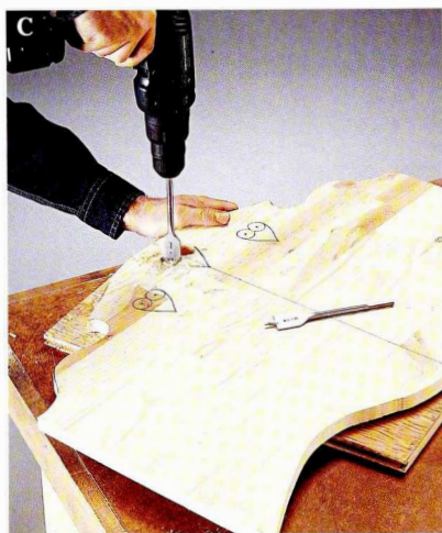
Drill out the larger heart using a 1" spade bit. Use a \frac{5}{8} " spade bit to create the smaller hearts. Complete the cutouts with a jig saw.
