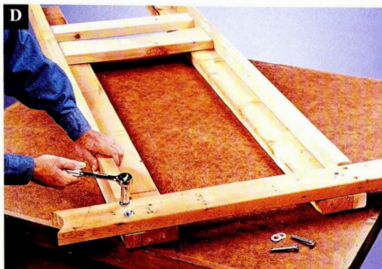
Lag-screw the cross beams to the legs, and fasten the spreaders and rails with deck screws to assemble the side frames.
