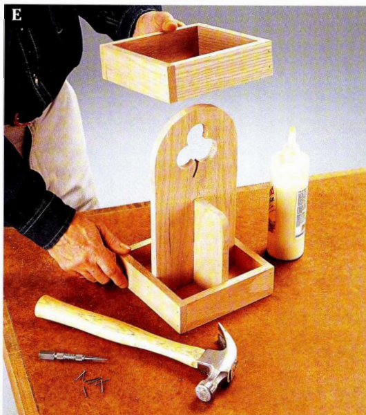
Maintain a 1/4 " gap between frames when assembling.
