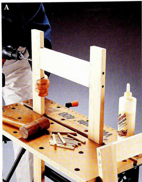
A Drill holes and insert the dowels after the frame pieces have been glued together.
