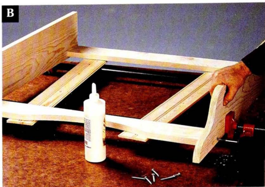
Clamp the sides and ledgers in position, then fasten with glue and screws.
