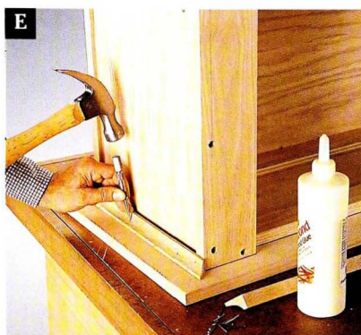
Miter-cut cove molding to cover the joint between the top panel and the carcass.
