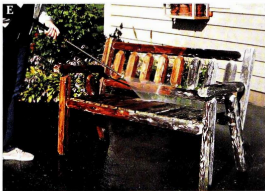
E A pressure washer can be used to clean and brighten unfinished outdoor projects, or to strip and clean finished surfaces for refinishing. Remember that high water pressure can destroy the soft wood fibers of cedar and redwood.
