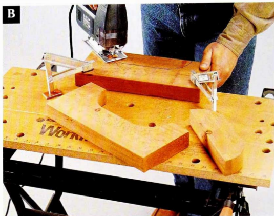
Use a jig saw to make scalloped cutouts in all four base pieces—make sure the cutouts in matching pieces are the same.
