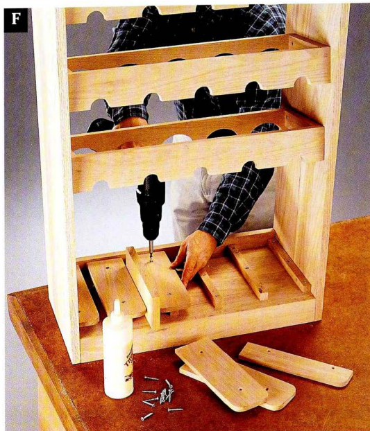
Use a \frac{1}{4} "-thick spacer to guide the placement of the stemware plates.
