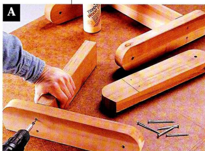
Fasten the stretchers between the legs with glue and deck screws.
