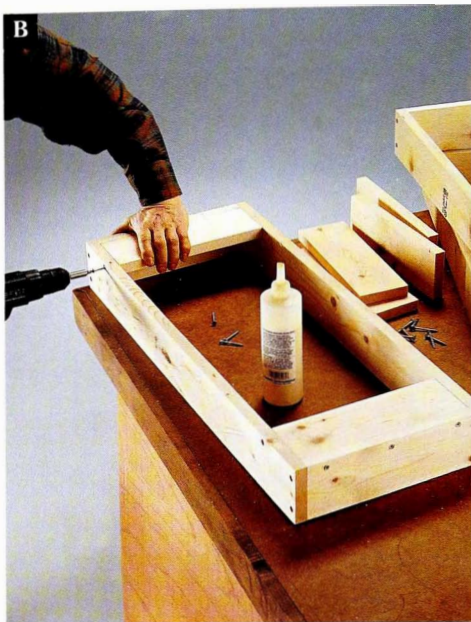
Apply glue and drive counterbored screws into the shelf faces and shelf ends to connect the stretchers.
