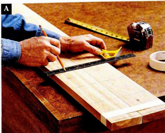
Tape the legs together with their edges flush, and gang-mark the stretcher positions on the inside faces.
