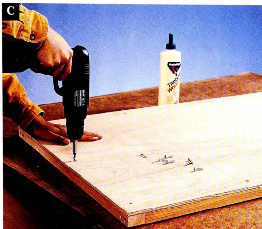
Attach the end panel to the open-ended frame assembly, making sure that the rough side of the cedar siding is facing outward.
