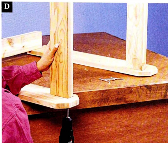
Attach the square ends of the posts to the undersides of the arms, being careful to position the part correctly.
