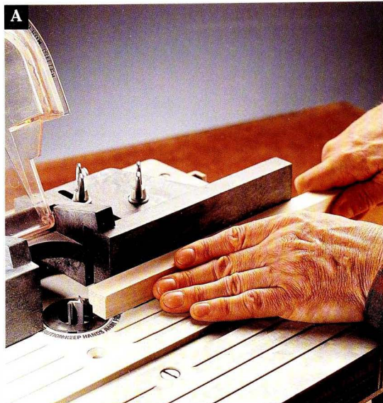
Use a router table and straight bit to cut the rabbets on the frame pieces.
