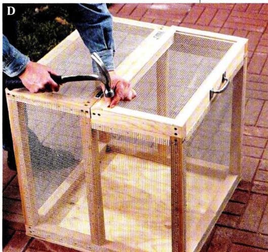
Cut pieces of trim to size, then nail them over the edges of the screen.
