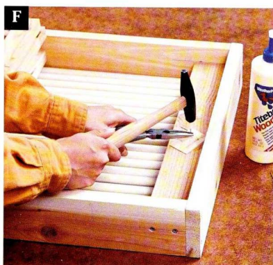
Fasten the stationary leg frame to the lower hinge support on the underside of the tray frame.
