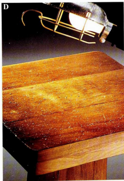
Examine the surface after each coat of polyurethane dries, using a bright side light.
