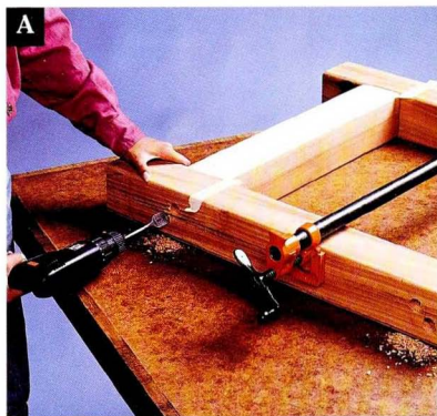
Counterbore two sets of holes on each leg to recess the lag bolts when you attach the legs to the stretchers.
