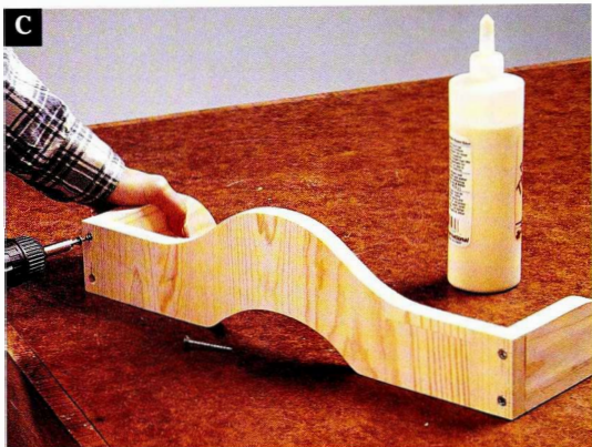
C Fasten the wings to the back rail with glue and screws.
