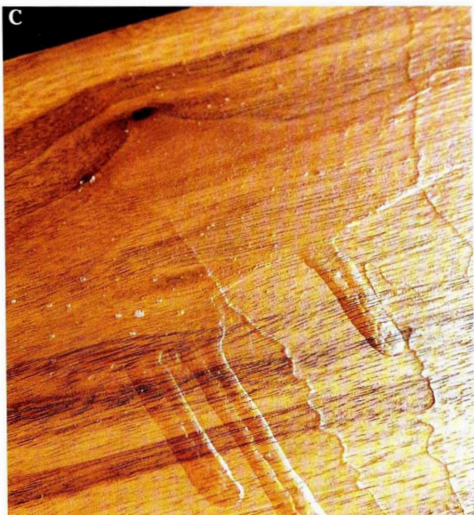
Applying too much finish at once causes running, wrinkling or sagging.
