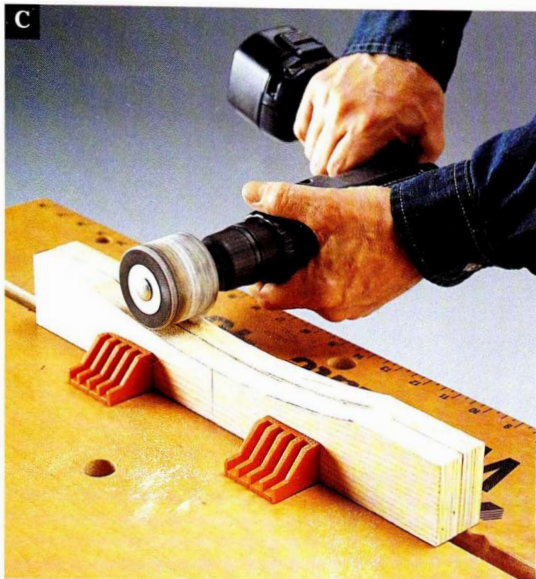
Clamp the stretchers together and sand the arcs smooth, using a drum sander attached to a drill.
