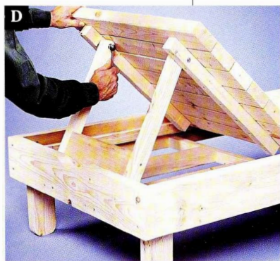
Use a washer and nylon locking nut to fasten the back braces to the back supports.
