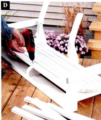
Install the finished slats, started at the crook and covering the seat and back. Space the slats evenly.
