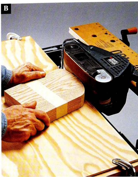
B Tape sides together and sand the corners to create identical profiles.
