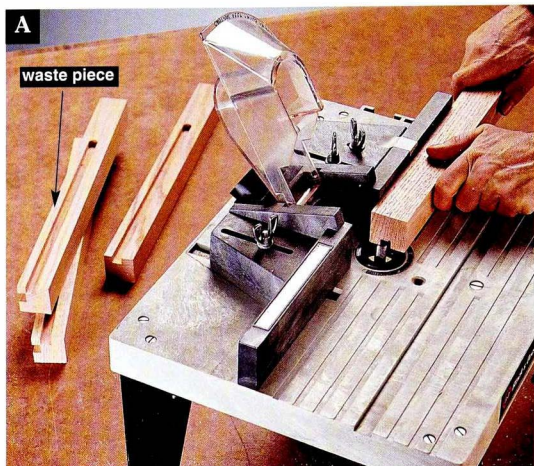
Cut \frac{1}{2} \times \frac{3}{8} "-deep stopped dados in the legs, using a router table. Note the waste pieces on the back legs, which you will need to remove with a handsaw and chisel.
