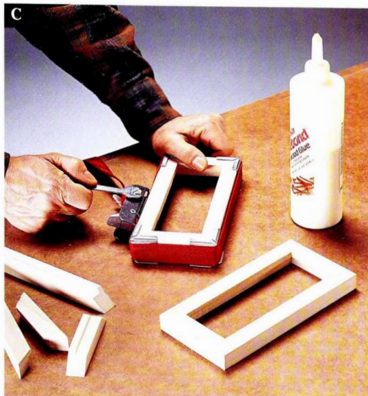
Join the frame pieces with glue and secure them with hand clamps until the glue dries.
