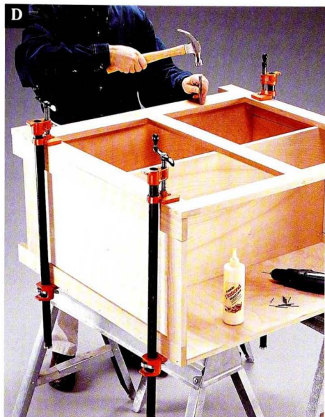
Clamp one side of the face frame and check for square, then clamp the other side and check for square again. Attach with finish nails and set the nailheads.
