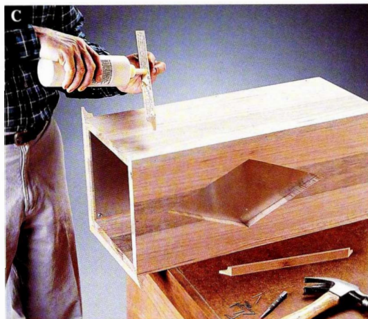
Attach the cove molding to the sides with glue and 1" brads.
