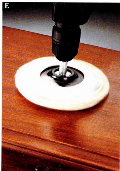
Buff wax to a hard, glossy finish with a polishing bonnet attached to a portable drill. Keep the drill moving to avoid overheating the wax.
