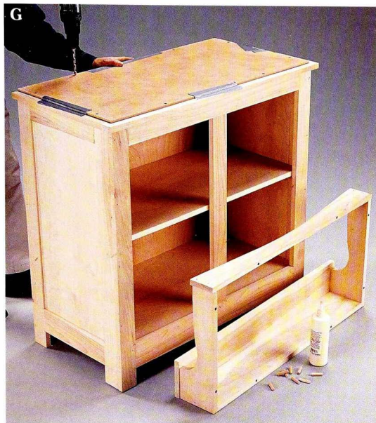
Use a template to ensure that the dowel holes in the top assembly will match those drilled in the top of the cabinet.
