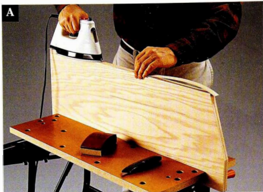
Apply oak-veneer edge tape with a household iron, and trim with a utility knife when cool.
