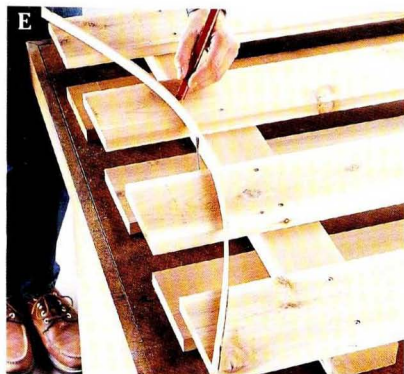
Use a flexible guide to mark the top contours.
