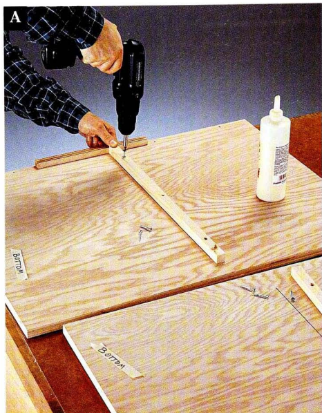
Use a \frac{3}{4} " piece of scrap wood as a spacer to inset the cleats \frac{3}{4} " from the back edges of the side panels.
