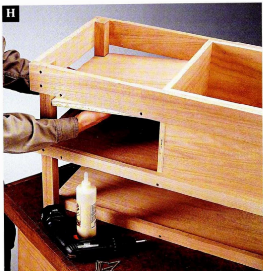
H Glue the bin bottom between the credenza sides, flush with their bottom edges, and secure it with screws.
