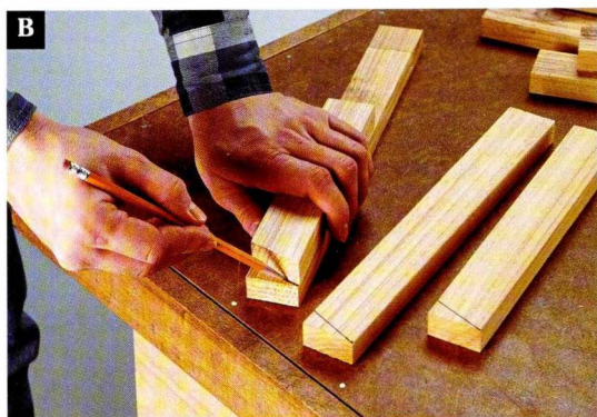
Make a miter cut at the top of one slat, then use that slat as a guide for marking miter cuts on the rest of the slats.
