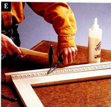
Center egg-and-dart trim molding under the cap, and attach it with glue and brads.
