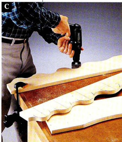
C Sand the curves with a drum sanding attachment and a drill.
