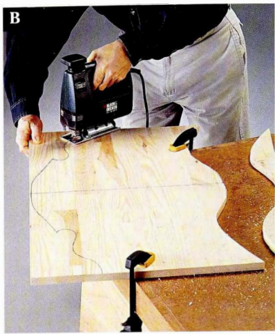
Clamp the back to your worksurface, and cut the pattern, using a jig saw.
