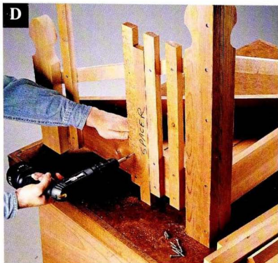
D Use one slat as a spacer to set the correct gap as you fasten the slats to the bin and the stringers.
