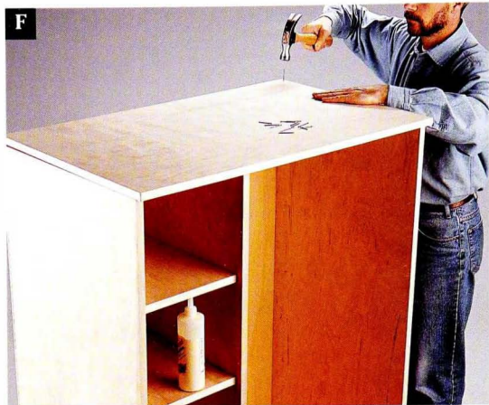
F Mount the top panel so it covers the top edge of the back panel and overhangs the front edges of the side panels by \frac{3}{4} ".
