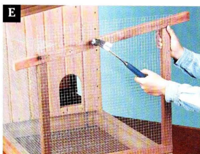
After folding and attaching the hardware cloth to the back, cut off excess cloth.
