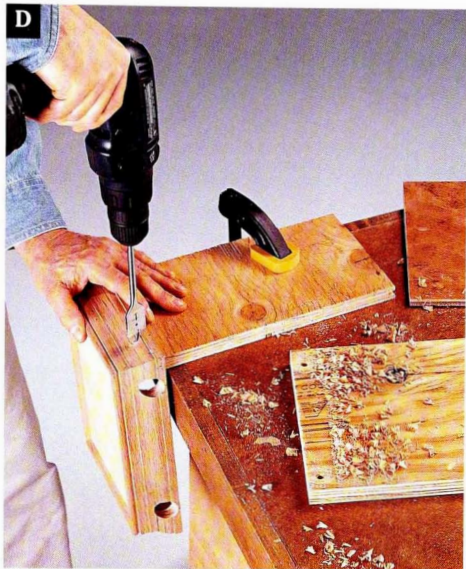
Use scrap plywood to support trivet and prevent tearouts while drilling "leg" holes in the molding.
