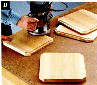
Cut decorative profiles along the edges of the inner and outer plates.
