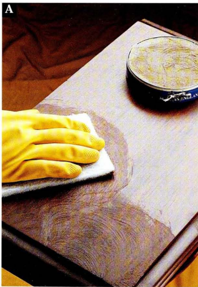
Apply a moderate layer of paste wax by rubbing the wax into the wood with a polishing motion.
