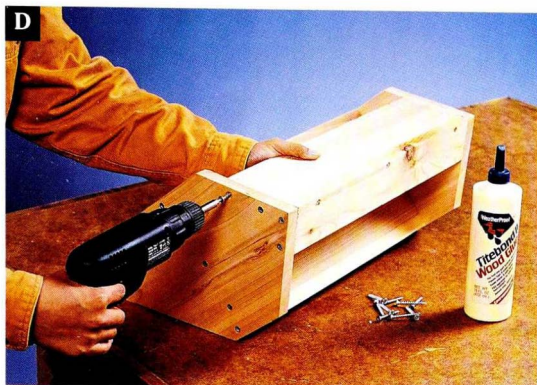
Keep the lip edges flush with the side edges to form the newspaper shelf.
