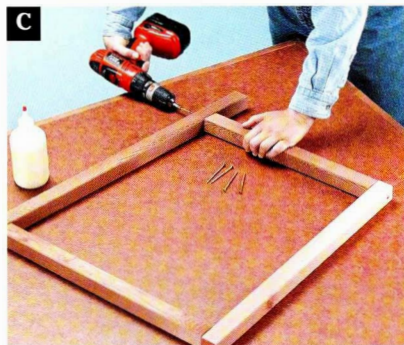
Attach the frame top to the frame back, sides, and base to create the cage side.
