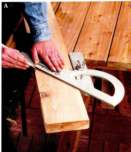
Use a saw protractor to mark a 50^\circ angle on the end of the table leg, then cut the angle using a circular saw.
