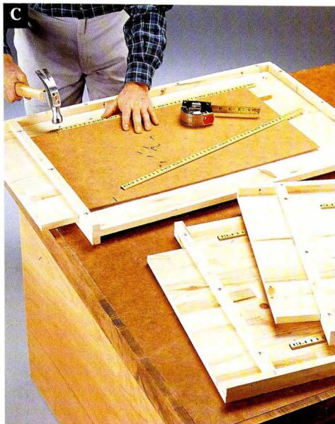
C Center a marked template between the cleats to uniformly attach the shelf standards.
