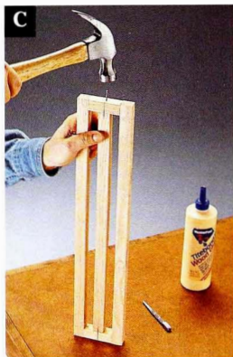
Glue and nail divider in place.
