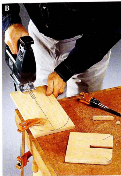
Clamp pieces to your work surface to ensure steady cuts.
