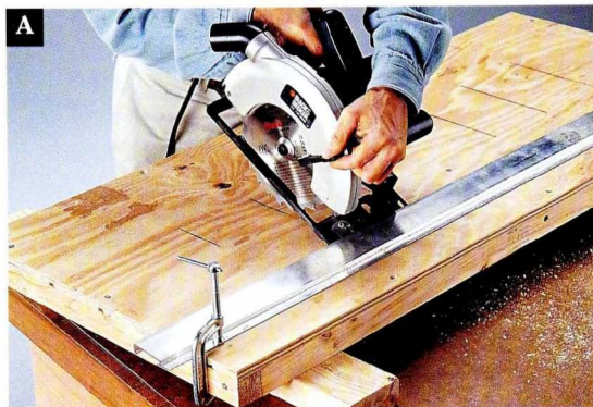
For ventilation, cut slots into the bottom panel, using a straightedge as a stop block for the foot of your circular saw.
