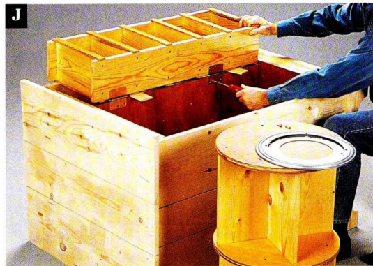
J With spacers in place to help align the parts, attach the swing-out rack to the divider with 3 \times 3 " butt hinges.
