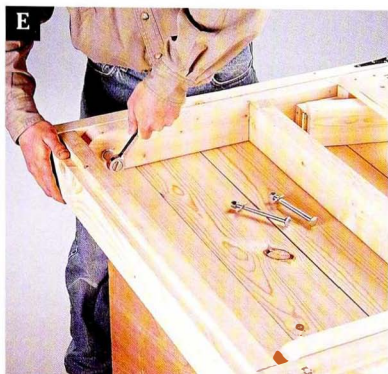
E Fit the legs into place and attach them with carriage bolts, washers and lock nuts.
