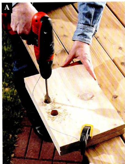
Mark the angled cut-offs. Drill holes for the handles, then cut away the remaining material.
