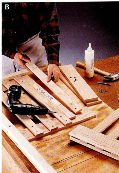
Attach the end slats to the outer rails with glue and wood screws, using a spacer as a guide.
