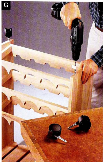
Drill holes for the casters in the bottom edges of the sides.
