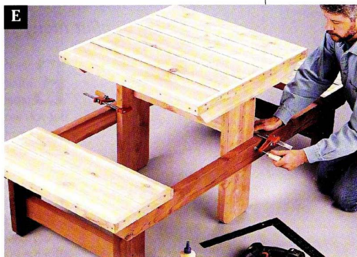
E Center the table within the cross rails, and clamp it in place.
