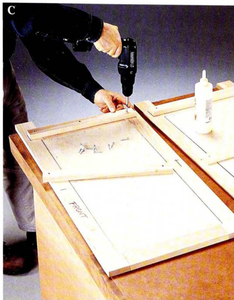
Drill pilot holes, and attach cleats with wood screws to the frame but not into the \frac{1}{2} " panel.
