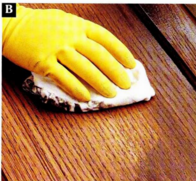
Remove excess stain with a clean, lint-free cloth. Wipe against the grain first, then with the grain. If the color is too dark, try scrubbing with water or mineral spirits. Let the stain dry, then buff with a fine abrasive pad.
