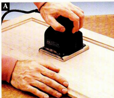
Use a finishing sander on flat surfaces and specialty sanding blocks on contours.
