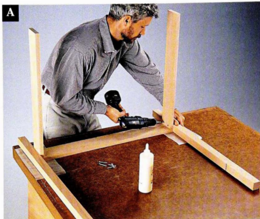
A Fasten the apron assembly between the back legs with glue and wood screws.
