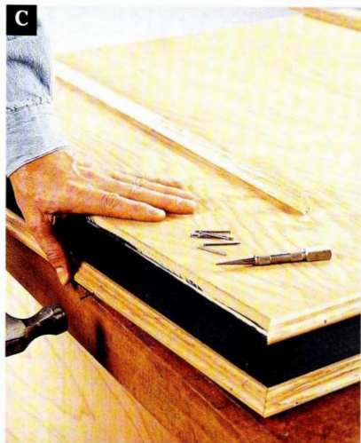
C Glue and nail oak trim around the tabletop and apron, making mitered joints at the corners.
