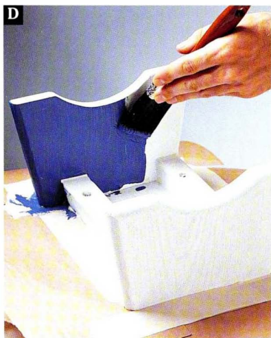
Apply a thin coat of paint, brushing with the grain.
