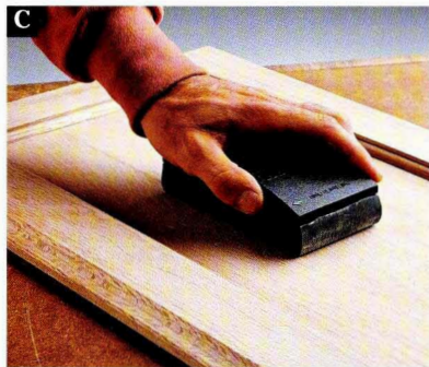
Use sanding blocks to hand-sand the entire workpiece with the finest-grit paper in the sanding sequence.
