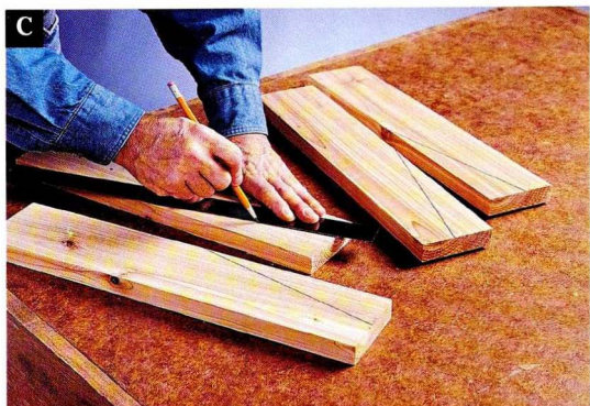
Use a jig saw or circular saw to cut the leg tapers.
