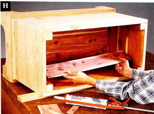
Install aromatic cedar panels to the sides, ends and bottom, using panel adhesive and 2d finish nails.
