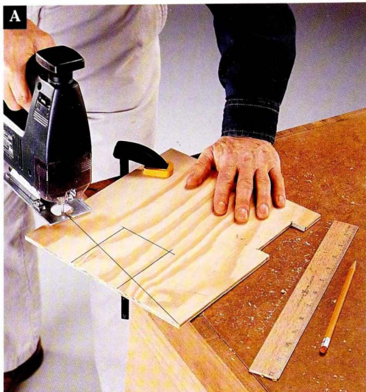
Use a piece of \frac{1}{4} " scrap plywood and your jig saw to create the mortising jig.
