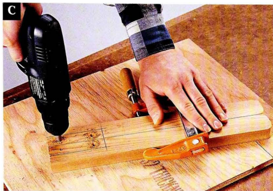
Drill and counterbore pilot holes in the posts before you attach them to the handle and divider.
