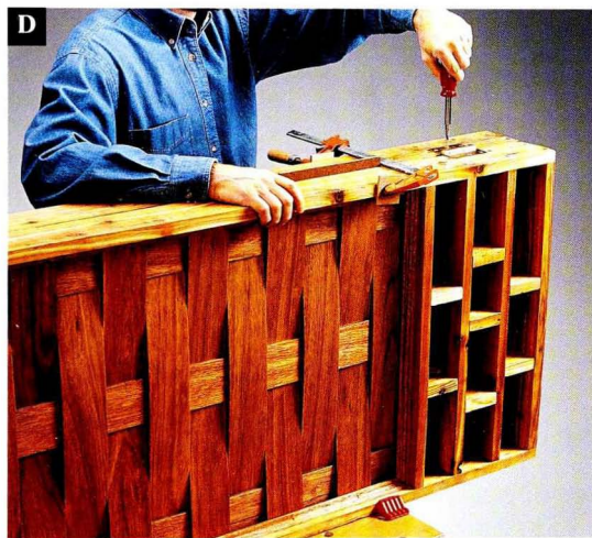
Connect the divider sections with brass butt hinges.
