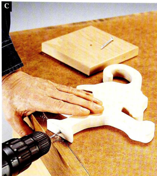
C Drill a pilot hole into the base of the monkey so it doesn't split when attaching it to the platform.
