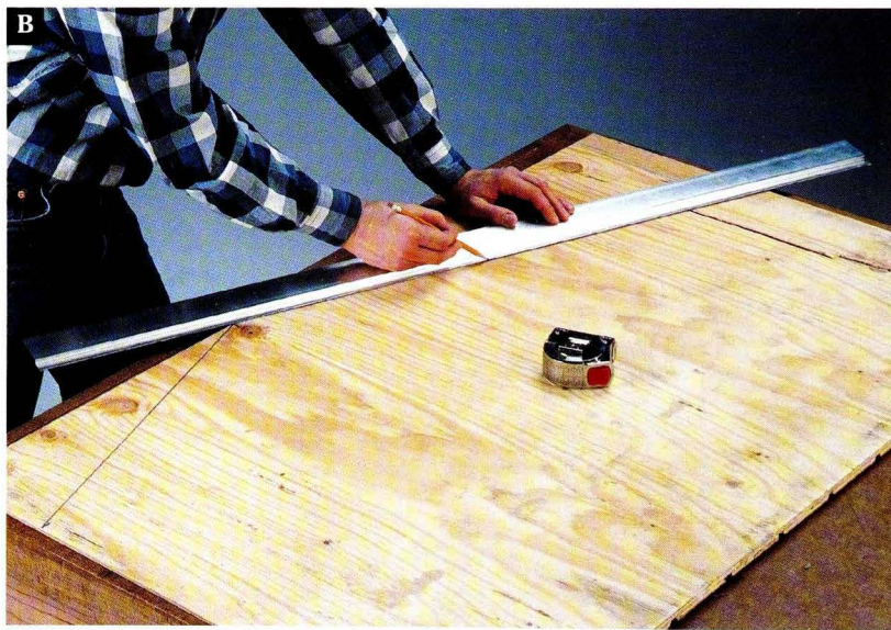
Lay out the roof angle on the side panels using a straightedge.
