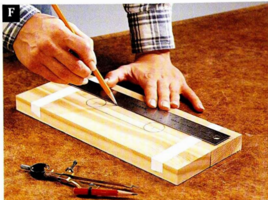
Tape the tray ends together. Then, draw a slot across the joint to mark identical handle cutouts.
