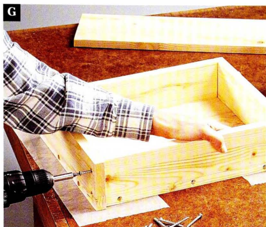
Fasten the drawer sides to the drawer ends and drawer bottom with glue and screws.
