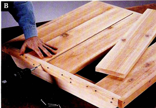
Install the tabletop slats by driving screws through the tabletop frame and into the ends of the slats.
