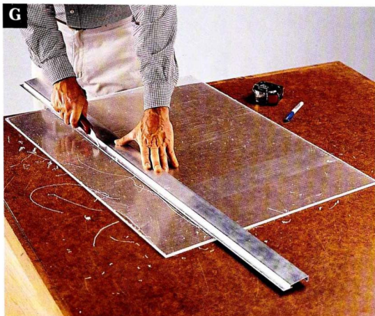
Score the acrylic sheet repeatedly, using a plastic cutter and a straightedge as a guide.
