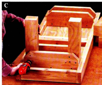
Position each leg between a set of braces and against the sides of the bench frame. Drill pilot holes through each brace and attach the leg to the braces.
