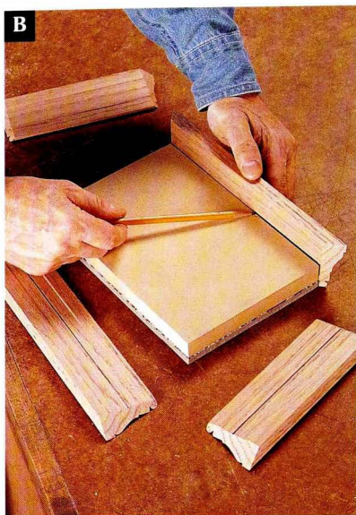
Test-fit the base molding side and end pieces to the substrate and tile before applying glue.
