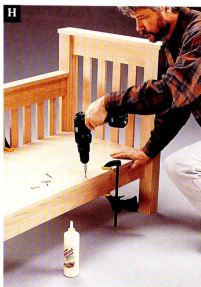
Attach the platform to the rails, frame face and support frame with glue and wood screws.
