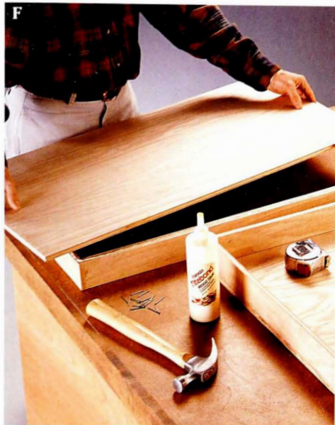
Assemble the drawer boxes and attach the bottoms with wood glue and brads. Make sure to check for square as you build each drawer.
