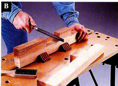
Smooth out the post notches with a wood file.
