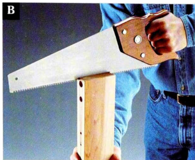
B Drill holes of varying diameter to create an outline, then cut a slot for the tail into the shaft.
