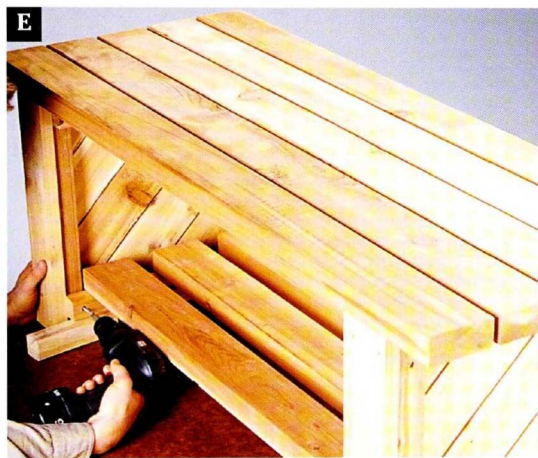
Attach the bottom cleats to the end frames with deck screws. Use a spacer to keep the cleat \frac{1}{4} " up from the bottom of the bench.
