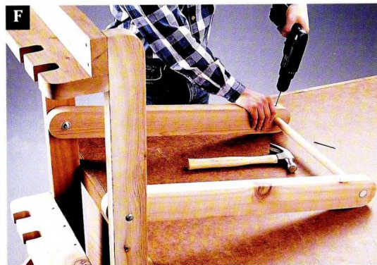
F Drill a pilot hole through each arm and into the ends of the handle, then drive 4d finish nails into the holes to secure the handle.
