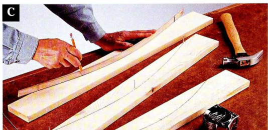
Use a flexible marking guide to draw the arches in the front rails.
