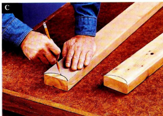
A piece of cardboard acts as a template when you trace the outline for the arc on the cross beams.
