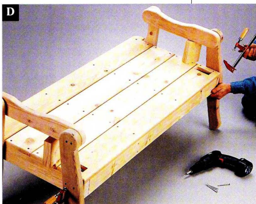
D Carefully clamp the leg frames to the seat, and attach them with glue and screws, driven through centered, counterbored pilot holes.
