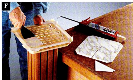
Frame the top of the top outer plate with masking tape, then apply a layer of construction adhesive to attach the sundial face.
