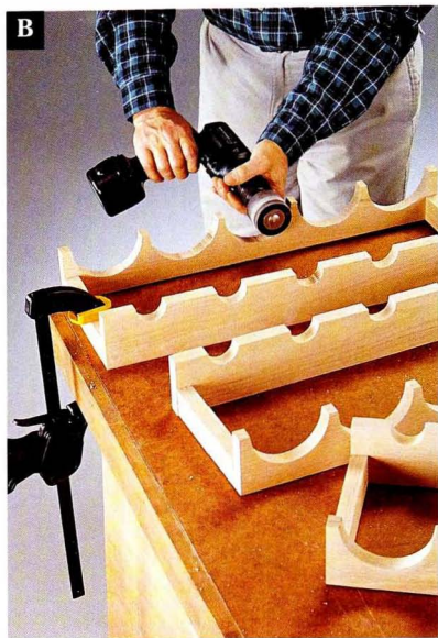
Use a drum sander attached to your portable drill to smooth the jig saw cuts on the wine racks.
