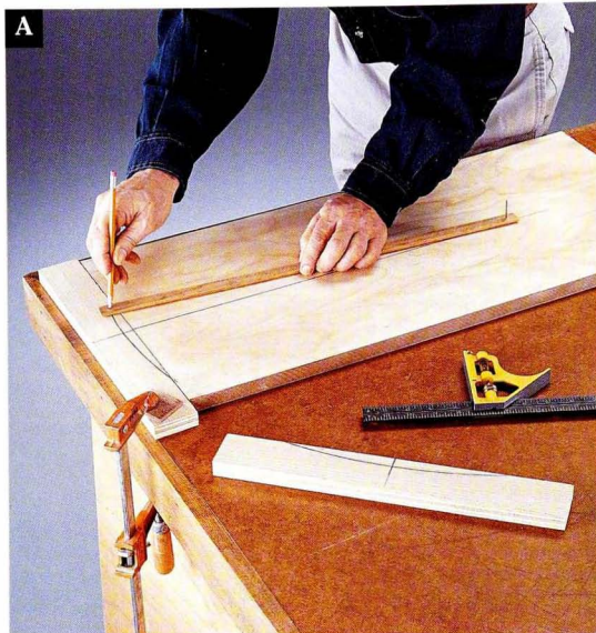
Use a makeshift bar compass to achieve smooth, uniform arcs on the front stretchers.
