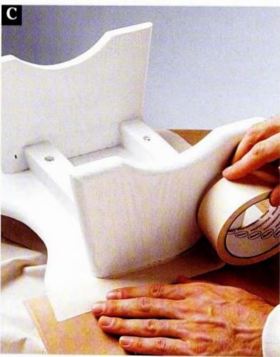
Mask any adjacent areas that will be painted a different color, using masking tape.
