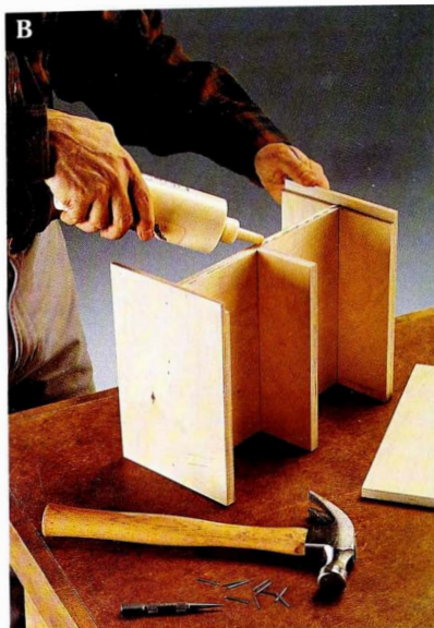
Apply glue to the shelf, the divider and the shoulders of the rabbets before attaching the back.
