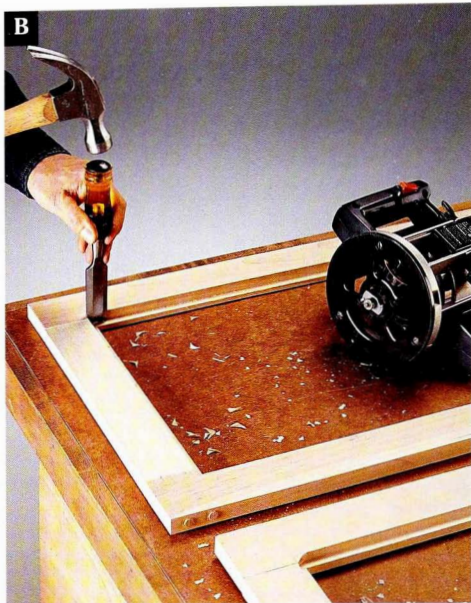
B Carefully square the corners of the rabbets in the side panels and door panels, using a sharp chisel.
