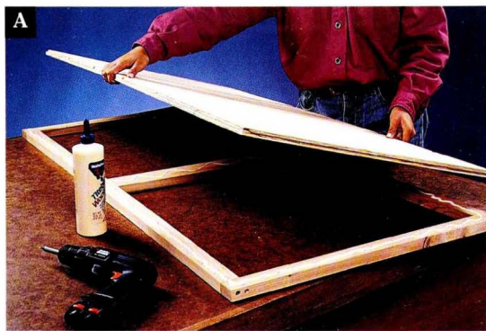
A Cut and fasten the lid to the lid framework with the grooves in the panel running back to front.
