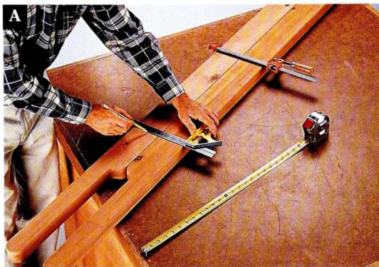
A Clamp the handles together and draw reference lines at the stringer locations.
