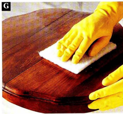
G Dab a few drops of penetrating oil onto a fine abrasive pad, then rub the surfaces until smooth. Let the oil dry for at least 72 hours before applying a topcoat. If you do not plan to topcoat the finish, buff with a soft cloth to harden the oil finish.
