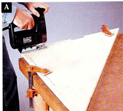
Use a jig saw to cut notches for the standards in the back edges of the center shelf.
