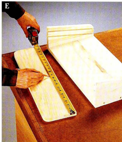
Find the center of the assembly and mark on the base and back to properly place the screw holes.
