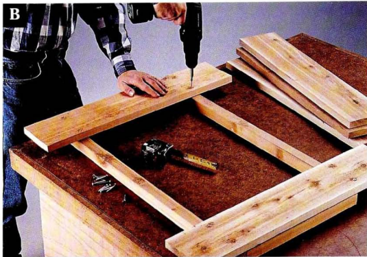
Attach a slat at each end of the panel frame so the outer edges of the slats are flush with the outer edges of the frame.
