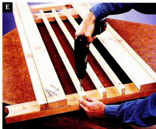
Attach trellis strips to the cross brace and spreader with deck screws.
