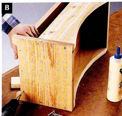
Attach the shelves by driving deck screws through the end pieces and into the ends of the shelves.
