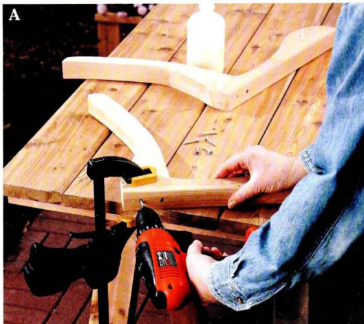
A Make sure the inside corner is flush, then attach each seat support to a back support with glue and galvanized screws.
