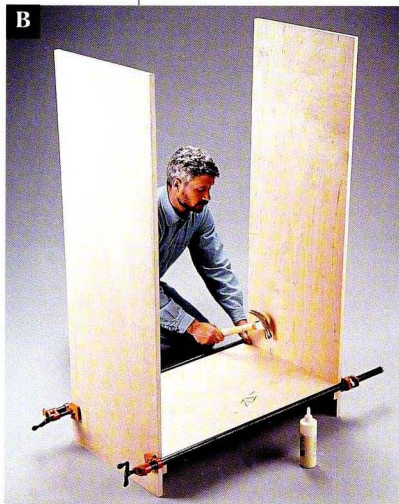
Clamp the bottom panel between the sides and fasten it to the cleats with glue and finish nails.
