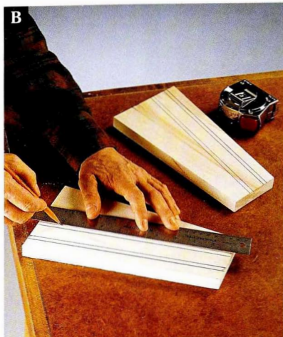
Draw lines to mark the placement and width of the dados.
