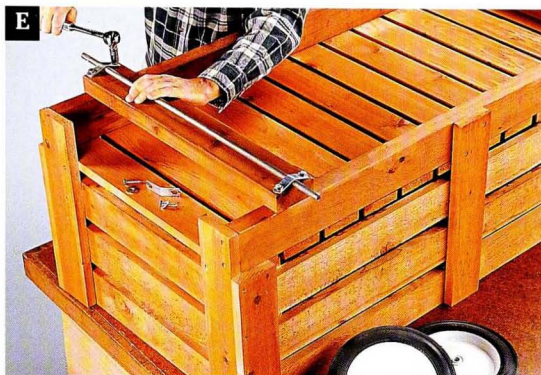
Attach the axles to the bottom of the front stringer with metal straps fastened with lag screws.
