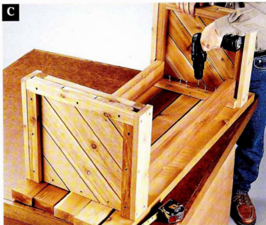
Use shelf slats to set the correct distance between the end-frame assemblies, then attach the end frames to the bottoms of the seat slats.
