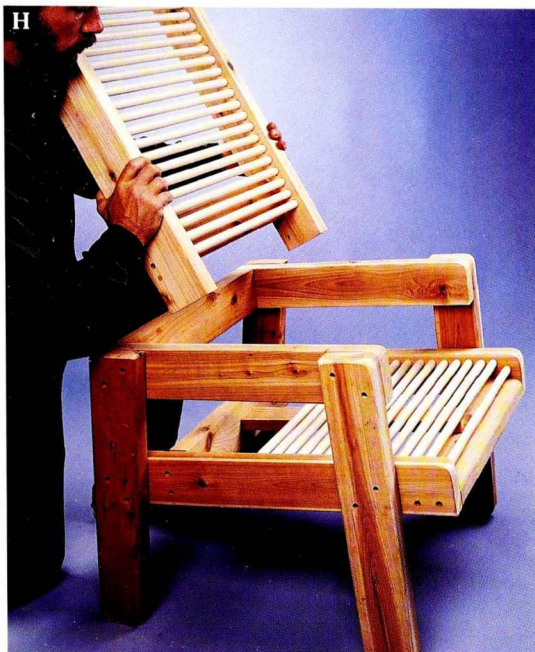
Slide the back frame into the seat frame so the back sides rest against the seat stop and seat support.
