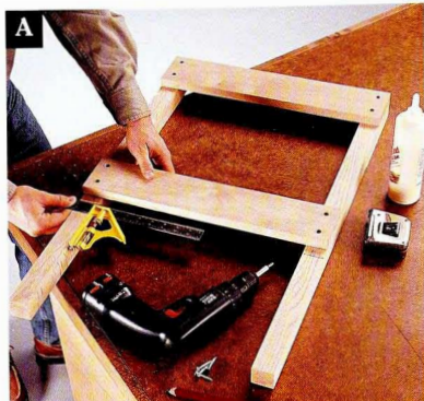
Check with a combination square to make sure the desk legs are square to the ends.
