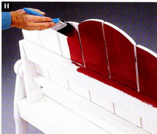
H Apply two thin coats of exterior primer to seal the pine, then paint the park bench with two coats of enamel house trim paint.
