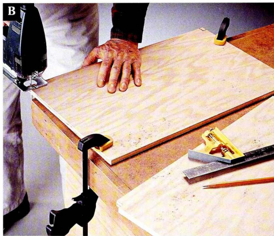
Cut a \frac{3}{8} \times \frac{1}{2} " notch out of the bottom corners of the back and side panels where they will overhang the dados in the legs.
