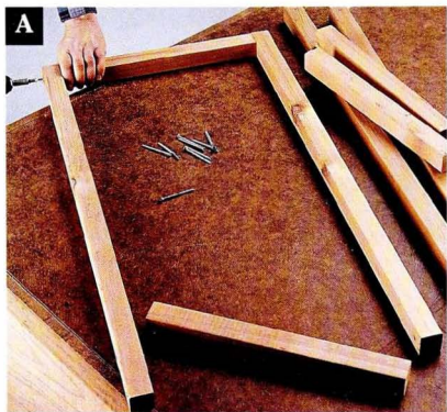
Fasten the cleats between the rails to construct the panel frames.
