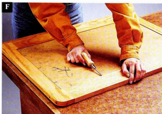
Install the mirror and mirror back. Then, secure them to the frame with brads, using a brad pusher.
