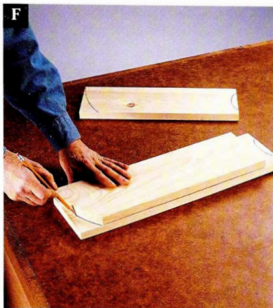
F Use the first completed back slat as a template for tracing cutting lines on the rest of the back slats.
