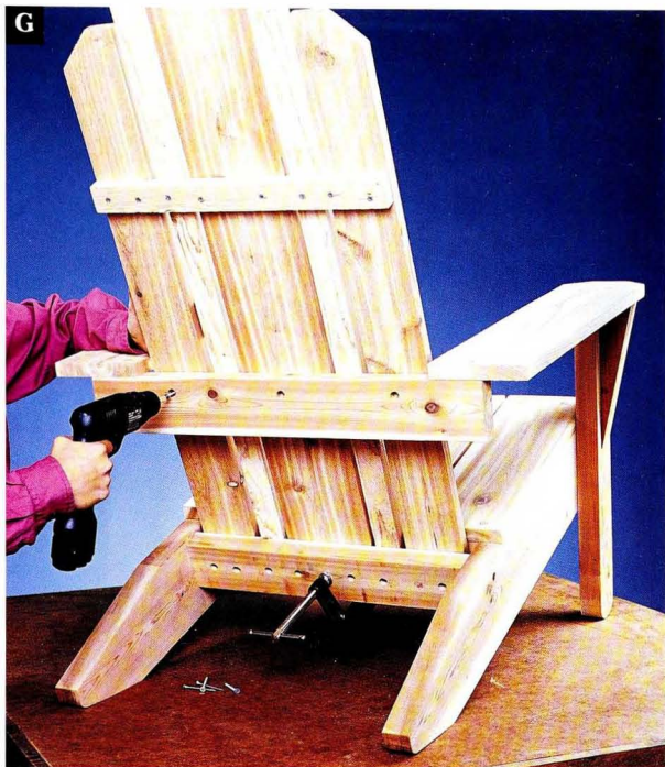
Drive screws through the arm cleat, near the top, and into the slats.
