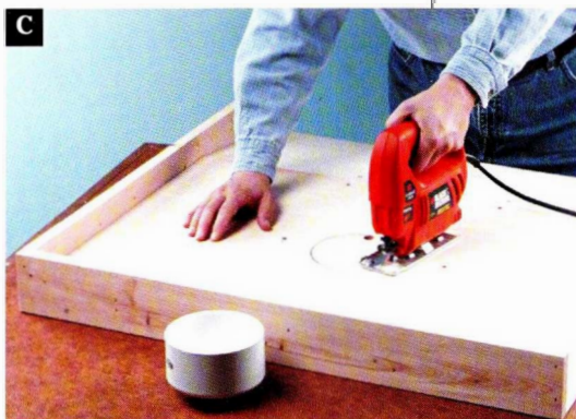
Drill a starter hole to insert the blade of a jig saw, then cut out the cup hole.
