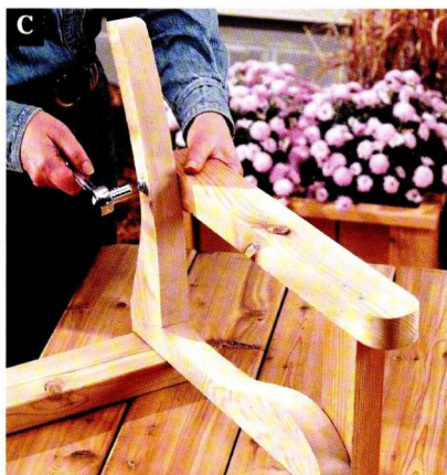
C Drill a hole through the back support into the arm and attach it with a lag screw.
