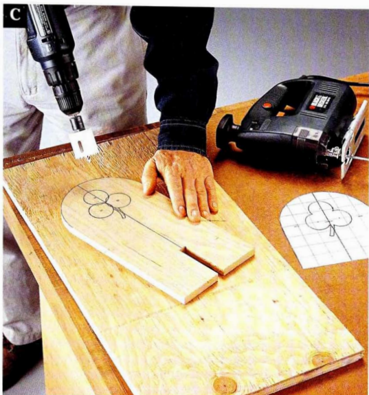
Use a hole saw to cut quickly and cleanly. Place a backer board underneath to prevent tearouts on the other side of handle.
