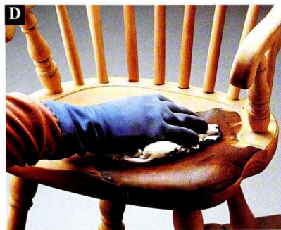
D Gel stain penetrates better if it is worked into the wood with a brush or rag, rather than simply wiped onto the wood surface.
