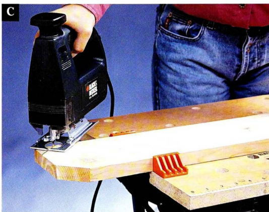
Make decorative cuts on the fronts of the arms (shown) and the tops of the back slats, using a jig saw.
