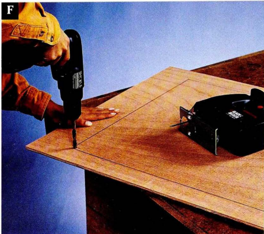
F Drill a \frac{1}{8} "-dia. hole on the inside of one of the corners of the door lay-out, then cut out the door opening with a jig saw.
