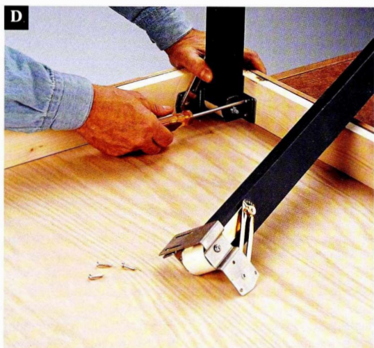
D Attach the card-table leg fasteners to the rounded ends of the legs. Then, attach them at the inside corners of the tabletop frame.
