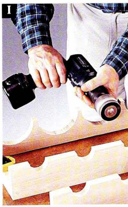
I Smooth curves and hard-to-reach surfaces with a drum attachment on your power drill.
