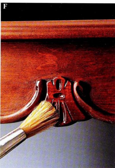
Use liquid wax on detailed areas, where paste wax is difficult to apply. Apply the wax with a stiff brush, then buff with a soft cloth.
