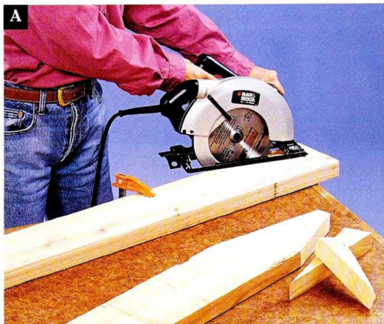
Cut tapers into the back edges of the legs.
