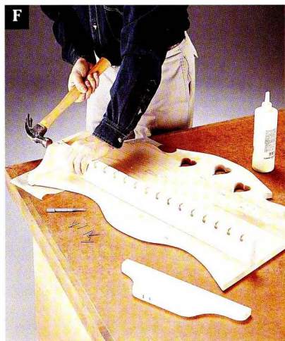
Attach the shelf to the sides with finish nails and to the back with wood screws.
