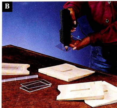
B Cover the viewing slots by hot-gluing clear plastic or acrylic pieces to the inside face of each panel.
