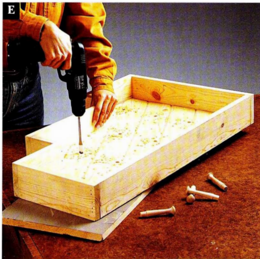
Measure and mark peg locations on the backing, then drill peg holes with a spade bit. Do not drill all the way through the backing.
