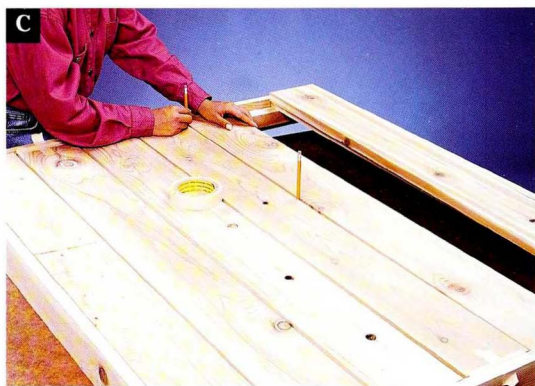
Use pencils or dowels to set even gaps between top slats. Tape slats in position with masking tape.
