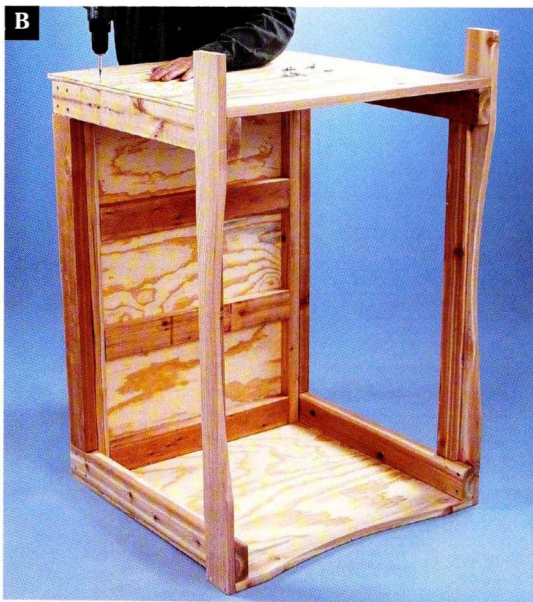
Attach the plywood cabinet sides and the cabinet base to the cabinet frame with 1 1/4" deck screws
