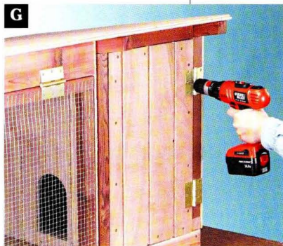
Mount the doors with 3" hinges.
