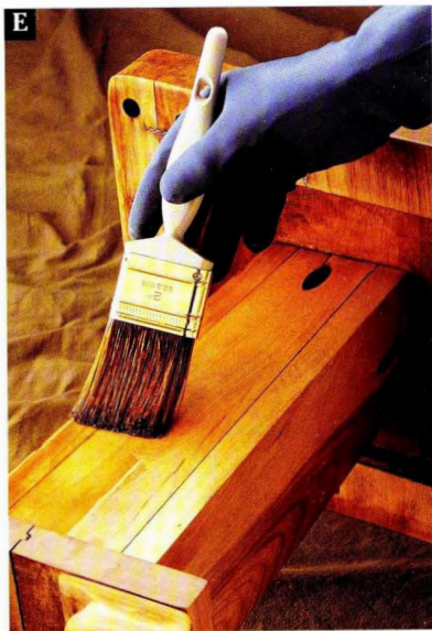
To keep the finish from running, always try to position the workpiece so the surface being topcoated is horizontal.
