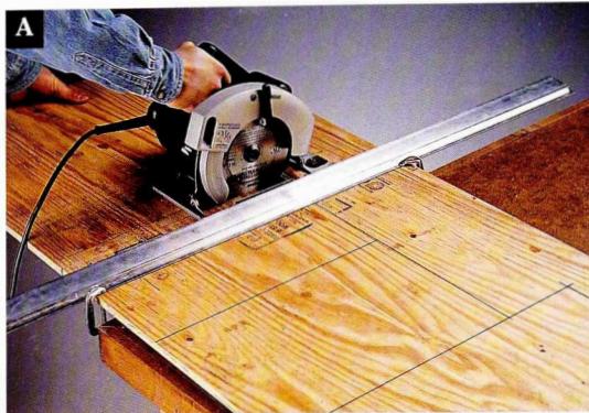
Cut the end panels and side panels to size using a circular saw and a straightedge cutting guide.
