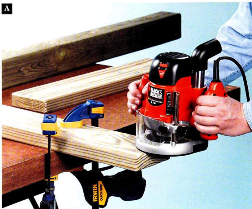
Round the top edges and ends of the balance beam with a router.
