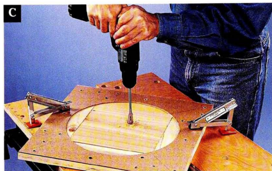
Drill a starter hole for the router bit in the centers of the components.
