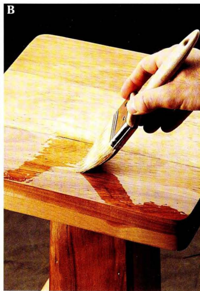
B Apply a coat of polyurethane, starting at the top of the project and working your way down.
