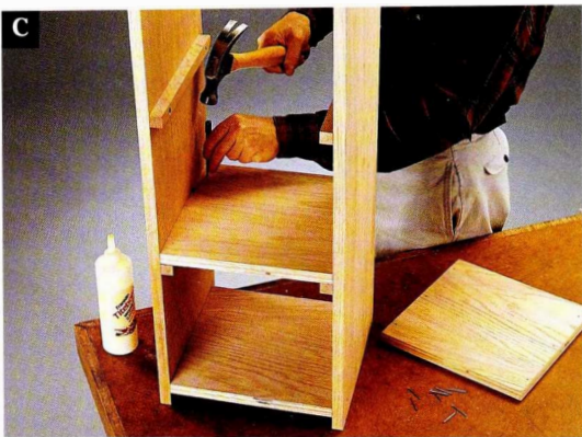
Use a nail set to recess nail heads flush with the shelves.
