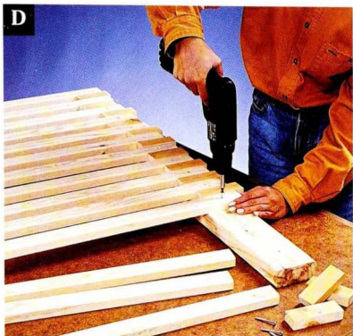
Use 1 × 2 spacers to align the back slats, then fasten the slats to the back cleat.
