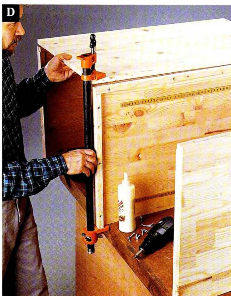
D Clamp the back to the divider along the centerline, and adjust when attaching to the end.
