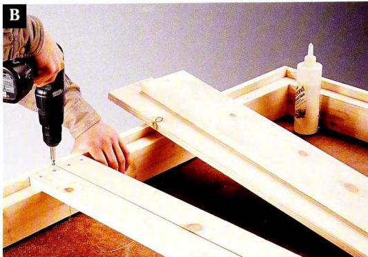
The middle slat is rip-cut in half and attached on each side of the hinged joint between the sides of the tabletop frame.
