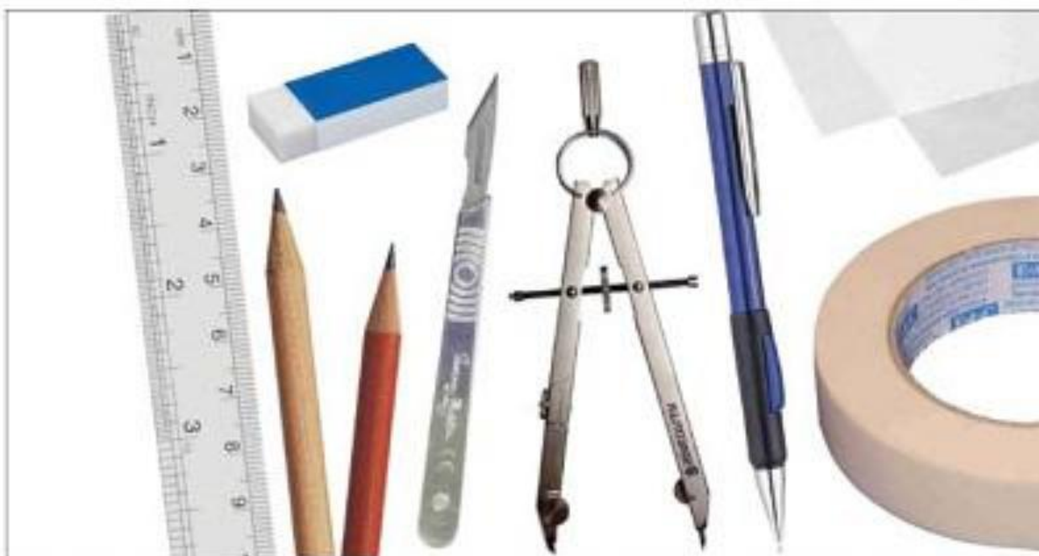
The basic essentials in terms of drawing equipment for any new pyrographer (from left to right): a steel ruler, an eraser, a selection of pencils, a craft scalpel, a pair of compasses, an automatic (or mechanical) pencil, tracing paper, and masking tape.
