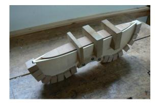
Once all the wedges are in place, the wood is returned to the fish kettle for a last five-minute steam. The wood needs to be steamed in its final form to set the shape. As the wood is cooling all the time that the wedges are being fitted, it is losing its plasticity, so might lose the memory of the final shape once the wedges are removed. By steaming it a final time in its finished state, the wood is "set" and will have the minimum loss of shape.
