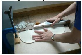
The front is glued and cramped up on a clingfilm-covered wooden board. The board has four screws at the widest point of the upper and lower bouts, and the front is held tight using wooden wedges. Then there's a stretcher cramp to hold the centre and two quick-release cramps at the ends to stop them lifting off the board.
