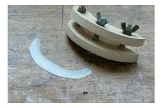
The two halves of the front need to be held together while they are bent. For the upper and lower bouts, I use simple wooden blocks with a 10mm x 10mm slot cut out to receive the wood for the front.
