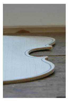
The grain lines are at right angles to the arching across the whole cross section of the front. Looking at the edges of the front, the grain will be at right angles to the plane of the ribs at the top and bottom block areas, and then will tip out to follow the arching in the upper and lower bouts and Cs.
