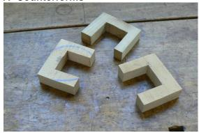
The final piece of equipment you need is three u-shaped blocks of wood to act as counterforms to hold the front against the boat deck wedge. These are made from hardwood, about 15mm thick. The width of the slot corresponds to the maximum height of the boat-deck plus the thickness of the two halves of the front
