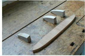
The arching of the front is made by driving wooden wedges between the two halves of the front. I make these from any suitable hardwood that's easy to work; fruitwood, lime or maple are all fine. The two main wedges form the cross-arching of the widest part of the upper and lower bouts. A third wedge just below the lower corners prevents this area from sinking. The final wedge, graphically described by Jane as the "boat deck" gives the shape of the long arch.
