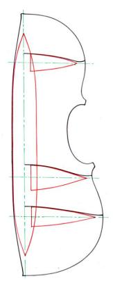
As you can expect the wood to sink once it's been bent and dried, you need to over-bend the wood. I find that a good rule of thumb is to make the width of the "boat deck" wedge at its widest point equivalent to the maximum arching height so that in the central area it follows the external arching of the finished instrument. In effect you're bending the wood to about 5mm higher than the finished instrument.
