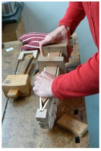
The front, complete with all the cramping blocks, is put in to the fish kettle for an initial steam of ten minutes. Once it comes out, I drive in the cross-wedges as far as they will comfortably go, hitting them with a mallet. Usually they will go in to about three-guarters of their length.
