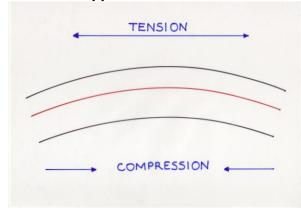
When wood is steam-bent, the outer, convex surface is in tension (stretched) and the inner surface is in compression. In practice, wood can support an increase in compression of up to 30%, but can only support an increase in tension of about 2% before it fails. So most of the change takes place by the inside surface of the front compressing. The diagram shows this – the red line indicates the neutral axis, which is slightly above the middle of the plank. The wood above the red
