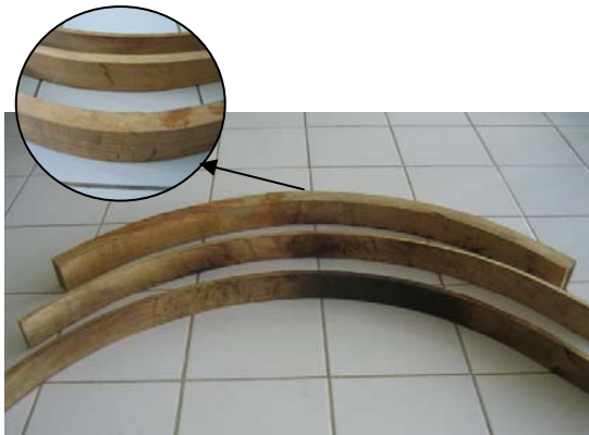
Figure 8. Pinus bent woods with 10 mm, 20 mm, and 30 mm thickness.
