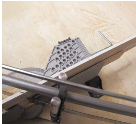
5 Use a well-placed shim to slightly adjust the angle of a bevel cut.
