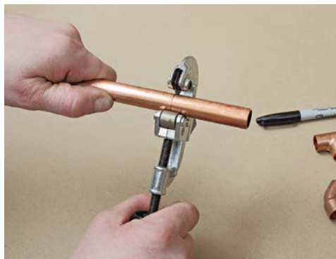
2 Twirl until it gets easy, then tighten and twirl again until the cut is made.
