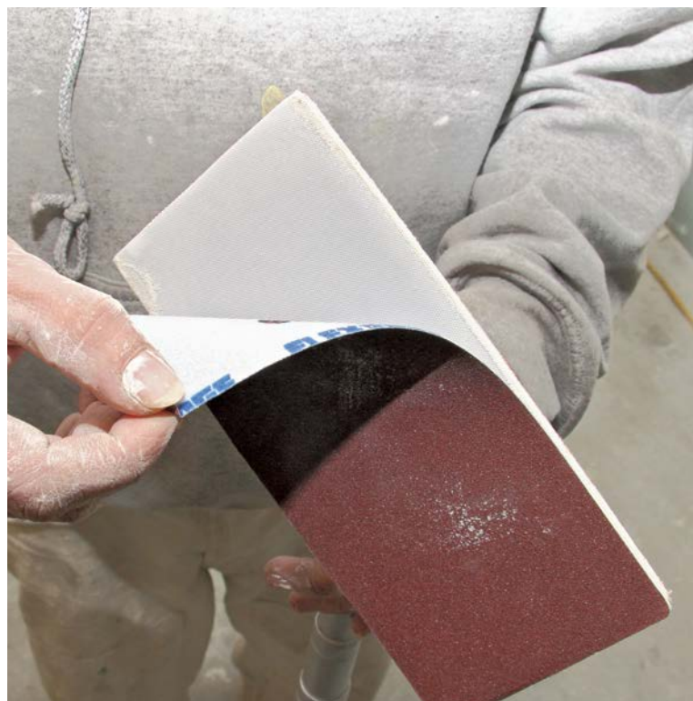
1 This type of sanding block, with paper that does not fold over, works best.
