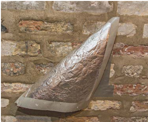
2 After four or five days, pull back the foil or plastic to see if the wall is wet.
