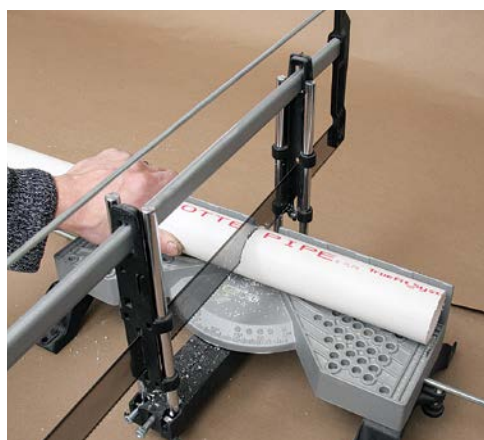
1 Make a straight, clean cut in the PVC pipe.
