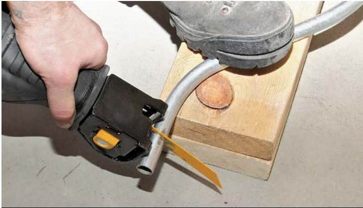
4 Cut conduit with a metal-cutting blade.
