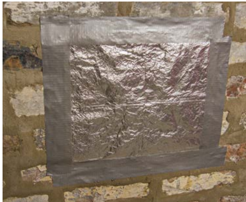
1 Firmly tape a piece of foil or plastic to the wall you are testing.
