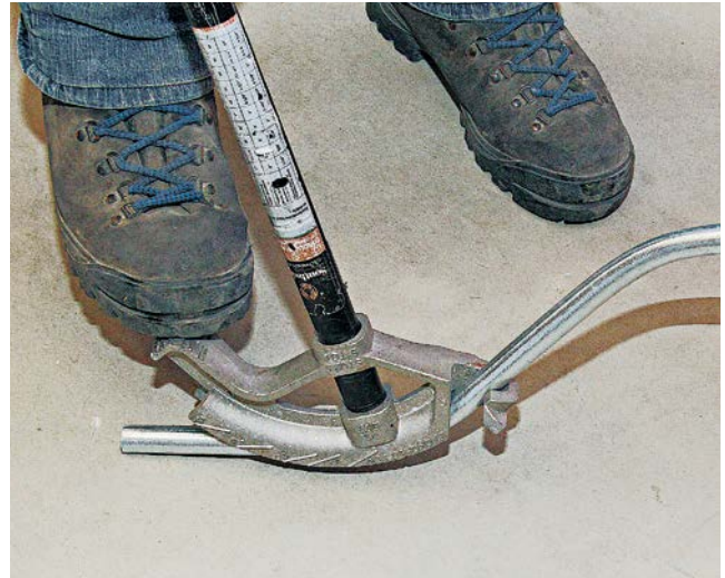
1 Step on the footpad of a conduit bender and pull the bar to make bends in conduit.
