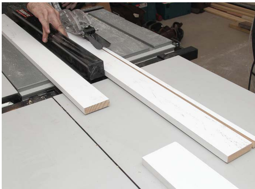
1 Rip-cut 1-by lumber or purchase plain casing.
