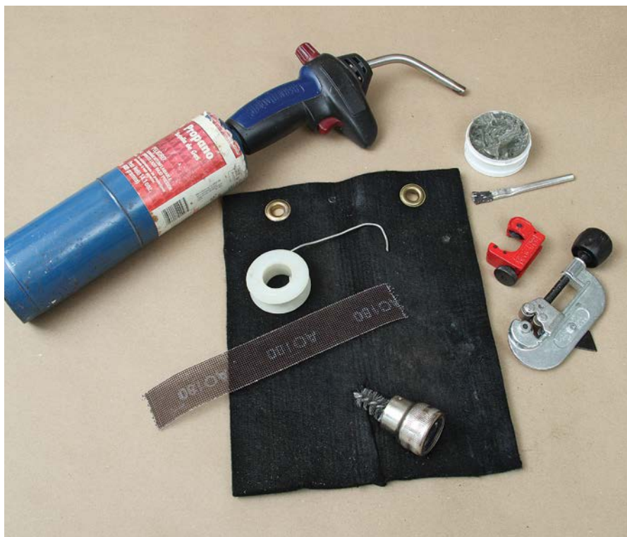
Tools for working with copper: standard-size tubing cutter; small tubing cutter for tight spaces; plumber's tape (sanding mesh); wire brush; flux and a flux brush; propane torch; protective heat shield.
