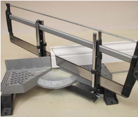
1 Straight-cut and attach the first board, then cut the second at a reverse 45° bevel.
