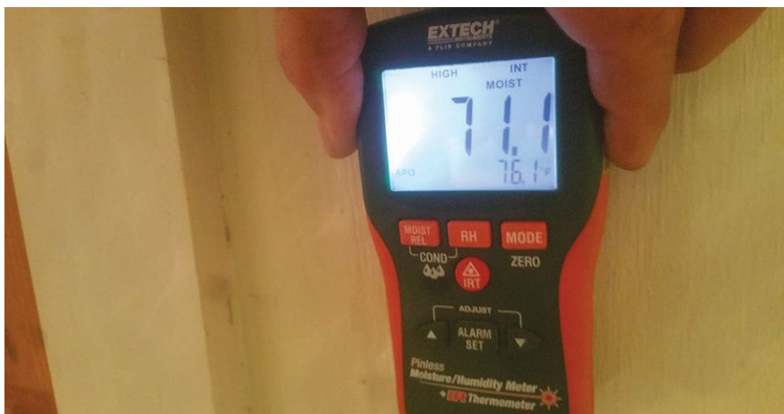
A moisture meter is used to determine moisture levels in various surfaces in the home.
