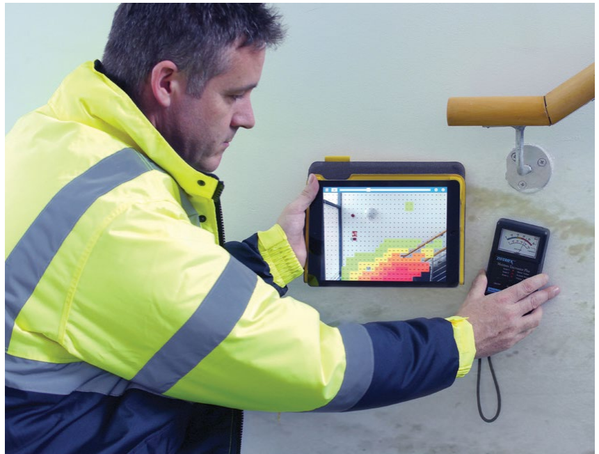
(above) Tramex's moisture mapping app, used in conjunction here with a non-destructive Tramex moisture meter.
