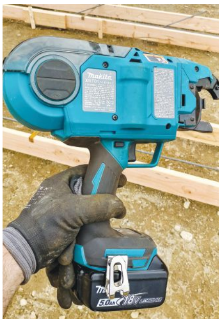
The Makita LXT rebar tier uses #3 wire and has a plastic cover to keep moisture and dirt out of the tying mechanism.
