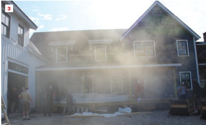
With the building pressurized, fog could be seen escaping from two doghouse dormers at their roof-to-wall junctures (3).
