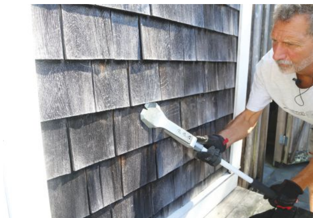
The salvage blade is useful for stripping siding (above left). Other blades include (above right, top row) finish nails; salvage; decking; 8-inch; and (bottom row) \frac{3}{4} -inch; 1\frac{3}{4} -inch; spike puller; 3-inch; 6-inch; and buried nail-head puller.
