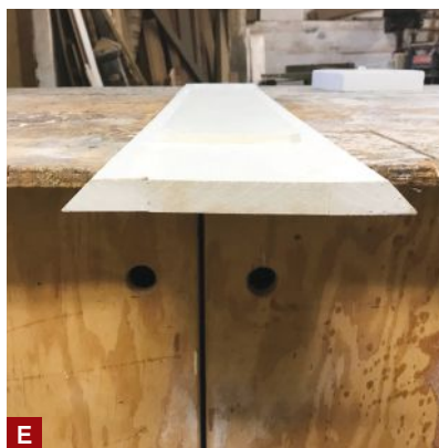
Figure 2. On most frames, the author cut a \frac{3}{8} -inch-deep rabbet with a router around the inside back edge, then glued the \frac{3}{8} -inch-thick PVC panel to the frame. Clipping the panel edges at a 45-degree angle allowed the panels to fit the rounded corners of the rabbet (A, B). For a deeper, \frac{3}{4} -inch panel reveal, the panels could simply be glued and stapled to the back of the frame (C, D). The edges of each frame were ripped to 45 degrees so that they could be glued together to form the post sleeves (E).
