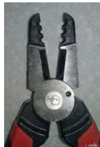
Truncated stripper. Cutting off the smaller slots of a wire stripper makes it easy to find the most-common 14-ga. notch.
