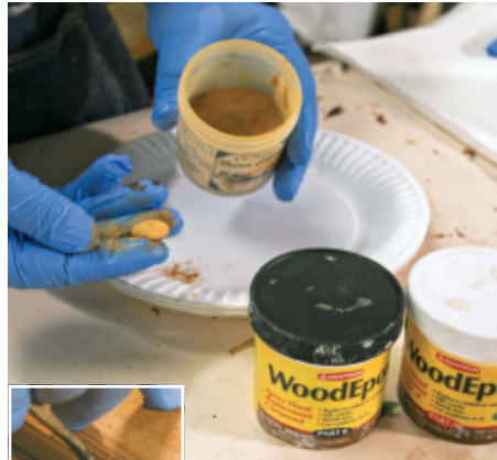
Epoxy for the holes. A two-part epoxy filler mixed with dry pigment creates a tinted filler that's easy to pack into nail holes or blemishes.
