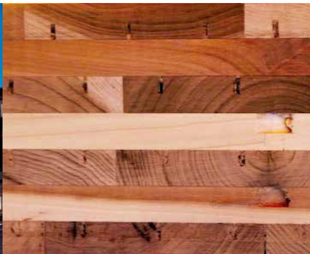
'The Smile' (left) is the first project in the world to use large hardwood CLT panels. A cross-section of the Tulipwood CLT (right).
