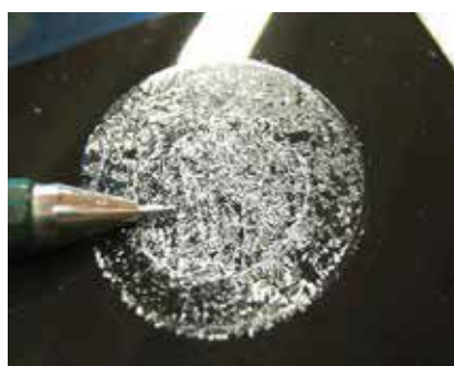
PETG performance after being exposed to acetone for 1 hour.
