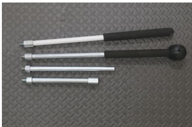
The standard, 25-inch-long steel handle (at top in photo, above left) can be fitted with a ball grip and shorter extensions for more comfort and better leverage. Specialty heads like this nail puller (above right) screw directly onto the handle.
