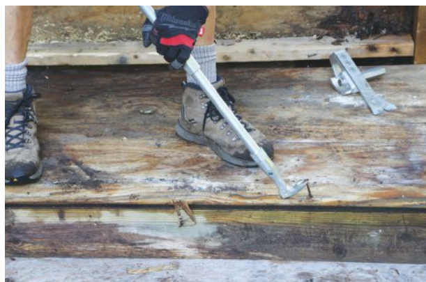
The standard, 25-inch-long steel handle (at top in photo, above left) can be fitted with a ball grip and shorter extensions for more comfort and better leverage. Specialty heads like this nail puller (above right) screw directly onto the handle.
