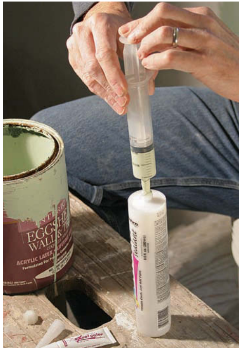
Add paint to the caulk tube. Measure out the specified amount of paint with the supplied syringe, then cap and shake.
