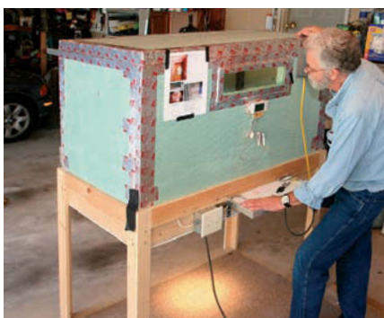
The author tested seven different bulbs in five air-sealing enclosures.
