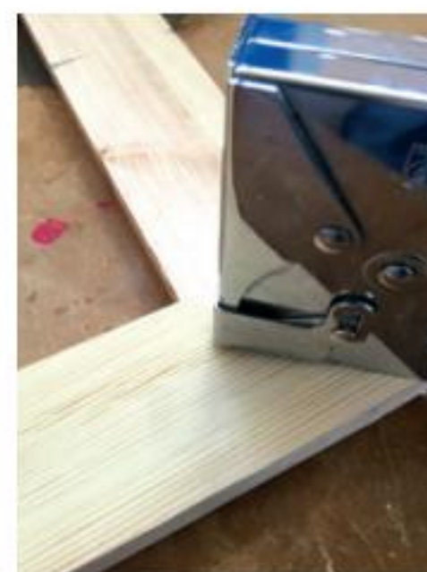
Staples can be used to strengthen the joint
