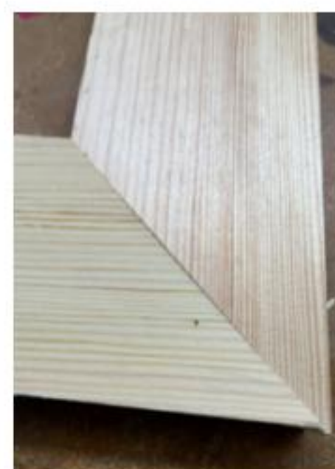
The simplest and quickest way to join the pieces together is to use adhesive
