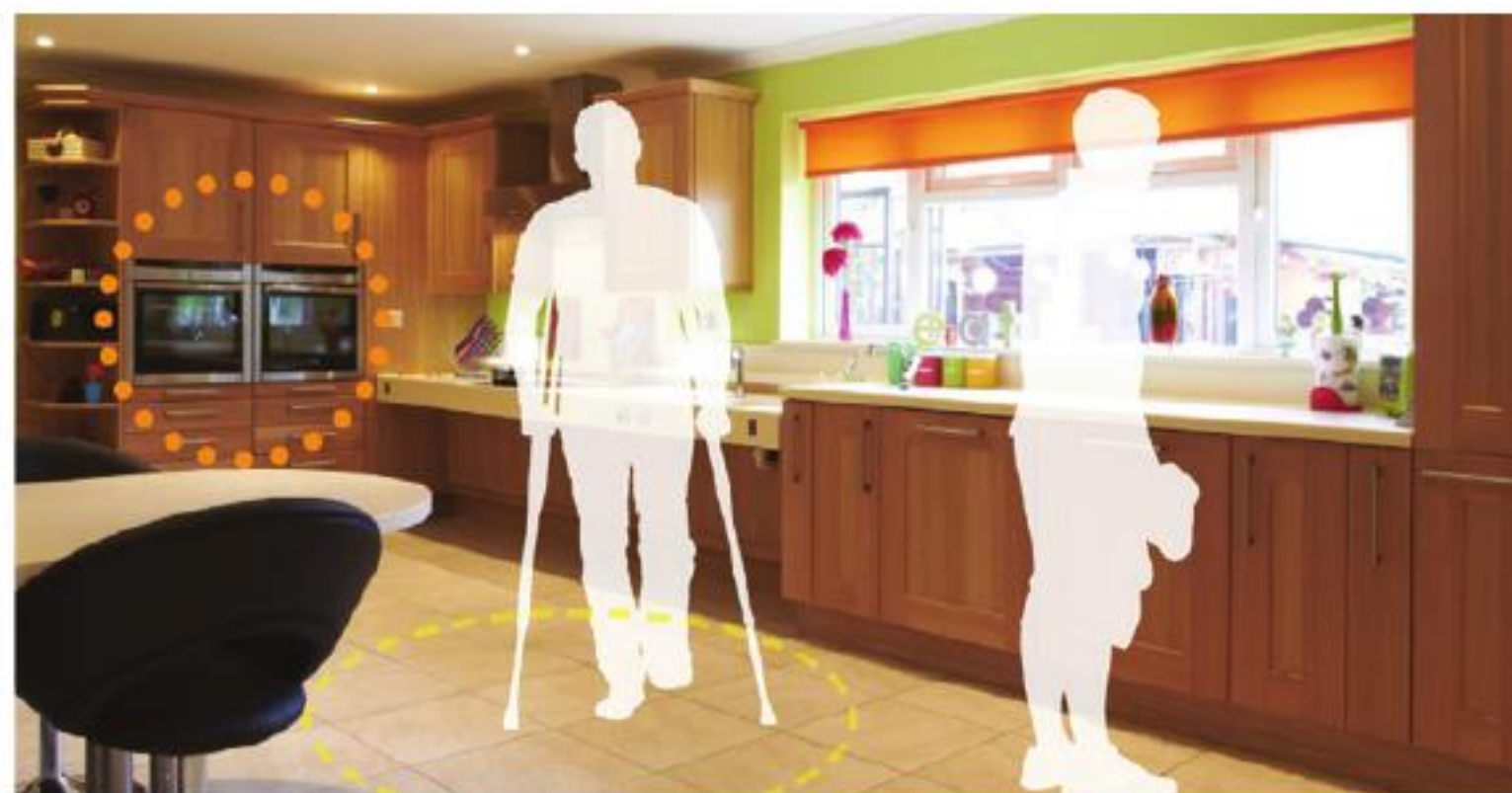
An 'L' shaped plan kitchen and dining area. Note the lower level ovens and toe space under the cupboards.
