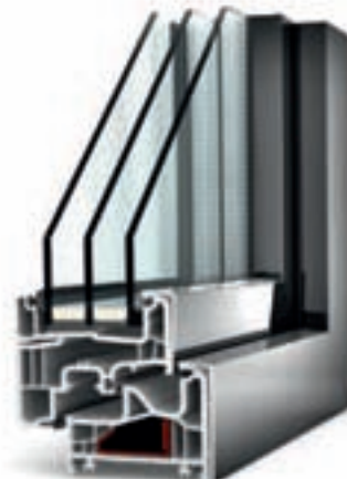
Window system KF 200 U_w up to 0.74 W/m 2 K
