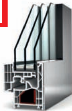
Window system KF 220 U_w up to 0.74 W/m 2 K
