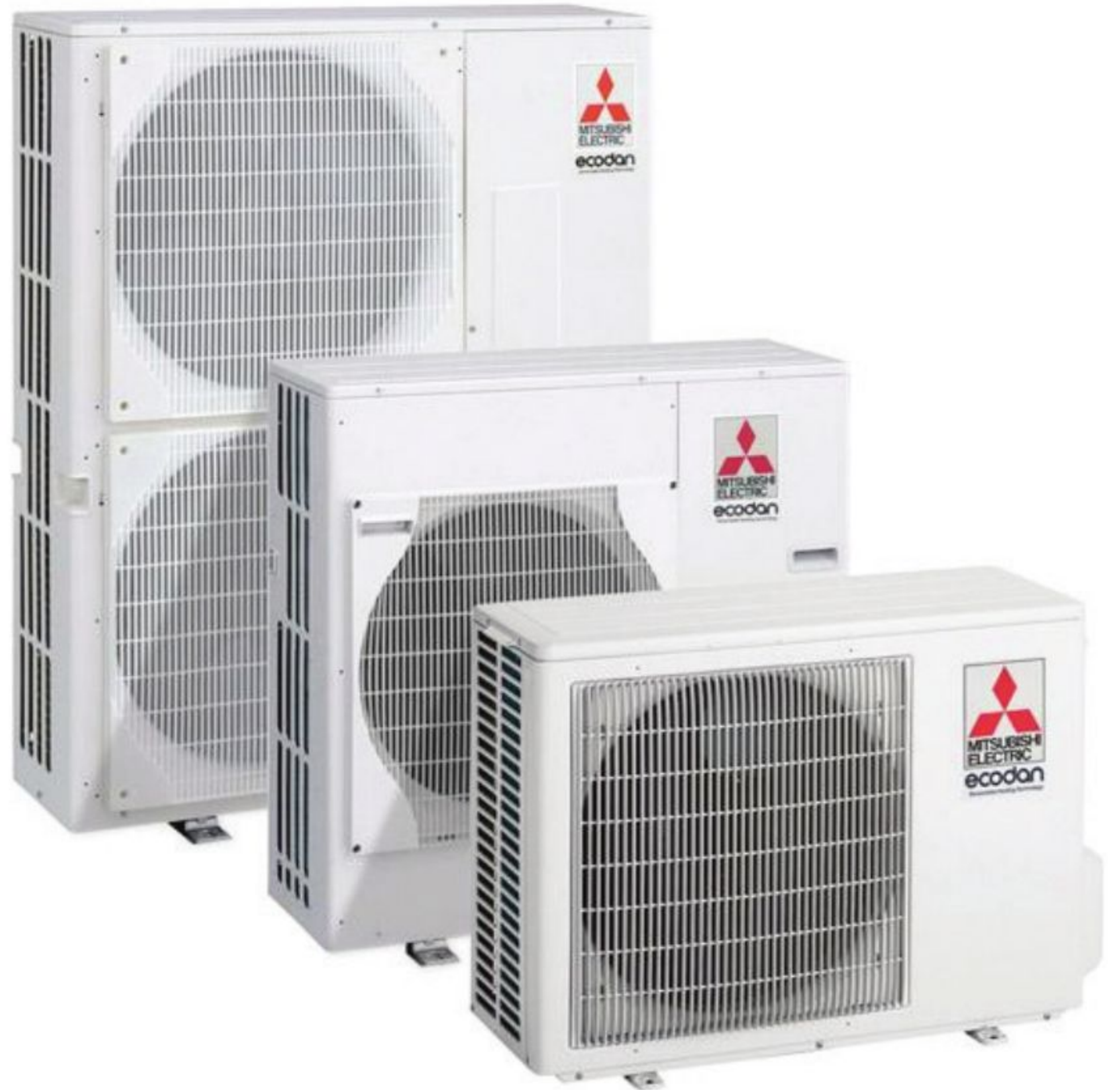
Above: Air-source heat pumps like these Ecodan units from Mitsubishi Electric typically have one fan on models from 4kW up to around 9kW and two fans on models up to around 16kW.
