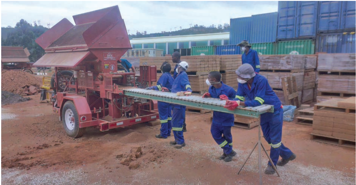
Construction takes place using bricks made via the compressed earth block method.
