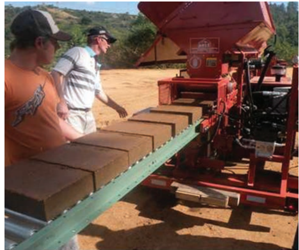
Construction takes place using bricks made via the compressed earth block method.
