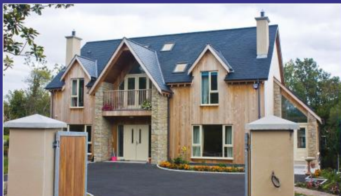
This is a low carbon home with an external wall U-Value of 0.13, built in Newcastle, Co. Down. The external facade has been finished in Cedar Cladding.
