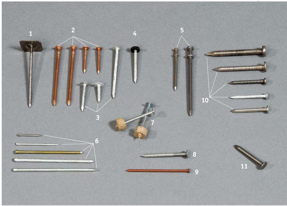
Specialty nails: 1. Simplex nail for roofing underlayment and thin foam insulation; 2. Copper flashing nails; 3. Galvanized roofing nails; 4. Gasketed nail for metal roofing and some skylight flashing; 5. Duplex nails; 6. Finish nails (the middle one is vinyl coated); 7. Furring nails for stucco wire; 8. Ring-shank nail; 9. Stainless-steel nail color matched to wood siding; 10. Joist-hanger nails (Teco nails); 11. Case-hardened masonry nail
