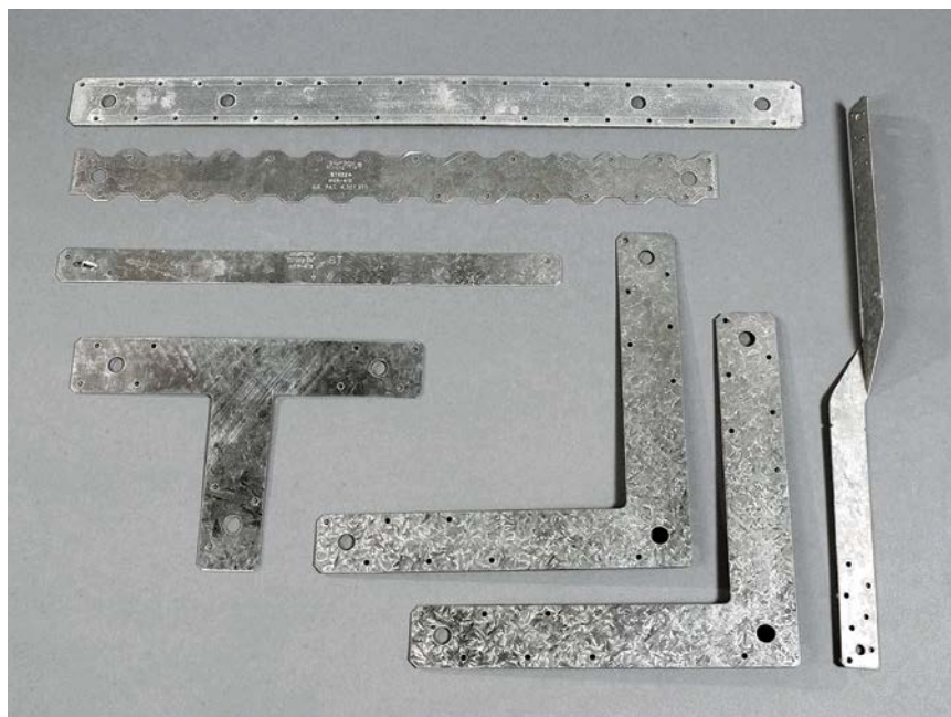
Straps, ties, and angles. Clockwise, from lower left: T-strap (post-to-beam connector), SST22 light-gauge strap, ST6224 (24-in.) strap, MST24 heavy-gauge strap, twist strap, and heavy-gauge L-straps.
