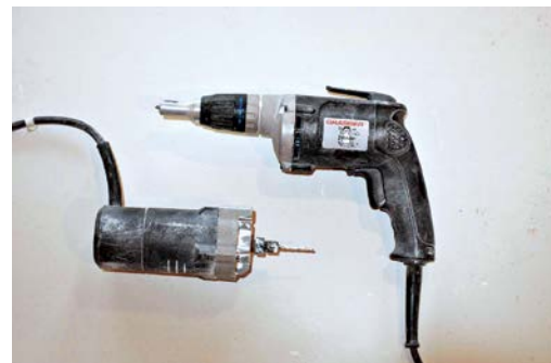
Drywall router (bottom) and screw gun.
