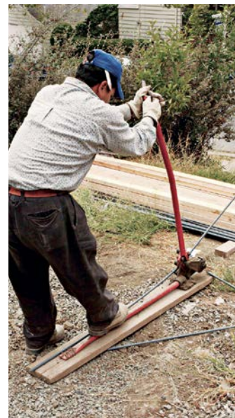
To use this rebar cutter-bender, you feed rebar parallel with the base arm for bending, as shown, and perpendicular to the base arm when cutting.
