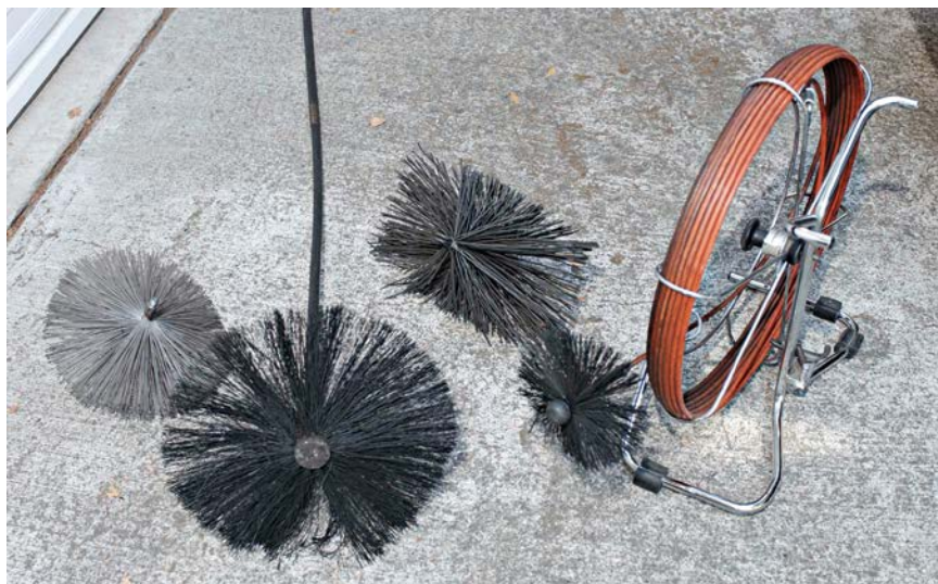
A professional chimney sweep needs a variety of brushes. The reel at right contains a 50-ft. flexible rod that can push and pull brushes.
