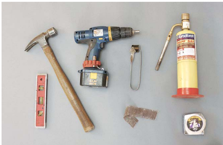
Miscellaneous tools. Clockwise, from left: torpedo level, hammer, 14.4v cordless drill, flint and steel striker (lights torch), gas soldering torch, tape measure, and plumber's sand cloth (used before fluxing pipe).
