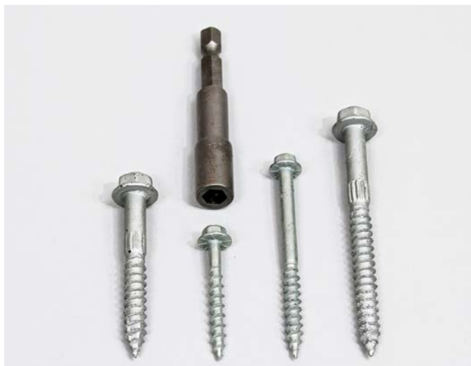
SDS and SD hex-head structural screws, whose shanks are sized to fit in the holes of various Simpson hardware. At top, a hex driver. The two outer screws are 1/4-in.-diameter SDS screws; the two inner screws are SD screws, typically used instead of Teco nails to attach joist hangers.
