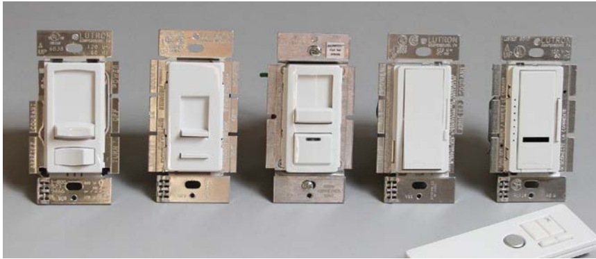
Slide dimmers. From left: Skylark Contour, Luméa, IllumaTech, Diva, Maestro IR (infrared) with remote control. All have a slide bar to preset light levels and a separate on-off switch. The bare-metal flanges around the dimmers are heat sinks.
