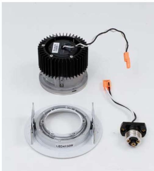
This simple kit can convert an incandescent ceiling fixture into an energy-saving LED fixture. Clockwise from lower right: a screw-in adaptor, cast-aluminum trim plate and lens, lamp housing, and heat sink.
