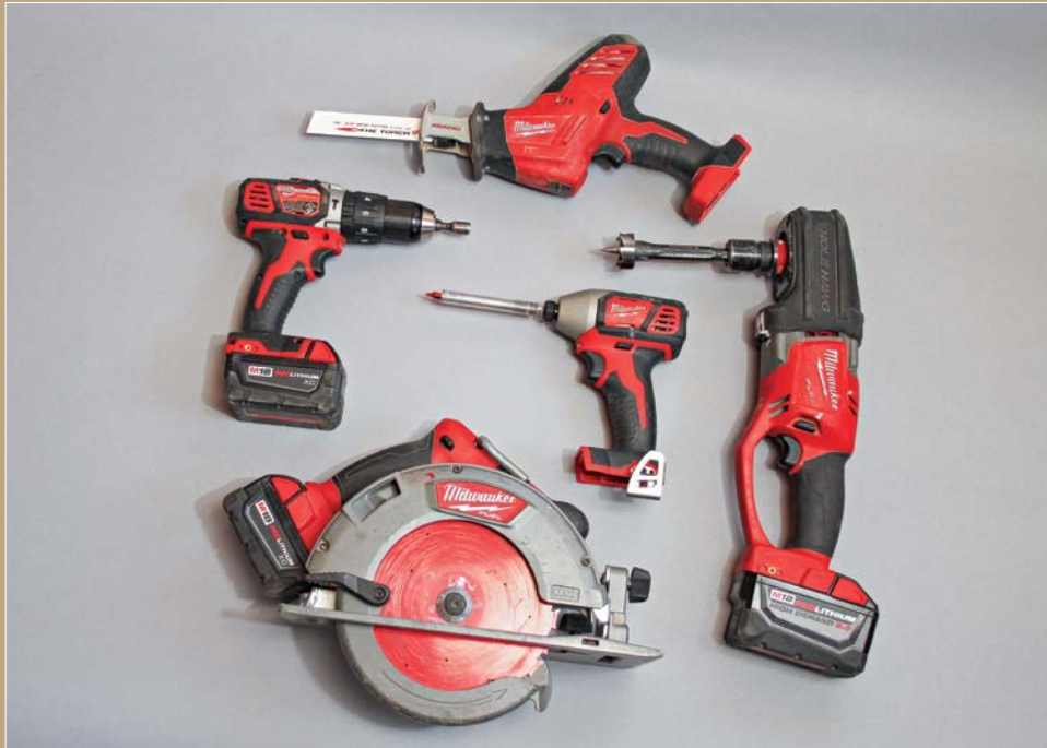
Milwaukee 18v cordless power tools. Clockwise from bottom: Circular saw, hammer drill, Hackzall reciprocating saw, HoleHawg right-angle drill, and impact driver.
