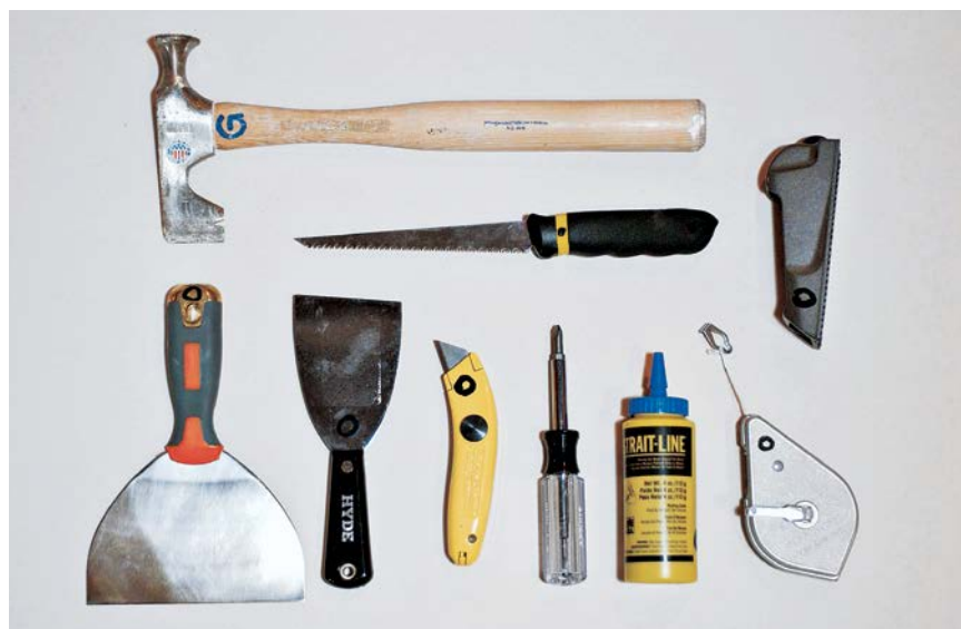
Basic drywall tools. Top: drywall hammer, utility saw, and rasp. Bottom, from left: 6-in. tapping knife, spackling knife, utility knife, multi-bit screwdriver, chalk, and chalkline box.
