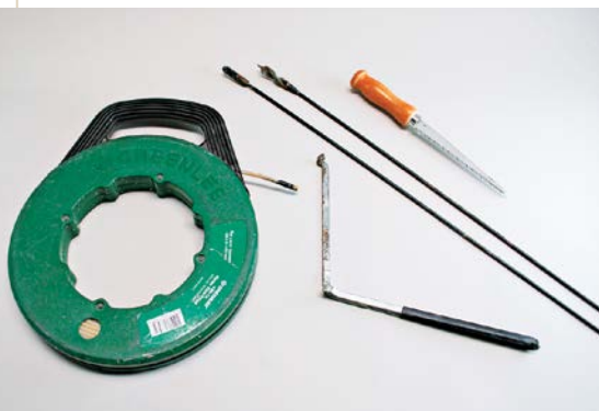
Remodel wiring tools. From right: drywall saw (sometimes called a stab saw), flex bit, bit extension, flex bit steering guide, and reel of fishing tape.
