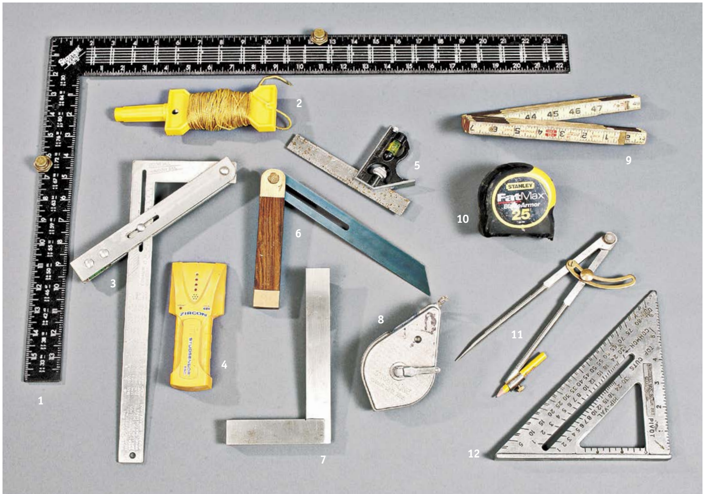
Measuring and layout tools: 1. Framing square; 2. String; 3. Adjustable square; 4. Stud finder; 5. Combination square; 6. Adjustable bevel; 7. Steel try square; 8. Chalkline; 9. Folding rule with sliding extension; 10. Tape measure; 11. Compass; 12. Swanson Speed Square
