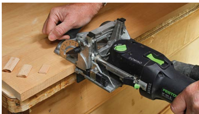
Domino biscuit joiner and biscuits. The fence on the front of the tool rests on the boards being slotted for glue and biscuits.
