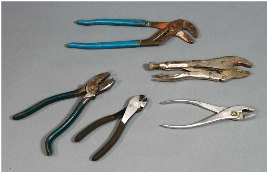
Pliers and cutters. Clockwise, from top: Channellock slip-joint pliers, Vise-Grip locking pliers, slip-joint pliers, side cutters, and lineman's pliers.
