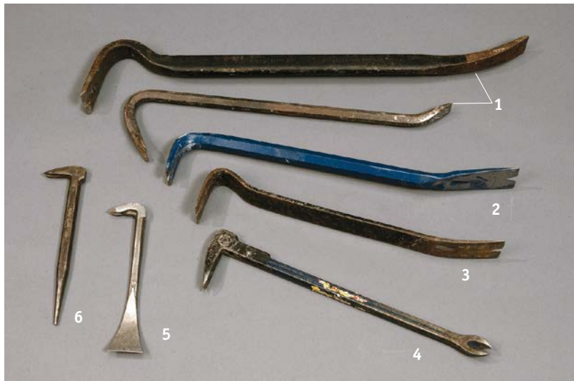
Wrecking and pry bars: 1. Crook-neck wrecking bars 2. L-bar 3. Flat bar 4. Cat's paw 5. 8-in. pry bar/nail puller 6. Cat's paw with punch point
