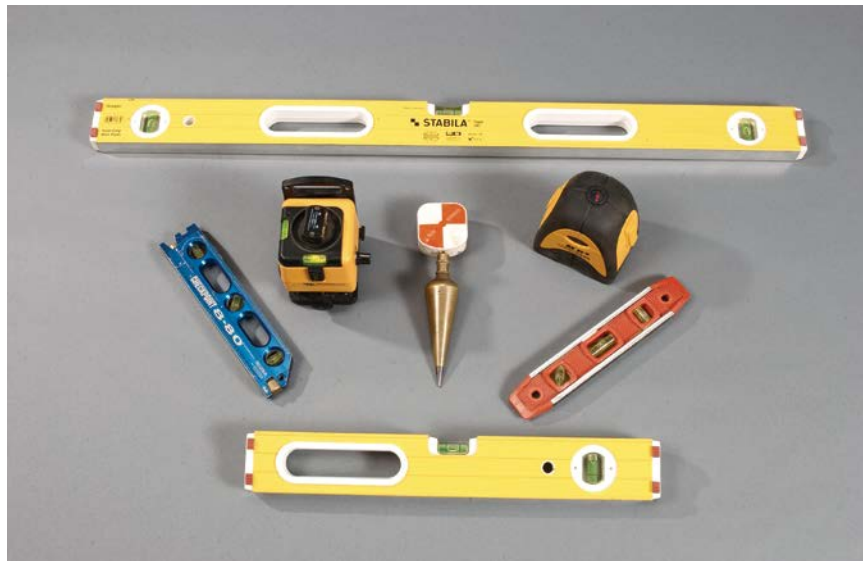
Levels and plumbing devices. Top: 4-ft. spirit level; center, from left: torpedo level with laser, rotating laser, plumb bob with Gammon Reel, five-beam self-leveling laser, and standard torpedo level; bottom: 2-ft. spirit level.
