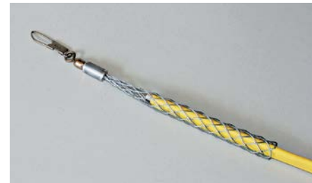
A swivel kelly grip slides over the end of the cable and prevents it from twisting as it's pulled.
