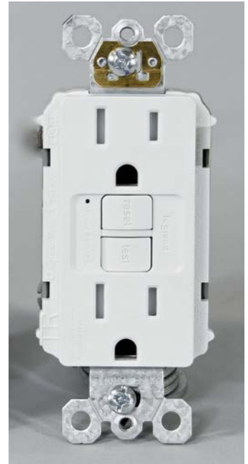
Ground-fault circuit interrupter (GFCI) receptacles detect minuscule current leaks and shut off power almost instantaneously. All bathrooms and kitchens must be GFCI protected, as well as outdoor outlets and garage outlets. Local codes may require additional GFCI protection.
