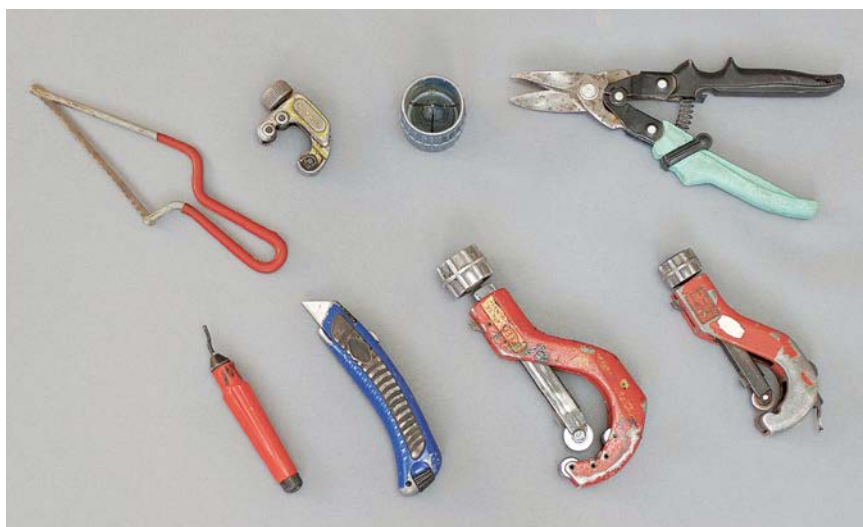
Cutting and reaming tools. Top row, from left: miniature hacksaw, close-quarters cutter, combo chamfer and reamer (cleans burrs from pipe ends after cutting), and aviation snips. Bottom row, from left: reamer, utility knife, large-wheeled tubing cutter (cuts up to 2-in. plastic pipe), and wheeled tubing cutter. The cutting wheels can be changed for different pipe materials.
