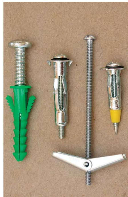
Use these anchors and bolts to attach light loads to drywall and plaster walls. From left: plastic anchor with screw, molly bolt, toggle bolt, and drive anchor.
