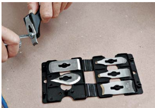
This hand scraper comes with six interchangeable stainless-steel blades, which will fit most contours you're likely to encounter.
