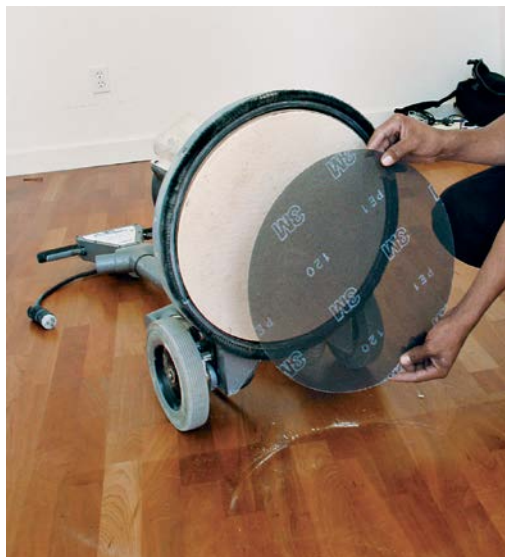
Buffer screens are held on with friction. Use them to fine-sand a floor that's been stripped or to sand between finish coats.
