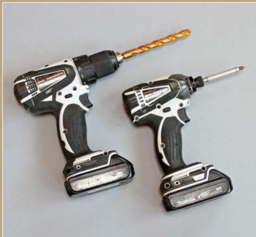
Impact drivers are beefy enough to drive bolts into masonry and compact enough to fit into tight spaces.
