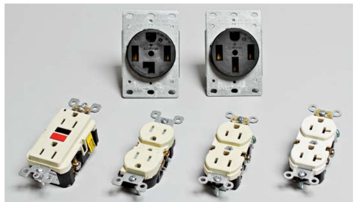
Receptacles for different loads. Clockwise from upper left: 30-amp dryer (125/250v), 50-amp range (125/250v), 20-amp duplex, 15-amp duplex, 15-amp tamper-resistant duplex, and 15-amp GFCI.
