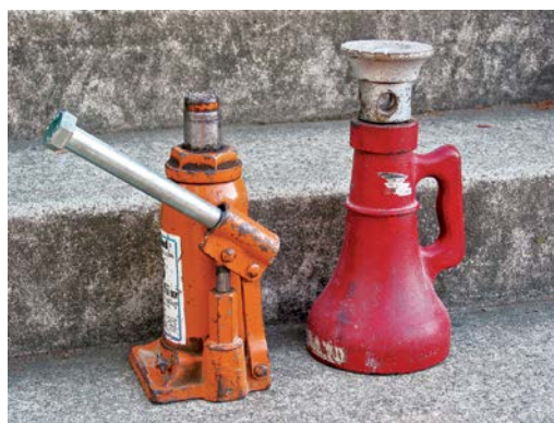
Jacks. Left: a hydraulic jack, the workhorse of house-raising. Right: a screw jack. Textured heads on both reduce chances of post slippage.
