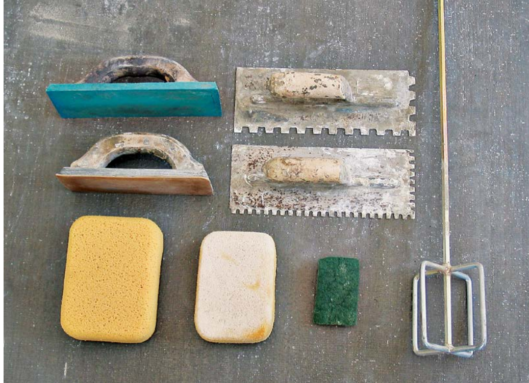
A small group of setting and grouting tools. Clockwise from upper left: grout floats, notched trowels, hand-drill mixing bit, and sponges (of which you'll need a variety).
