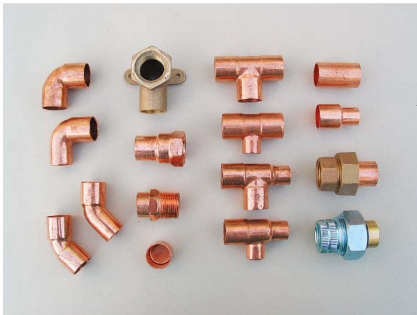
Water-supply fittings. First column, from top: \frac{3}{4} -in. 90, \frac{3}{4} -in. street 90, \frac{3}{4} -in. street 45, and \frac{3}{4} -in. 45. Second column, from top: \frac{3}{4} -in. CxF (copper-by-female) drop-ear 90, \frac{3}{4} -in. CxF adapter, \frac{3}{4} -in. CxM (copper-by-male) adapter, and \frac{3}{4} -in. cap. Third column, from top: \frac{3}{4} -in. tee, \frac{3}{4} -in. by \frac{1}{2} -in. tee, \frac{3}{4} -in. by \frac{1}{2} -in. by \frac{3}{4} -in. tee, and \frac{3}{4} -in. by \frac{1}{2} -in. by \frac{1}{2} -in. tee. Fourth column, from top: \frac{3}{4} -in. coupling, \frac{3}{4} -in. by \frac{1}{2} -in. reducing coupling, \frac{3}{4} -in. CxF union, and \frac{3}{4} -in. dielectric union.
