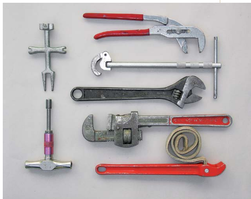
Jaws VII: wrenches and pliers. Clockwise, from upper left: tub-strainer wrench, slide-nut or sliding-jaw pliers, basin wrench, adjustable wrench, pipe wrench, strap wrench (won't mar polished pipe), and no-hub torque wrench.
