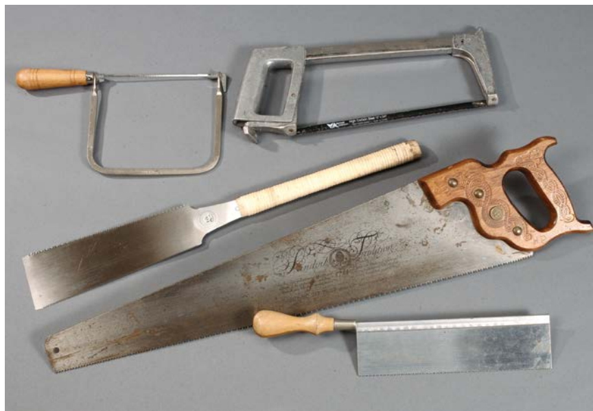
Handsaws. Clockwise, from lower right: dovetail saw, crosscut saw, Japanese saw, coping saw, and hacksaw.
