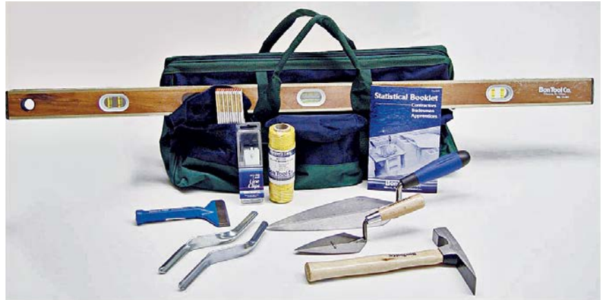
A bricklayer's tool kit (clockwise, from upper left): 4-ft. brass-bound level, tool bag, 6-ft. folding rule, statistical booklet (which covers estimating bricks and blocks, portland cement types, metric conversion, and a glossary of masonry terms), 11-in. steel trowel, 5½-in. pointing trowel, brick hammer, two convex jointers, 4-in. brick set, box of line clips, and yellow stringline.
