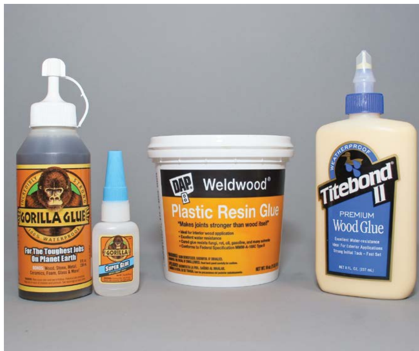
Four popular adhesives, followed by their chemical names. From left: Gorilla Glue (polyurethane), Gorilla Super Glue (cyanoacrylate), Weldwood plastic resin (urea formaldehyde), and Titebond II wood glue (polyvinyl acetate).
