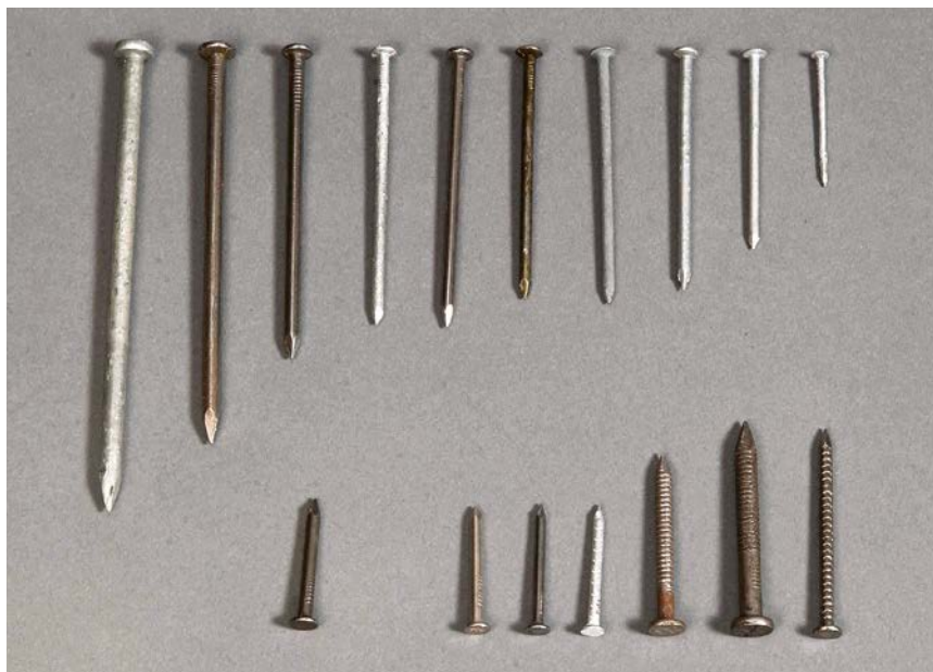
Nail types. Top row, from left: 60d galvanized spike, 40d common, 20d common, 16d galvanized, 16d common, 12d vinyl-coated sinker, 12d galvanized box, 10d galvanized common, 8d galvanized box, and 4d galvanized siding. Bottom row, from left: concrete nail and six joist-hanger and metal-connector nails (also called Teco nails). Longer nails may be required when sheathing covers framing.
