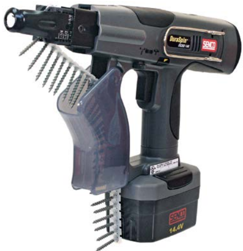
This Senco DuraSpin 14.4v driver employs a clutch to prevent overdriving screws, as well as a collated strip of fasteners that frees up one hand to hold a drywall panel in place.
