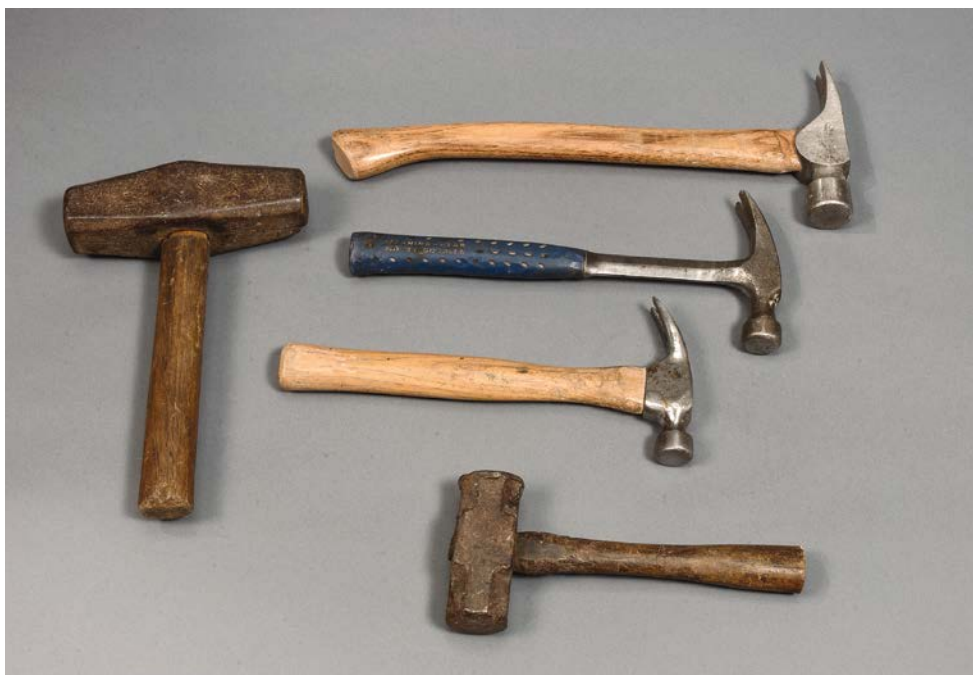
Hammers. Left: hand sledge; top to bottom: 26-oz. framing hammer, 20-oz. framing hammer, 16-oz. finish hammer, and small hand sledge.
