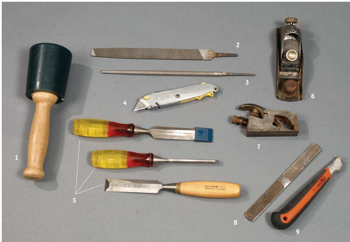
Cutting and shaping tools: 1. Mallet; 2. Flat file; 3. Rat-tail file; 4. Utility knife; 5. Chisels; 6. Block plane; 7. Bullnose plane; 8. 4-in-1 rasp; 9. Carbide scraper
