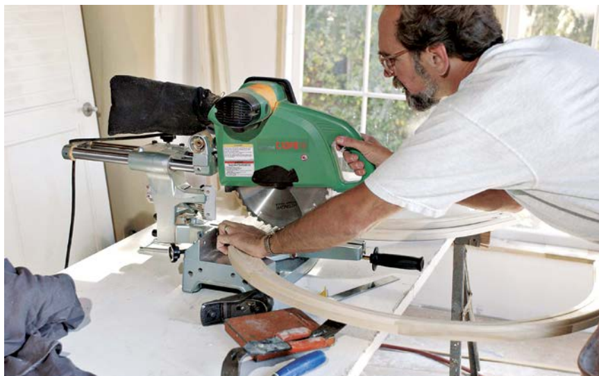
A power miter saw is a must if you're installing a houseful of trim. The 10-in. sliding compound miter saw shown is big enough to make complicated beveled miter cuts in large crown molding.
