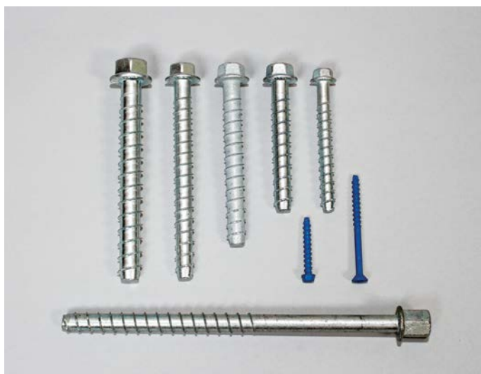
An assortment of concrete anchors, which are specialized screws that attach wood to concrete. The larger ones are Titen bolts, which can be used when anchor bolts are not required, such as when attaching the sills of non-load-bearing interior walls to concrete. The huge bolt at the bottom of the photo is a 3/4-in. specialty hanger bolt, which has a threaded hole in its oversize nut.
