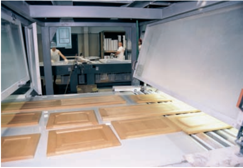
Quality control of cabinet doors on the KraftMaid assembly line.
