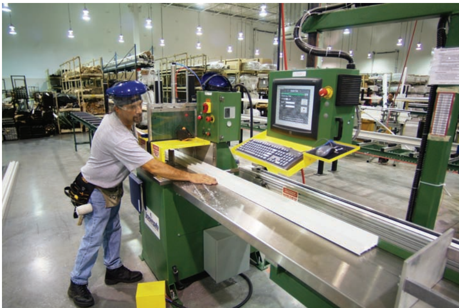
Vinyl is cut in sections for the creation of windows (Simonton Windows).
