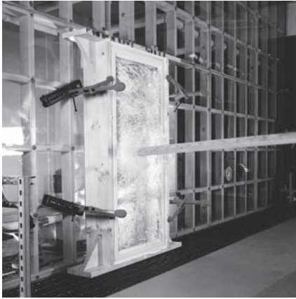
Windows are tested at a lab to see if they will withstand hurricane-driven projectiles (Photo courtesy of Simonton).
