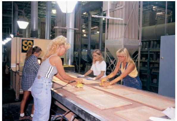
Cabinet doors are sanded on an assembly line in a KraftMaid plant in Ohio (Photo courtesy of KraftMaid).
