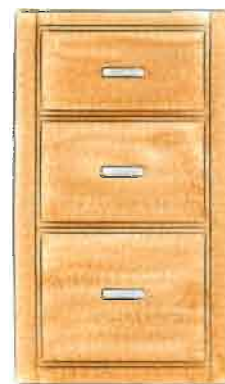
Graduated-size drawers with beaded edges, inset in face-frame, but without intermediate rails
