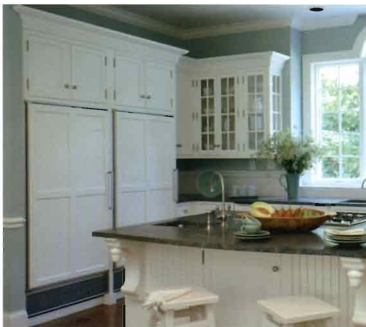
▲ THIS HIGH-EFFICIENCY REFRIGERATOR (SUNFROST) IS FINISHED with a copper veneer that has been given a patina with heat and chemicals. Handles are turned walnut. Countertops are solid surface and stainless steel.
