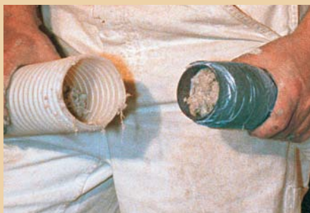
Clogs occur where hoses reduce in size. To clear the blockage, disassemble the joint.
