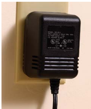
This wall cube draws power even when nothing is plugged into it.
