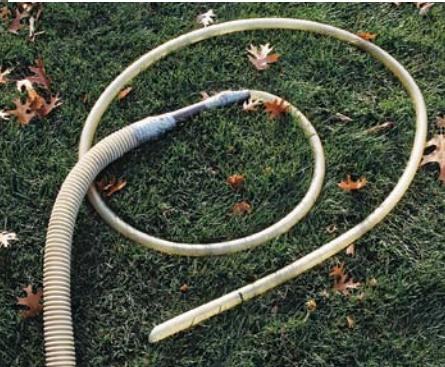
A 1¼-in.-dia. vinyl fill tube attached to the end of a larger-diameter hose makes it easy to snake into confined spaces for dense-packing cellulose. The marker line near the end warns you that the end is near as you pull the tube out.
