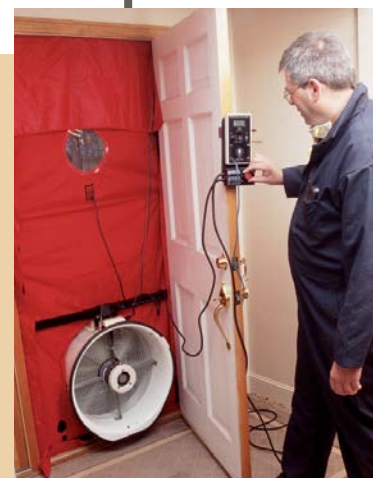
A blower door is used to measure how airtight a house is. It's also useful in helping identify where the air leaks are.
