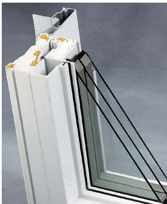
This fiberglass frame conducts much less heat than vinyl and wooden frames do, and it is more dimensionally stable, too. This Canadian-made sample has a third layer of glass, instead of plastic film.
