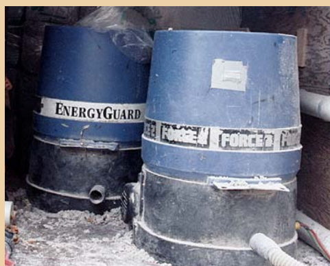
This medium-size cellulose blower is typical of the type of machine that you might rent or borrow from an insulation supplier.
