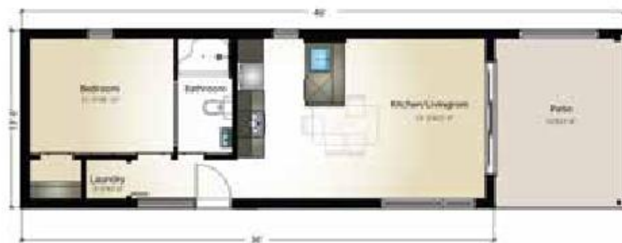
Certified in accordance with CSA A277, Guildcrest Homes' Eldorado complies with the Ontario Building Code for year-round occupancy. Set on a permanent foundation, it has a gross area of 486 sq. ft.; 621 sq. ft. including patio.
