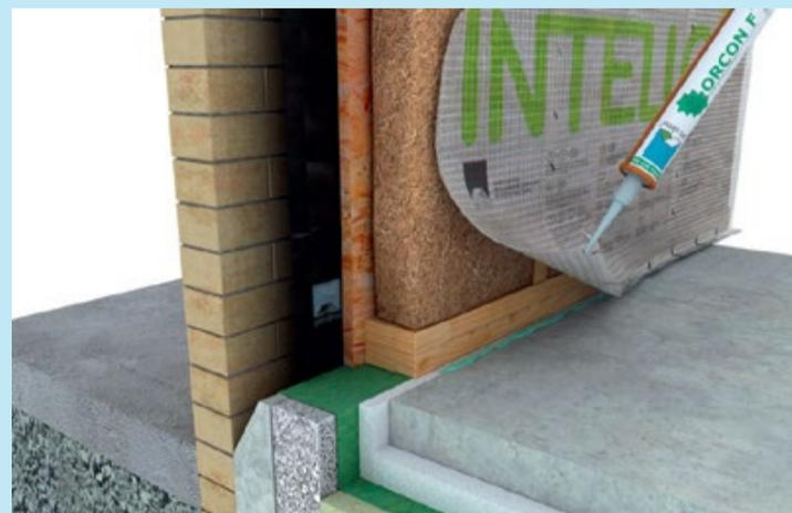
Bonding airtight vapour control layers to other building materials for an airtight finish requires an adhesive which boasts high adhesion but is also flexible and elastic. One such product is the Pro Clima Orcon F.
