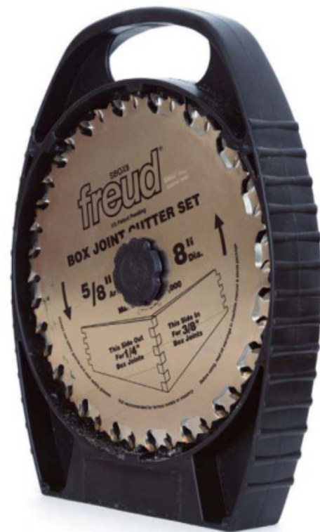
At the ready. A case with a threaded knob secures and protects the two cutters. The set makes perfect 1/4-in. and 3/8-in. grooves and box joints.
