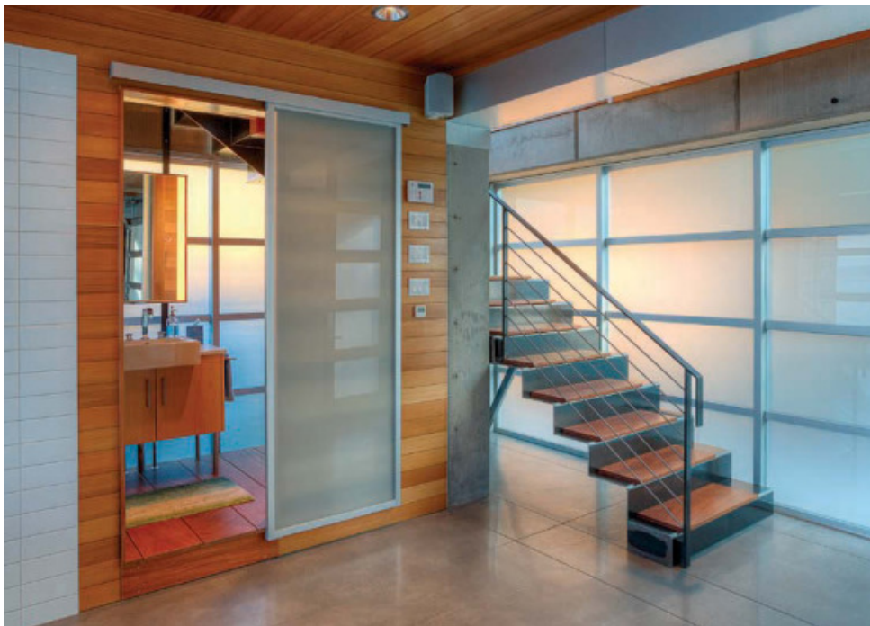
WEATHERPROOFED The main floors are connected by a steel-plate stair with sapele-wood treads. All electrical recepticals, switches, and controls are located high up on the walls in case of flooding.
