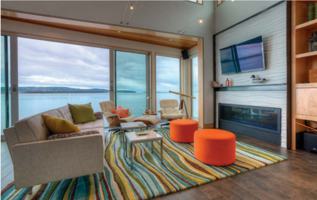
AT ONE WITH THE WATER The living room is lined with 85-mph impact-rated aluminum-clad windows with insulated glass, yielding 180° views of Skagit Bay. The prow sitting area is meant to give the sense of being on a boat; the wave-patterned Modular Arts wall panels fit the ocean theme.
