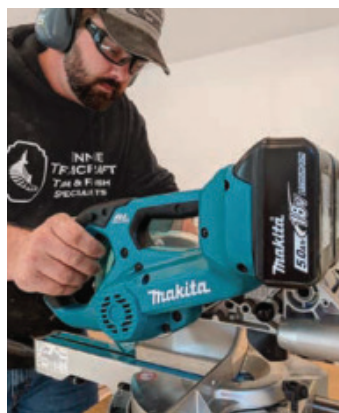
Small yet powerful. Weighing less than 30 lb. (including its two 18v batteries), the Makita XSL02Z can crosscut a 2x12 at 90°.
