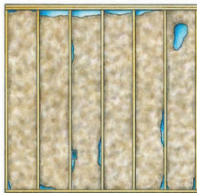
Grade II: Up to 2% missing insulation
