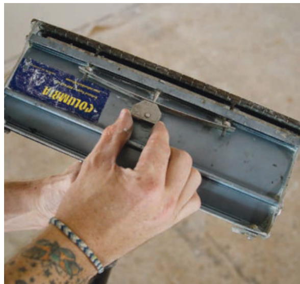
Adjust the flow. The eccentric cam adjusts the flow, so you can determine the amount of compound to dispense. The idea is to fully coat the seam without excess and leave a smooth finish free of voids as you go.
