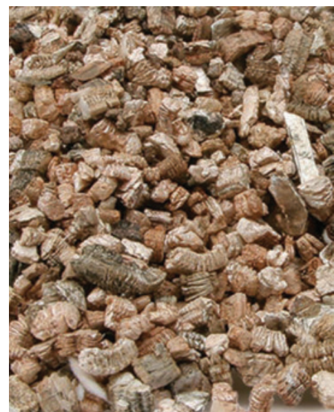
Vermiculite is a mined mineral that was used as building insulation for decades. It frequently contains asbestos and is costly to remediate.
