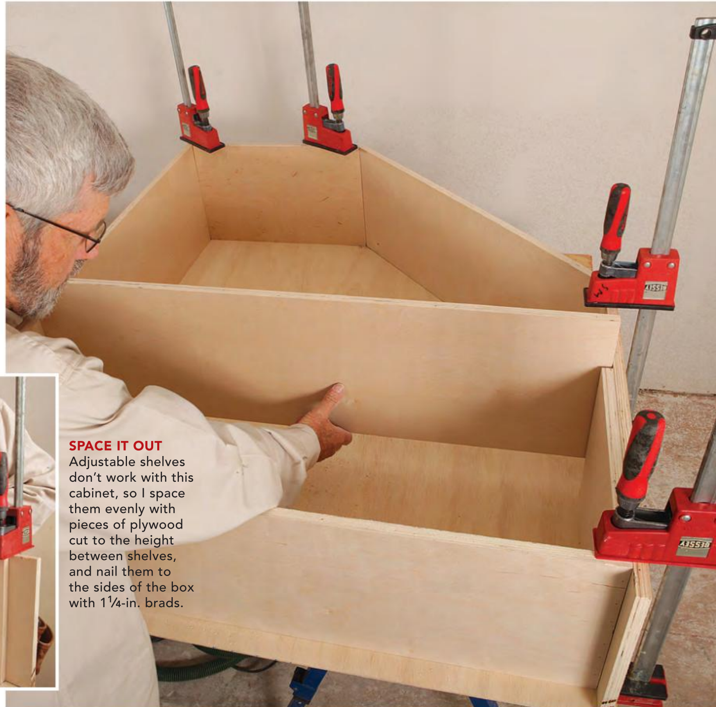
FASTEN AS YOU GO Fasten parts as they're cut for a tight fit, for accurate marks, and to ensure nothing gets mixed up.
