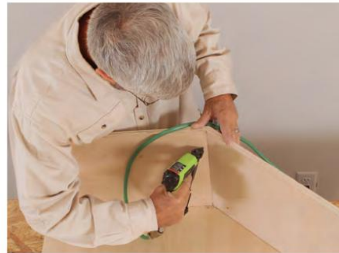
FASTEN AS YOU GO Fasten parts as they're cut for a tight fit, for accurate marks, and to ensure nothing gets mixed up.
