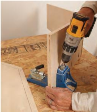
PREP THE POCKETS Pocket-hole screws secure the face frame along the sides that butt into the wall and ceiling. Drill the pocket holes before the entire perimeter of the cabinet is fastened to make things easier.
