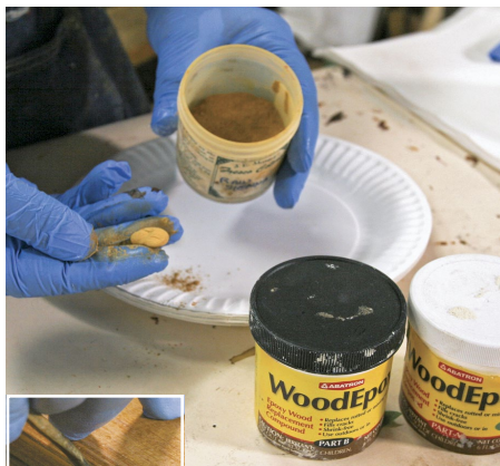
Epoxy for the holes. A two-part epoxy filler mixed with dry pigment creates a tinted filler that's easy to pack into nail holes or blemishes.
