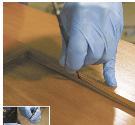
Sealer makes life easy. Because the glaze is sealed, excess filler can be wiped away easily, and glaze can be dabbed on to match the rest of the finish.
