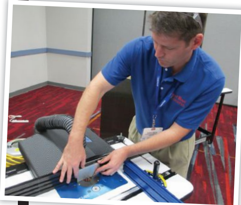
At AWFS, NextWave previewed its digitally controlled undermount router table, due out soon. The router follows a programmed path.
