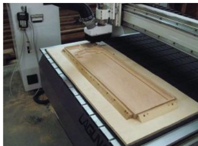
Step 3: Oak panel locked in place the Laguna Swift CNC (detail on facing page.)
