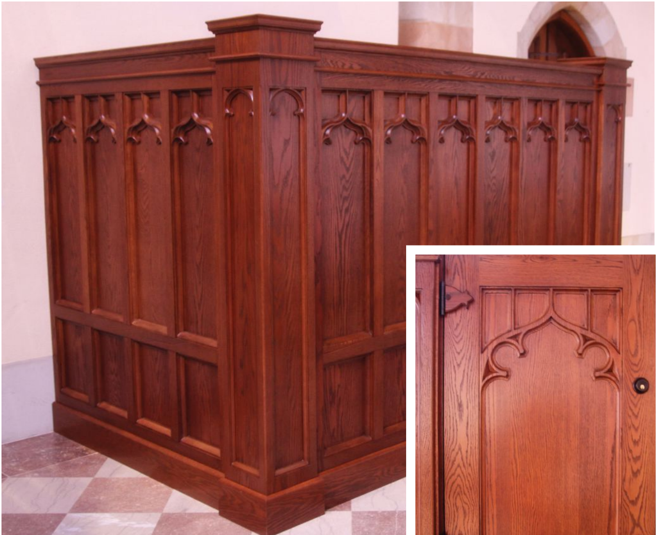
To match a new electronics control booth (above and facing page) to its century-old landmark setting, Lutes copied detail from original woodwork (right) and matched it using Aspire software and his Laguna CNC.
