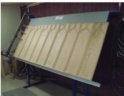
Step 4: Unfinished panels are glued to form the wall of the control booth.
