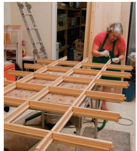
Counter clockwise from top: Completed windows weighed 700 pounds, challenging for transport and installation; the jig makes a concave cope cut on the end of the muntin bar where it meets the convex part of the inner arch; vertical muntins being notched, on a Laguna CNC; a concave cope cut lets the muntin meet the arch; gluing the lattice; profiling the convex side of the inner arch.
