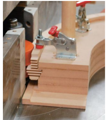
Counter clockwise from top: Completed windows weighed 700 pounds, challenging for transport and installation; the jig makes a concave cope cut on the end of the muntin bar where it meets the convex part of the inner arch; vertical muntins being notched, on a Laguna CNC; a concave cope cut lets the muntin meet the arch; gluing the lattice; profiling the convex side of the inner arch.
