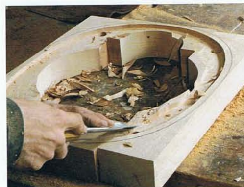
THIS GOUGE IS GOOD. To hog away stock the router couldn't reach, the author used a gouge.
