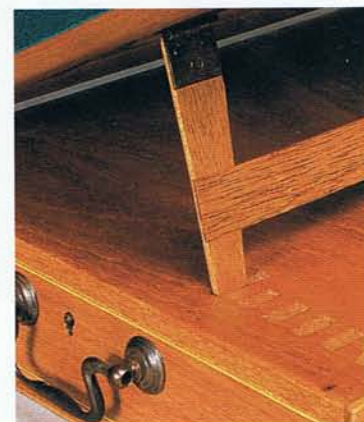
A STAND THAT FOLDS AWAY. The top of the desk is mortised to accept the support stand, which is hinged to the lower writing surface.
