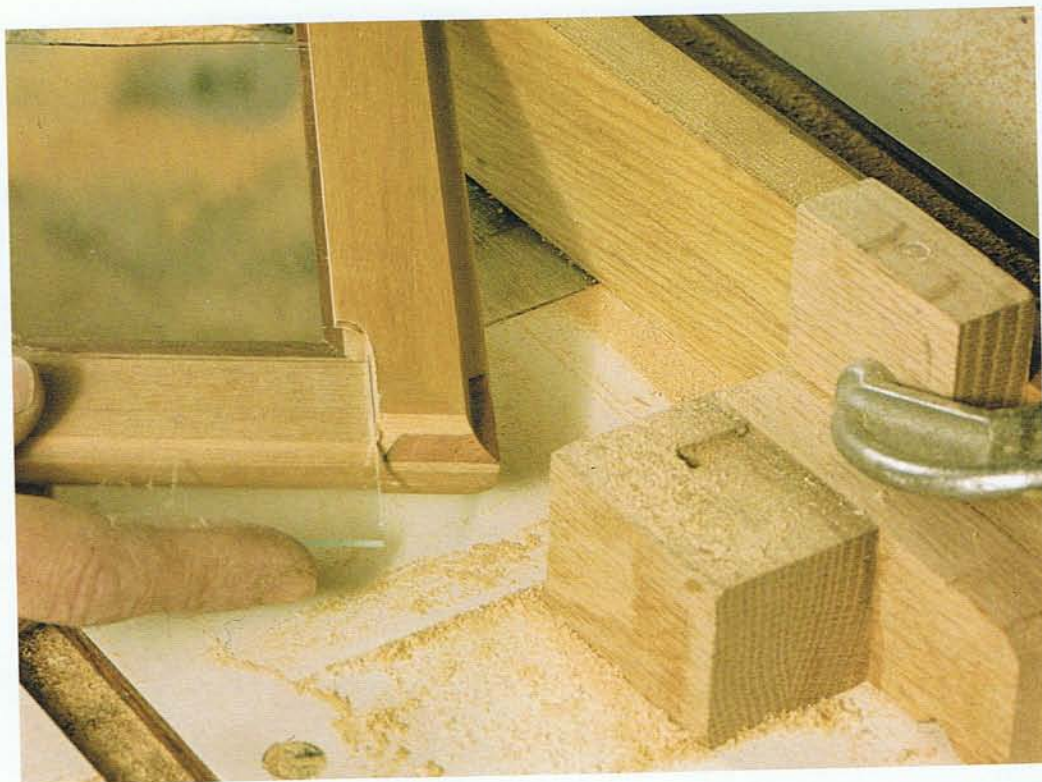
ACCESS SLOT. After routing a picture-entry slot by sliding this frame between two stop blocks on his router table, Segal checks the fit of the glass. The frame back was coved to show more of the spline.
