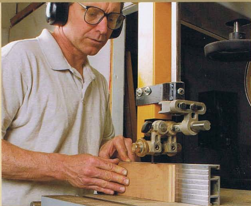
Sides resawn from thick stock on the bandsaw will produce a box with four matching corners.
