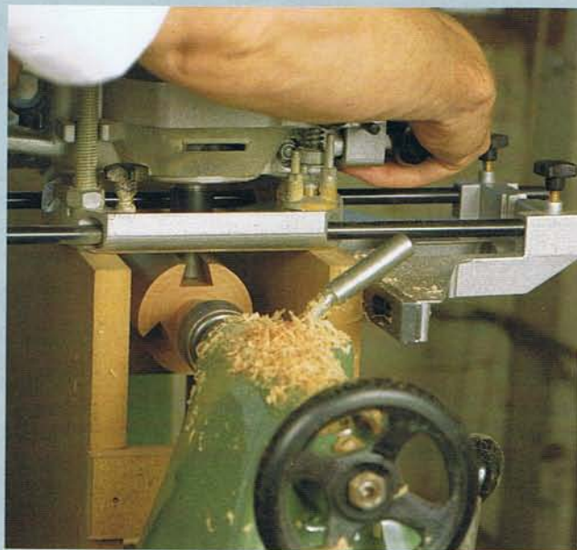
TO CUT THE DOVETAIL SOCKETS, the router rides on top of the jig, with an edge guide positioned to center the bit on the table post. The author first hogs out most of the socket waste with a straight bit and finally cuts the socket in one pass with a dovetail bit.
