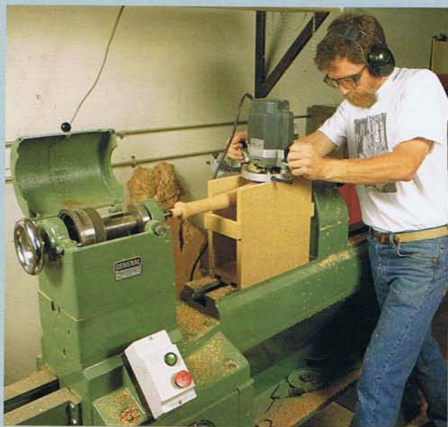
CUTTING SLIDING DOVETAIL SOCKETS IS A SIMPLE TASK WITH THIS LATHE-MOUNTED JIG. The jig must be square, accurate, and parallel to the axis of the lathe for proper attachment of the legs. The stability of medium-density fiberboard makes it a good choice for jigs.
