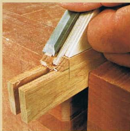
A MITERED DOOR JOINT. With a 45° miter jig clamped to the rail, a chisel pares to the line. This simple detail lends a framed and finished look to the door.
