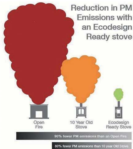
Above: This illustration, provided by the Stove Industry Alliance (SIA), outlines the difference in harmful PM emissions between Ecodesign Ready Stoves and other, less efficient alternatives
