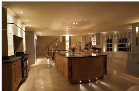
Above: For this scheme, Brilliant Lighting ( www.brilliantlighting.co.uk ) incorporated powerful downlighters that deliver shadow-free task illumination for the central island unit. Accent fittings built into the kickers and window sill add interest and texture, while the pillar-mounted units throw light in both directions and wash the ceiling with brightness to help lift the space
