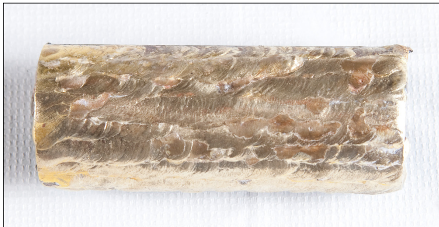
FIGURE 13-3: An example of a brazed corncob.
