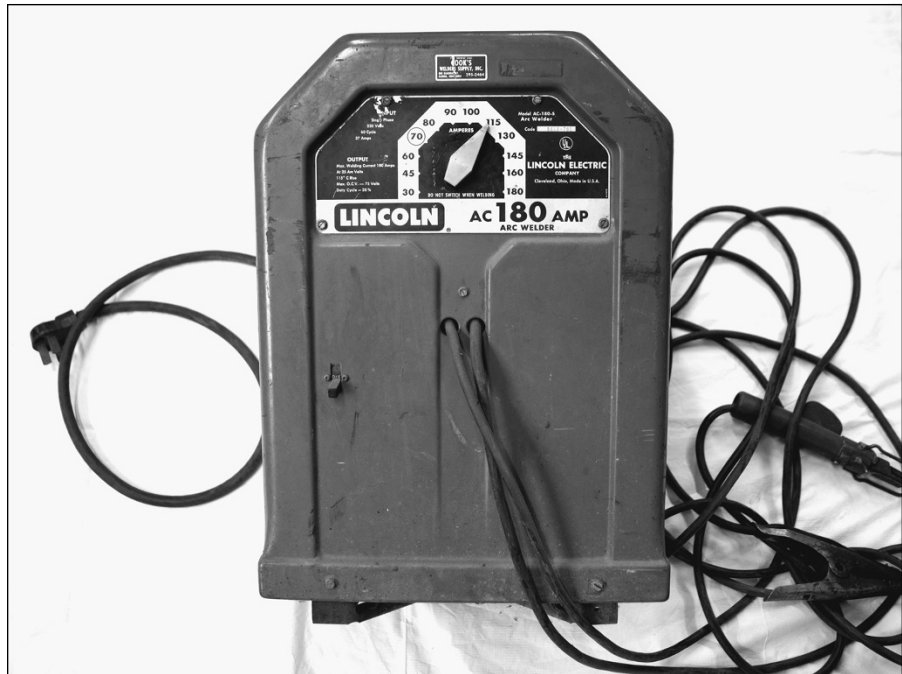
FIGURE 5-2: Transformer buzz box.
