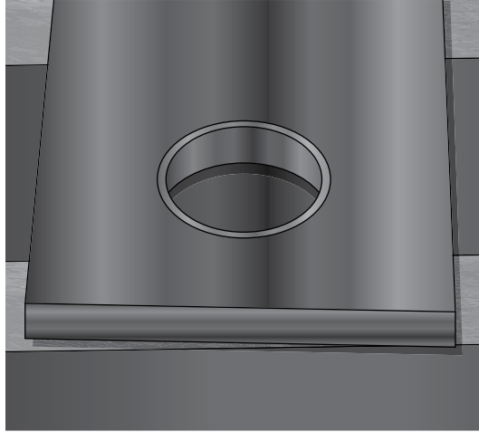
FIGURE 12-2: Perfect circle cut in aluminum.
