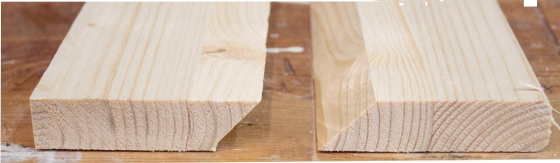
A photograph showing two pieces of light-colored wood on a wooden workbench. The piece on the left has a 45-degree bevel cut on its top edge. The piece on the right has a 90-degree cut on its top edge. Both pieces are oriented vertically, showing their grain and the precision of the cuts.
