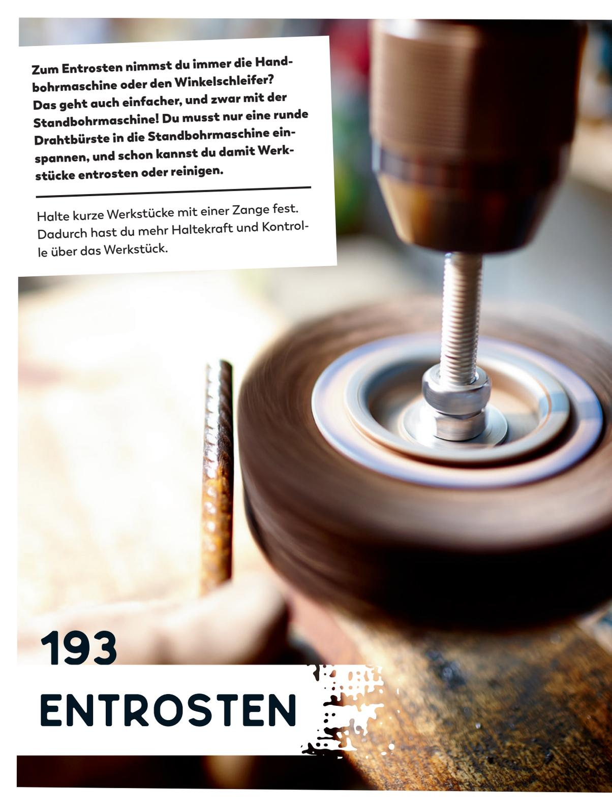
A close-up photograph showing a wire brush being used to clean a metal workpiece. The brush is mounted on a drill bit and is spinning, creating a blurred motion effect. The workpiece is held in a vise, and the background is softly blurred, focusing attention on the cleaning process.
