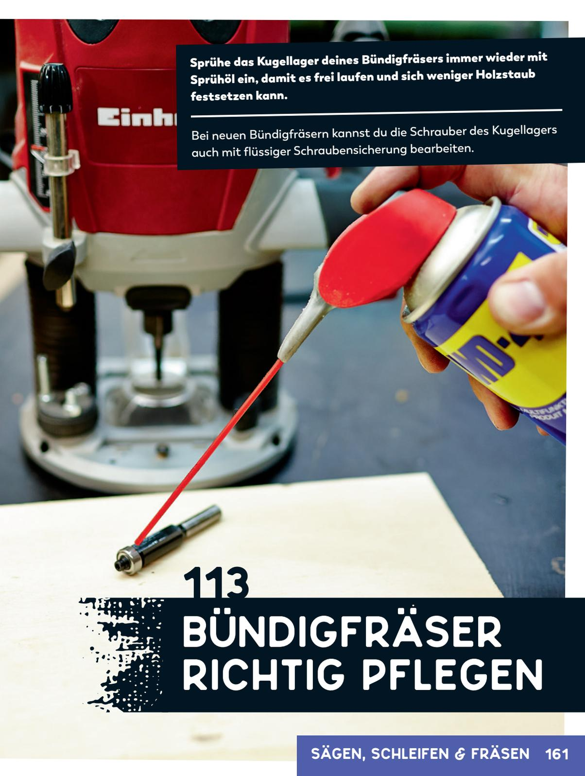
A close-up photograph of a red Einhell router. A hand is holding a blue and yellow spray can with a red nozzle, applying a red spray to the ball bearing of the router's spindle. The router is positioned on a light-colored wooden surface. The background is slightly blurred, showing a dark workbench.
