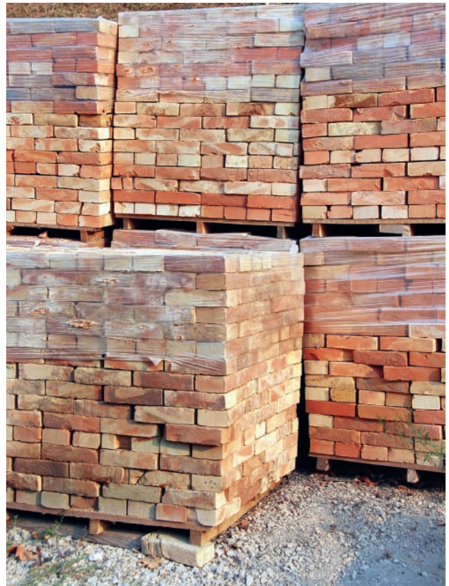
▲ Figure 4.11 Bricks protected by polythene sheeting
