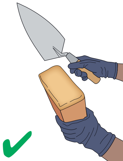
▲ Figure 5.40 Bricklayer correctly making a full perp joint
