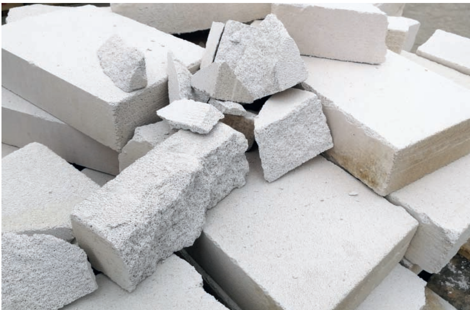
▲ Figure 3.10 Check the suitability of materials before you use them; these lightweight thermal blocks have been damaged by careless handling
