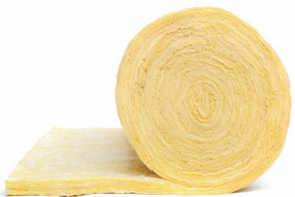
▲ Figure 1.20 Fibreglass insulation can be manufactured from recycled glass
