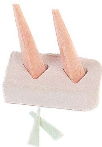
The senior cone sits in a clay cone sitter, while the junior cone will be placed in the kiln's cone sitter.
