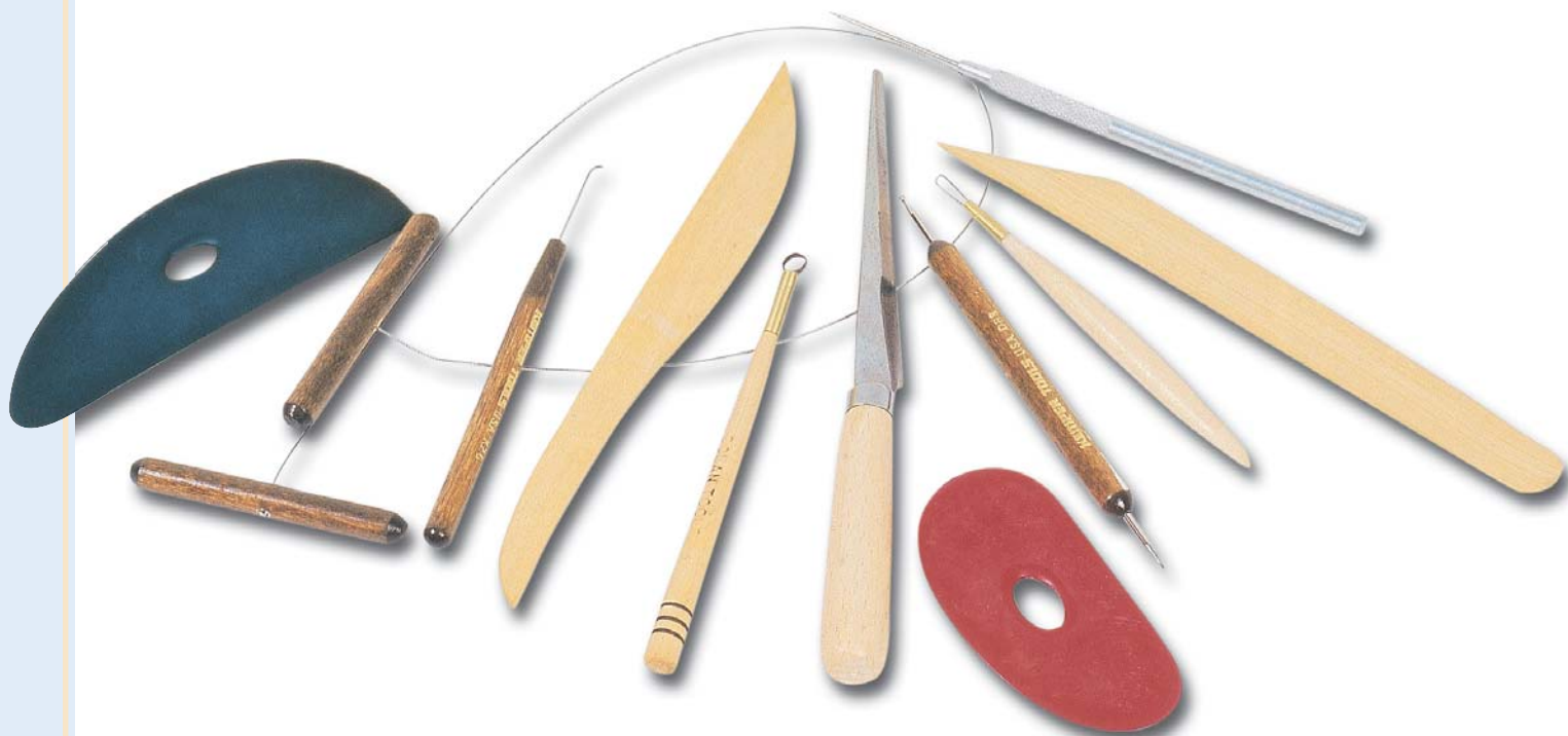
Common ceramic tools can be used to create tile. Left to right: small sponge, flexible rib, cutting wire, finger tool, wood modeling tool, wire end tool, potter's knife, flexible rib, stylus, wire/wood modeling tool, wood modeling tool, metal potter's needle.
