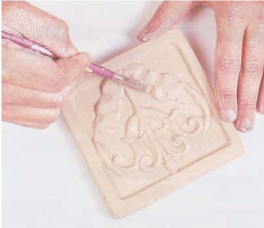
9. Use a short bristled brush to clean off the tool marks and to smooth out any edges. Brushes make excellent tools when carving tile. I switched back and forth between my tools and the brush, until the tile became smooth, and the detail refined.
