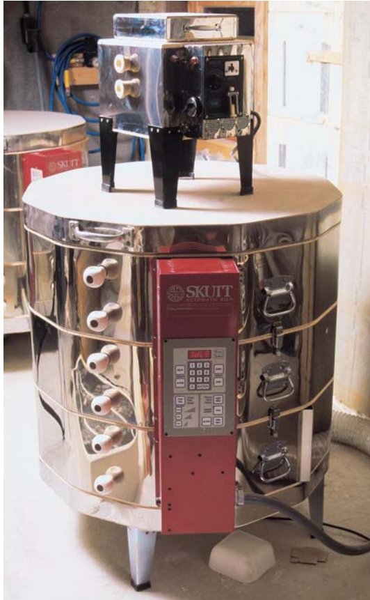
A large electric kiln, which can produce hundreds of tiles with each firing and a small test kiln with a chamber that can accommodate two to three tiles at a time.
