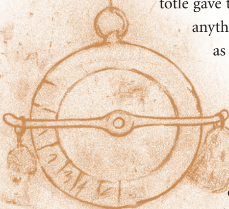
Sketch of hygrometer designed by Leonardo.
