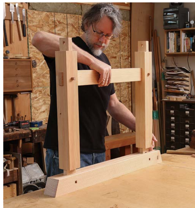
Assemble in stages. Cullum first drives the pins connecting the stretcher to the posts (top), then fits the posts into the beam (above).
