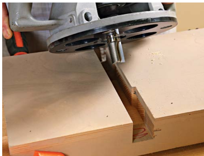
Rout the final shape. A template ensures that all of the dog holes are identical. Because the dog holes in the vise jaw face the opposite direction from those in the benchtop, Gochnour uses a template that has a pattern for both directions (top). The pattern has a notch so that a flush-trimming bit creates the pocket into which the dog's head fits (above).
