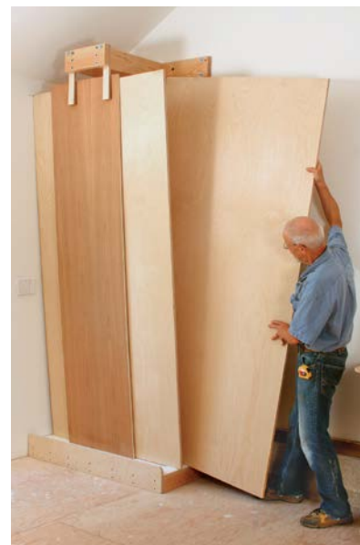
Take your pick. The restraining bars let you leaf through the stack to find a sheet and remove it easily without removing others.
