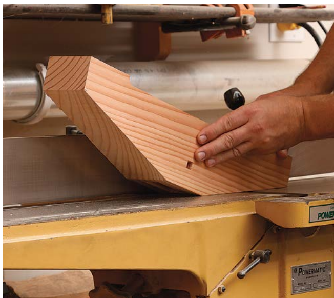
Quick slant. Cutting close to his layout lines, Cullum bandsaws the foot's diagonals (top), then smooths out the sawcut with a few passes on the jointer (above).
