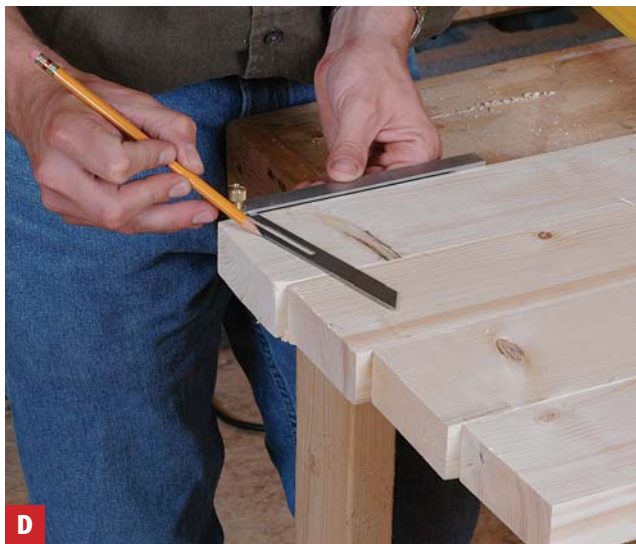
D Mark out the angle Clamp the legs together and transfer the angle from the bevel gauge.
