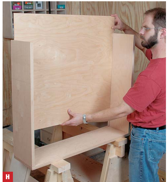
H Insert the back Add just a few drops of glue into each of the grooves.
