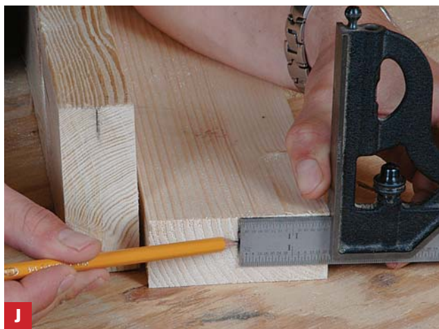
Mark out the centers Use a combination square to find the center of the top and the subtop.
