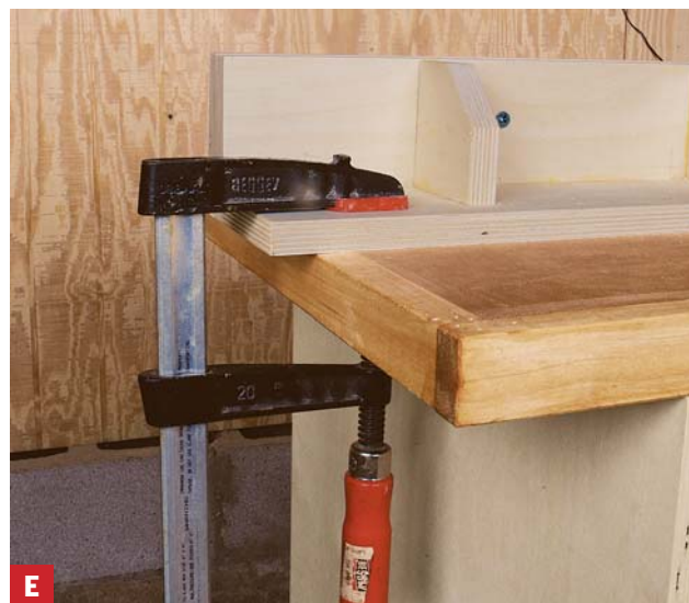
You're ready to rout To put the fence to use, just clamp it in place on the top of the router table.
