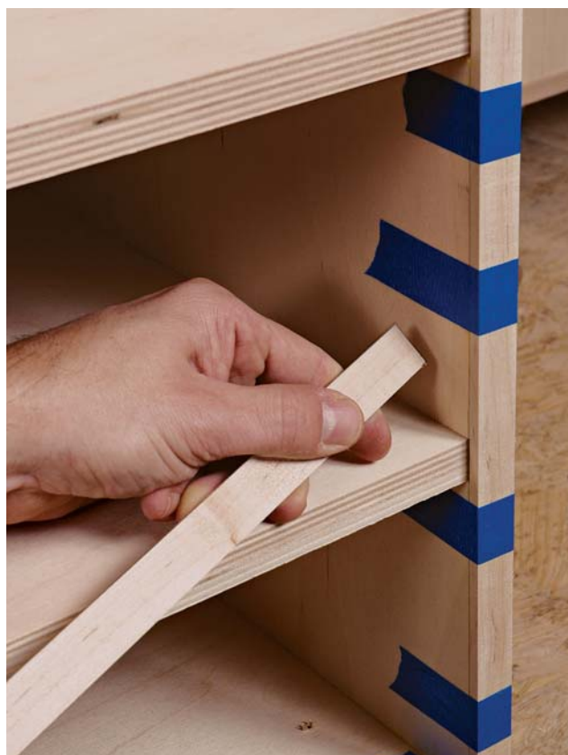
Trim plywood The raw edges of plywood can be trimmed with hardwood strips to disguise plywood as hardwood.
