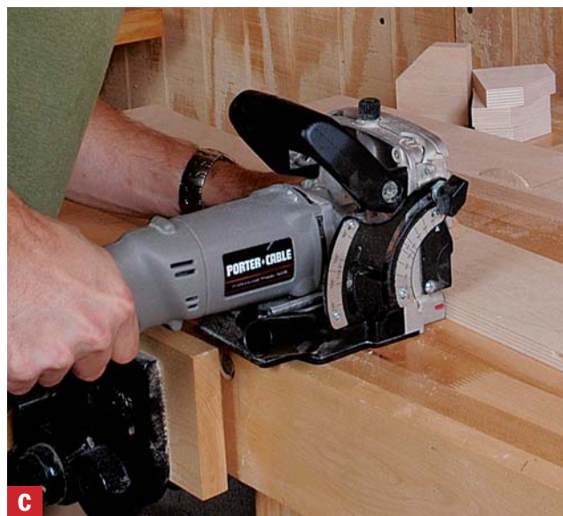
Biscuit the fence Mark and cut mating biscuit slots on the base of the fence.
