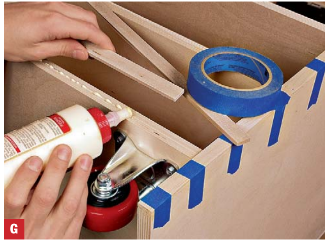
Give it a finished look A thin bead of glue and painter's tape offer plenty of holding power to attach a hardwood edging.
