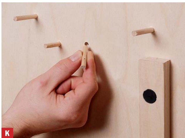
Use pegs to hold tools Lengths of ¼" dowels are glued and hammered into place.
