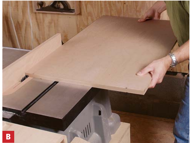
A rabbet is a dado at the edge A rabbet is nothing more than a dado cut along the edge of a board. Keep the stock flat on the tablesaw table to ensure a cut of consistent depth.
