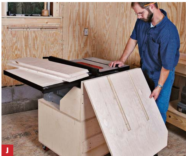
Fold the table down When not in use, remove the braces to fold the table down and out of the way.
