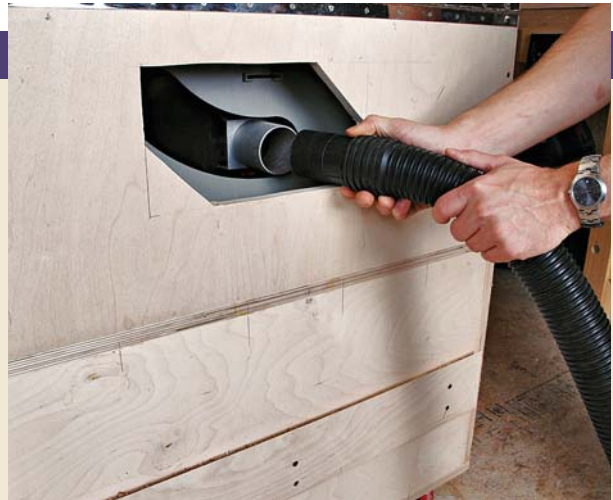
Attach the vacuum On the saw used for this station, the vacuum hose attaches to the saw's dust chute through the cutout in the rear support.
