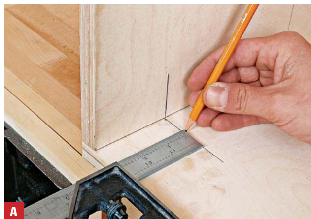
Lay out the biscuit slots With the case parts set in place, use a combination square to mark out the centerlines for the biscuit slots.
