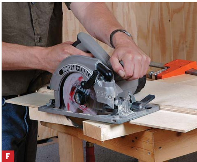
F Cut the angled ends Using a circular saw guide guarantees a straight cut. After cutting, leave the legs clamped together and repeat the same process on the other end.
