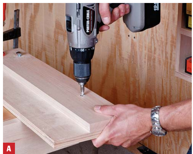
A Drill the stop and skirt Before attaching the end skirt to the left end of the vise, drill holes through both the skirt and the end stop.
