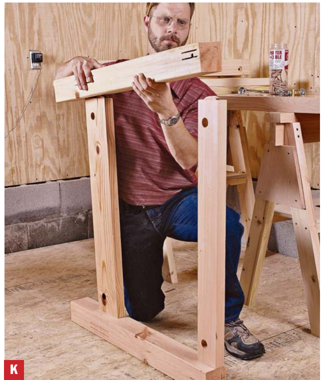
Assemble the front and back Before adding any glue, set the biscuits in place and assemble all the parts one side at a time.
