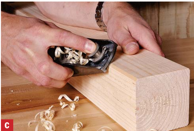
C Chamfer the hard edges To soften those bumps against the bench, ease the corners—of the legs and all other exposed edges—by knocking off the hard edge with a block plane.
