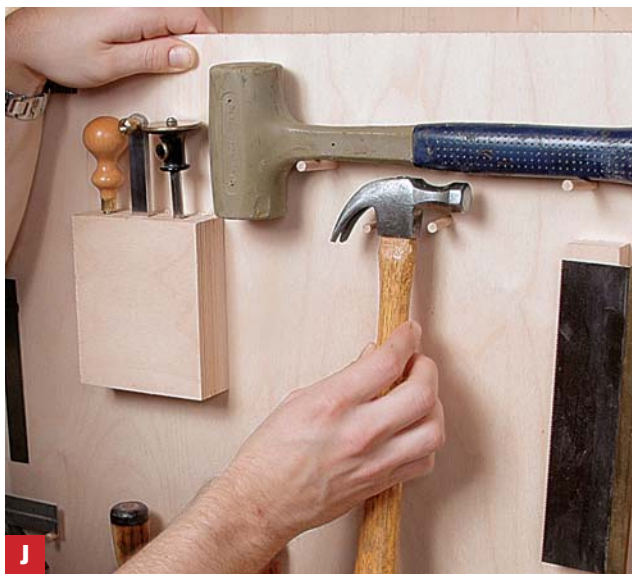
Two pegs hold a hammer in place The hammer hangs flat against the board, and it will be in easy reach when the board is hung.
