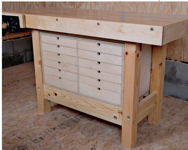
Small space, lots of storage This drawer unit provides a dozen drawers and plenty of storage for small hand tools and supplies.
