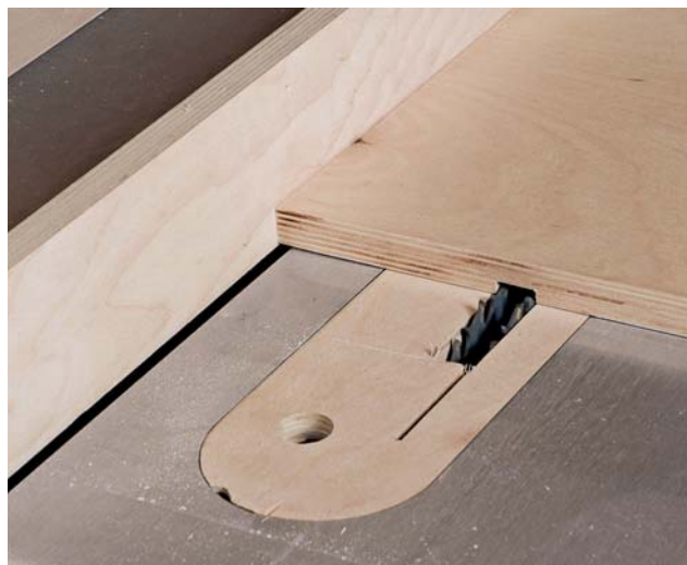
Cut dados and grooves Learn to use a dado set to cut dados, grooves, and rabbets at the table saw.
