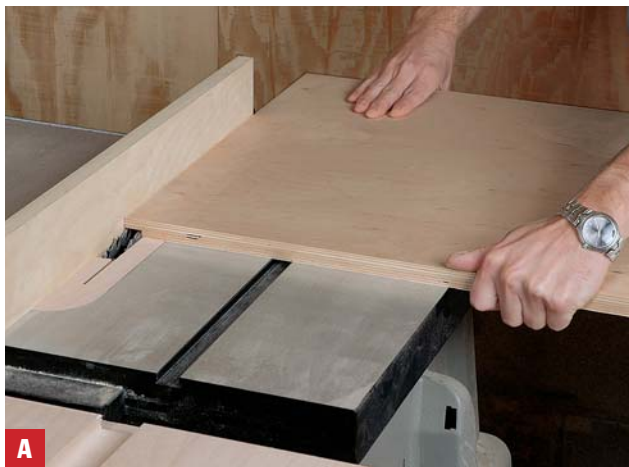
Rabbet the top and bottom To rabbet the edges of the top and bottom, install a dado head set to \frac{3}{4} " and run the auxiliary tablesaw fence almost flush to the blade.
