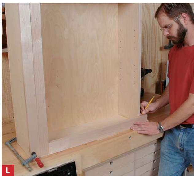
Measure the frame members With the two vertical pieces of the face frame cut to length and width, clamp them flush to one side, then hold the horizontal frame pieces in place and mark for length.
