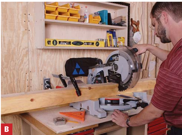
B Cut legs to length Be sure to clamp your work in place and see that the offcut is supported.
