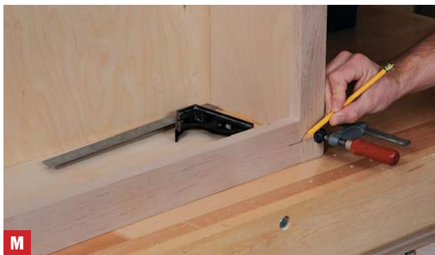
Mark for biscuits With the frame members held in place, mark out centerlines for #0 biscuits.
