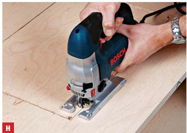
H Cut out the top To allow dust to fall through into the base, make a cutout in the top. Drill access holes at the corners, then make the cut with a jigsaw.
