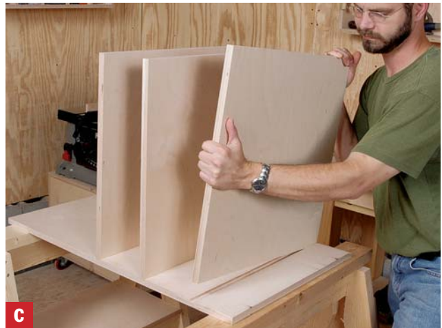
Set the shelves in place With one side of the base flat on sawhorses, fit shelves into the dados.
