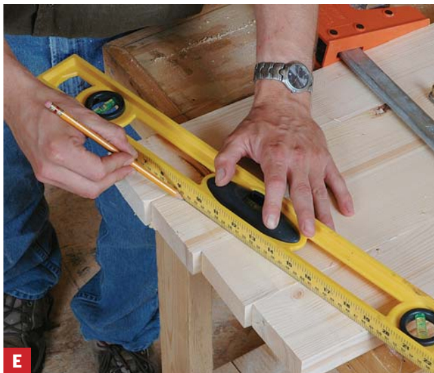
E Extend the angle Use a long ruler or straightedge to continue the angled line.
