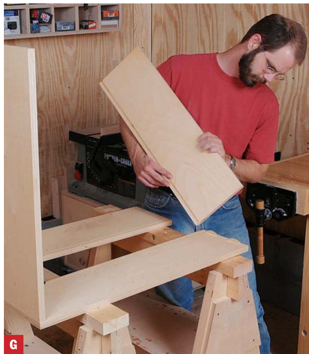
G Set the ends in place With one side of the cabinet laying across sawhorses, add glue and biscuits, then set the top and bottom in place.
