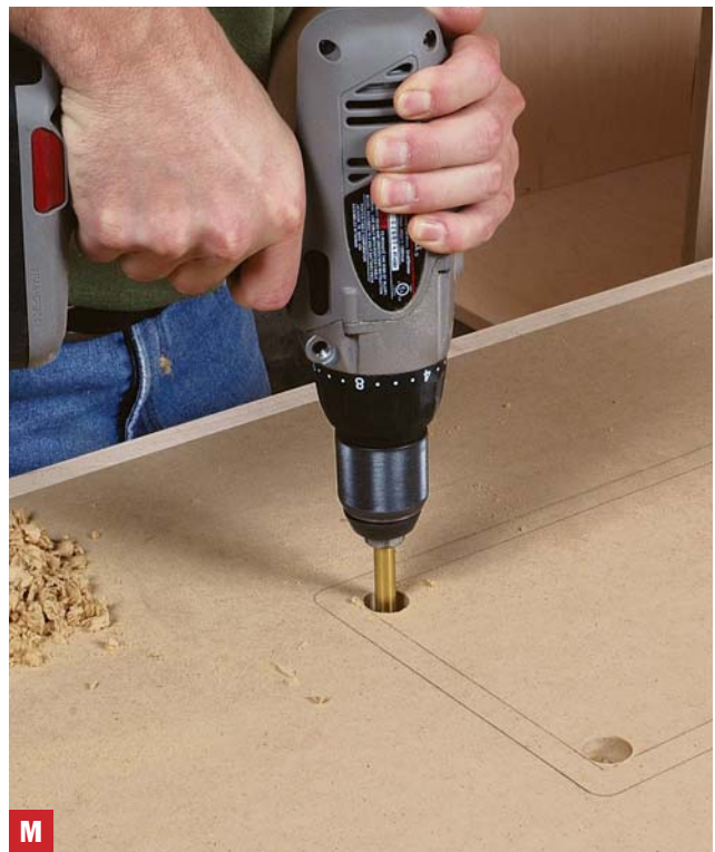
Drill access holes for the jigsaw In order to drop the blade of the jigsaw through the top, drill holes inside the corners of the inset lines.
