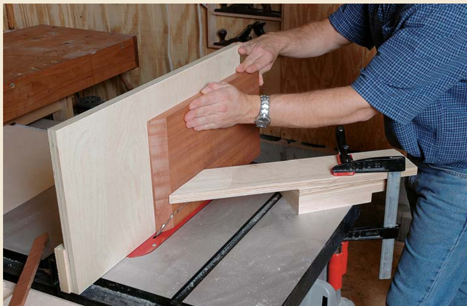
Using a high fence To cut along the edge of a wide board—for grooving or profiling an edge—use a high fence and clamp a featherboard in place above the blade.
