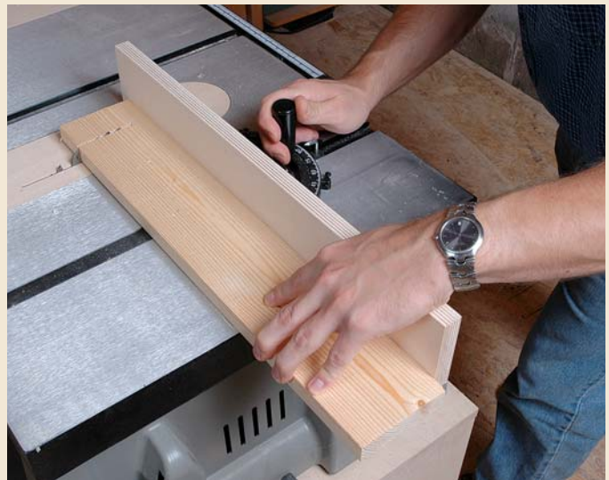
Using a miter gauge A longer miter fence provides better support as you crosscut.
