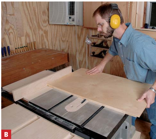
Dado for the divider Shift the fence and set it to cut a dado down the center of both the top and the bottom.
