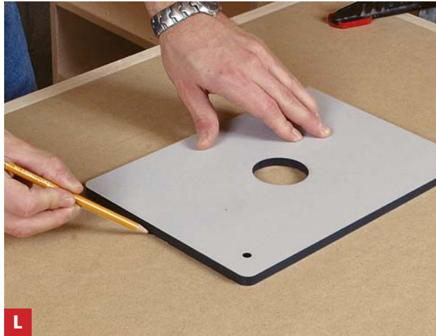
Trace around the insert plate With the router insert centered on the top, mark the outline with a pencil.
