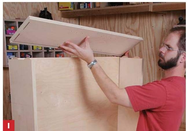
I Secure the other side Put the biscuits into place, then set the other side onto the assembly.
