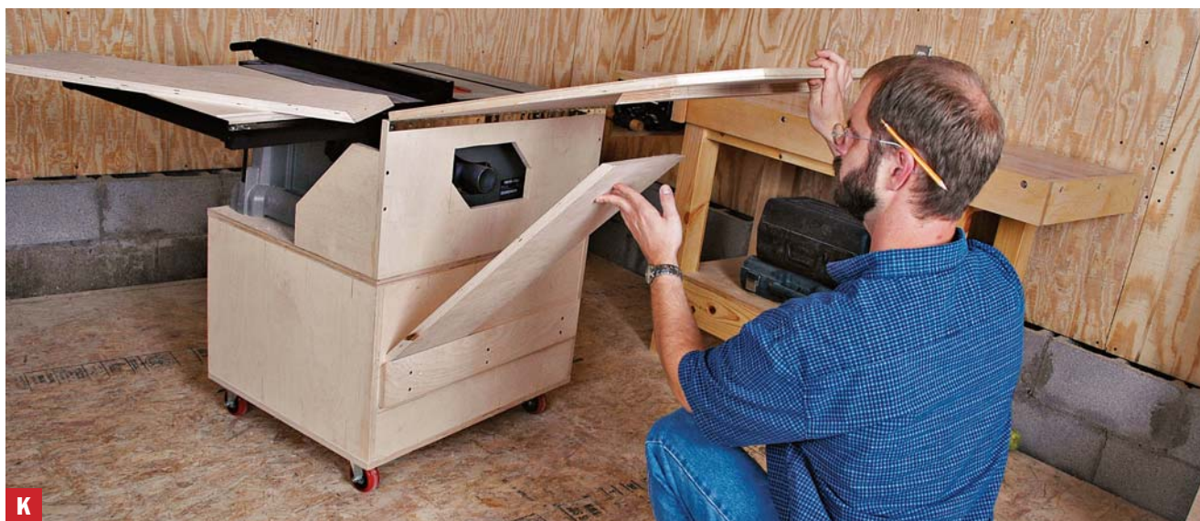
Raise the outfeed table To use the outfeed table, simply raise the table and slide the mitered braces into place. To add the first brace, lift the top and lower it onto the brace. Then add the second brace by sliding it in from the side.
