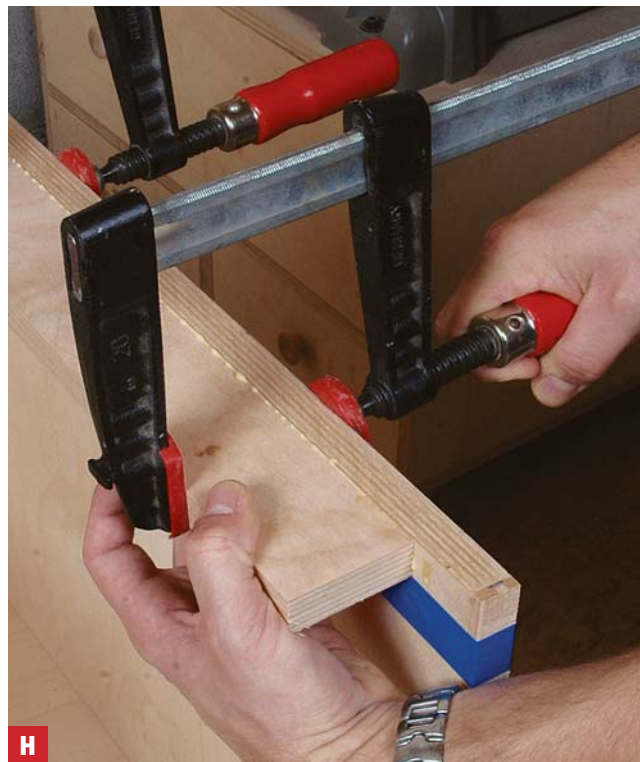
Add the glue blocks When attaching the glue blocks, make sure they are flush (or slightly below flush) to the top edge the case.
