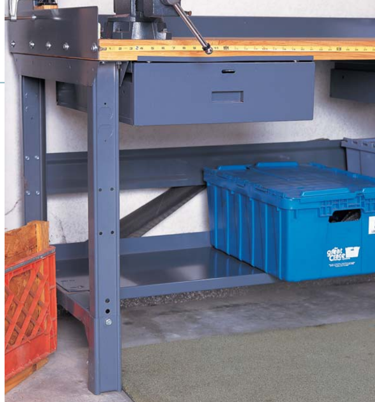
THIS BENCH , ordered from McMaster-Carr Supply Company, has legs that easily adjust in height by loosening a few bolts. John Allison uses it not only for woodworking but for many other jobs around the shop.
