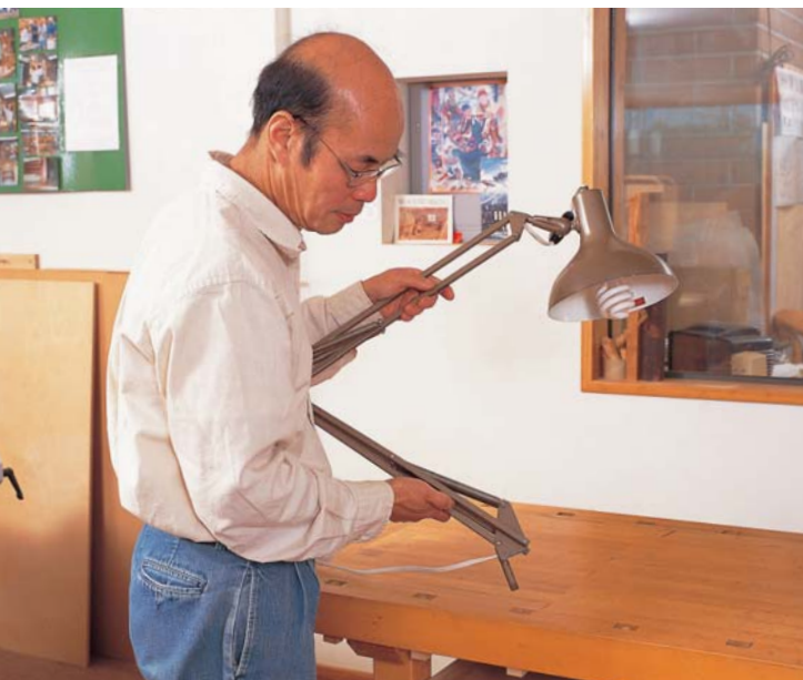
IN ONE OF HIS BRILLIANTLY SIMPLE SOLUTIONS, Yeung Chan made a solid wooden bench dog and drilled a hole in it to fit the base of his lamp. He can position the lamp anywhere he likes by inserting the special dog in any hole on his bench.
