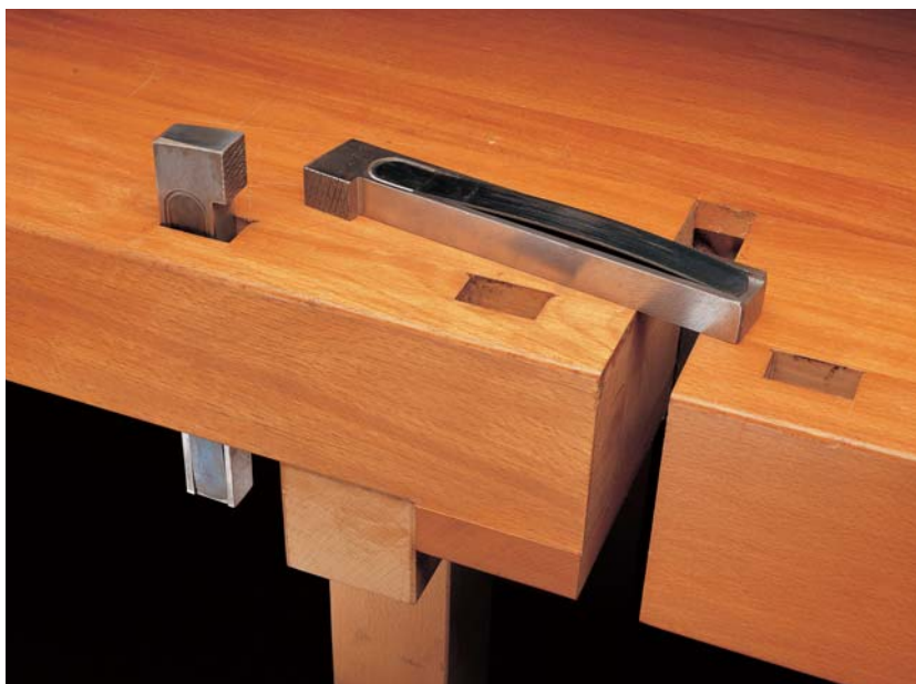
STEEL DOGS ARE STRONGER and more durable than those made of wood, but having to worry about hitting one with an edge tool is their chief drawback.
