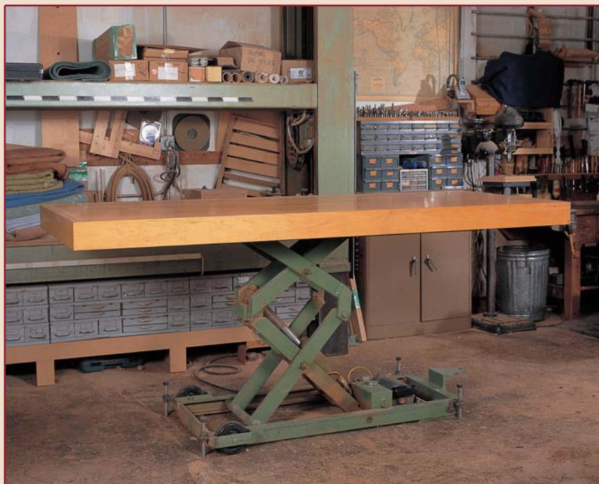
HAROLD FOSS FOUND A SOLUTION from an unexpected source. The hydraulic scissors jack that allows the height of this bench to be adjusted is more commonly seen in industrial applications, but the wooden benchtop turned it into a woodworking bench.
