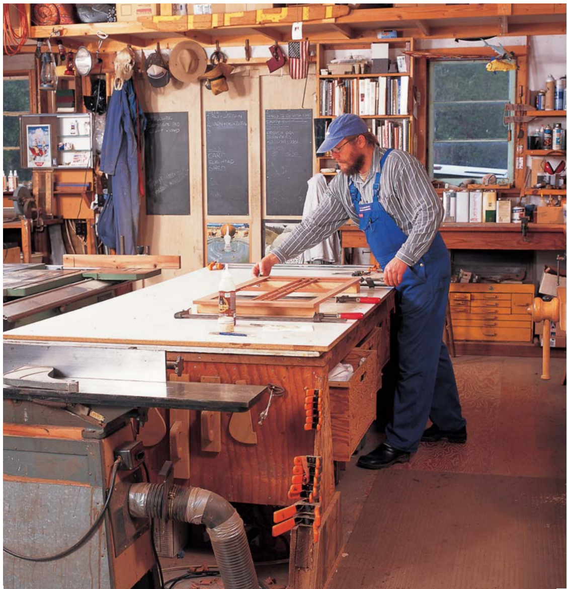
PAUL SCHURCH USES A VACUUM BAG to make many of the curved parts for his furniture. A large smooth surface is essential for proper operation of the bag.
