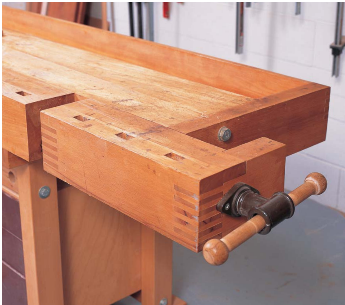
THE ENORMOUS DIEFENBACH TAIL VISE is in keeping with the proportions of the rest of the bench, one of the heaviest on the market. The narrow fingers connecting the jaws give the all-important joint plenty of gluing surface area.
