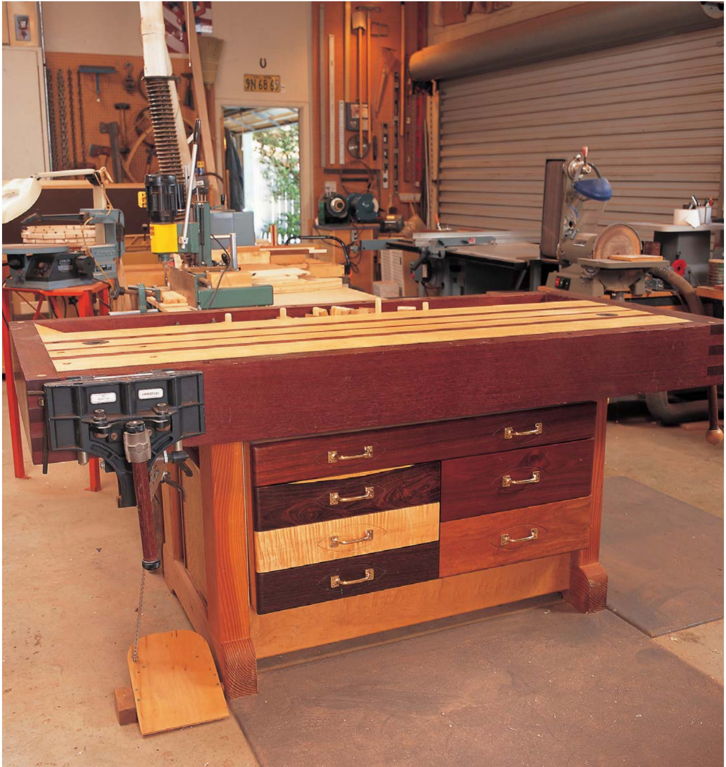
HARRY WILLIAMS CREATED A SHOWPIECE BENCH by using contrasting woods. The side rails, end caps, and some of the benchtop planks are purpleheart. He carried the theme into the drawer faces, each a different species of wood.
