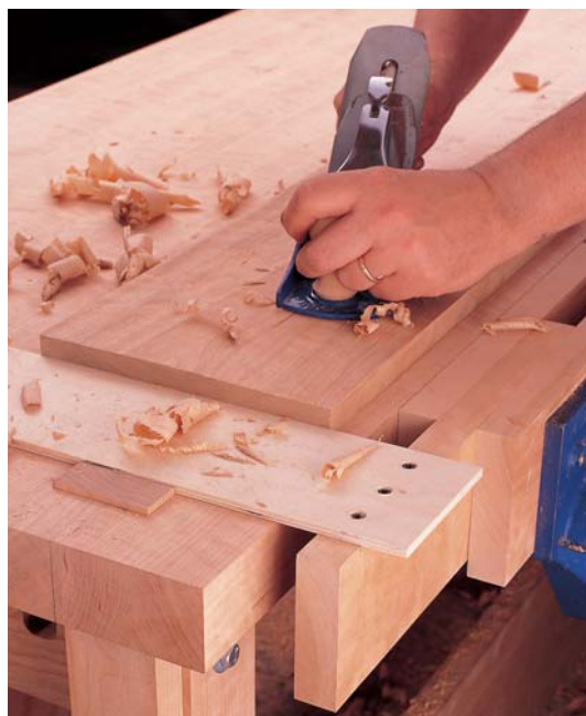
WHEN PLANING A WIDE PANEL Barrett uses his bench stop. One of the reasons he positioned his vise where he did was to facilitate using this simple device. With the stop in place, he can plane anywhere across the width of the board.
