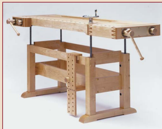
ON GARY BLAISE'S ADJUSTABLE-HEIGHT BENCH , which Curtis Erpelding custom-built for him, each leg has a threaded rod linked together with a chain hidden under the benchtop. By rotating a single crank, the entire benchtop raises and lowers.
